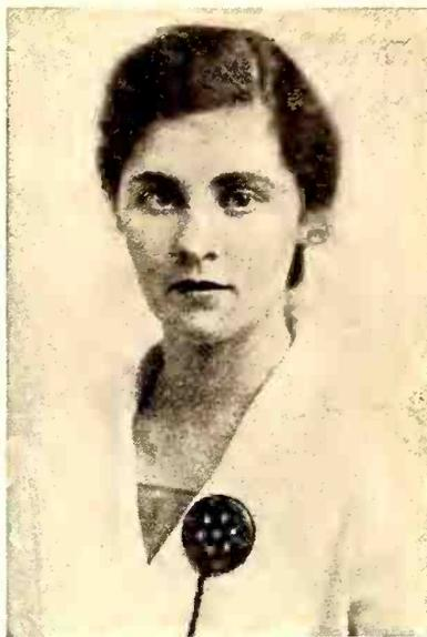
NEW LAPEL MIKE—Adrian Rousseau, school teacher, is shown wearing the new two-inch, two-button lapel microphone being introduced by Universal Microphone Co., Inglewood, Cal. The makers claim it eliminates all noises in the loud speaker when the cord is moved by using special binding screws. Satin bakelite finish makes it inconspicuous when worn.
