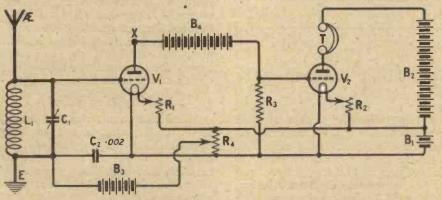
Fig. 1.-A conventional example of the trigger circuit.
