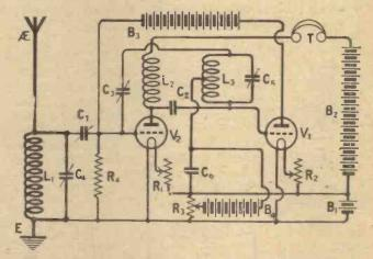
Fig. 4.—The final development was a neutralised version.
