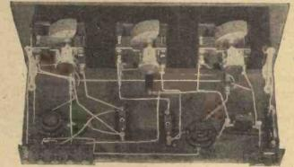
The wiring of the coil sockets should be spaced out carefully.
