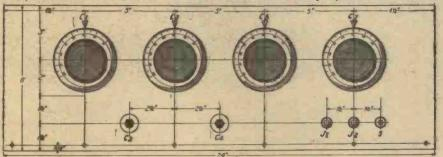
Fig. 1.—The simplicity of the panel lay-out is partly due to the omission of filament rheostats.
