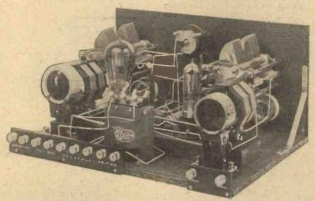
The centre-tapped coils are raised on a wooden platform in order that they may be co-axial with the standard plug-in coils.
