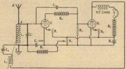
Fig. 5. Reinartz reaction can be used if the L.F. valve is employed for the purpose.
