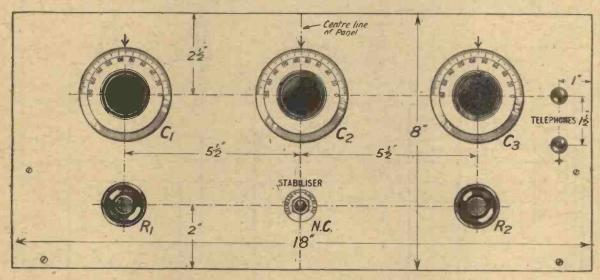
Fig. 3.—The lay-out of the panel is particularly neatly balanced.
