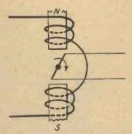
Fig. 2.—The addition of an alternating field to the alternator of Fig. 1 will produce modulations of the current generated.
