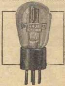
Type L.240 is a small power valve of low impedance and consequently should be used for one or two stages of low frequency amplification when distortionless loud speaker reproduction is desired. A 30 ampere - hour battery will run one of these valves for 75 hours. This valve is 3½ ins. overall in height and has a maximum bulb diameter of 13 ins.
