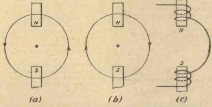
Fig. 6.—(a) represents a field magnet system revolving anti-clockwise, and (b) a similar system revolving clockwise. If the two are imagined superimposed, it can be seen that they give the same effect as the alternating field (c).
