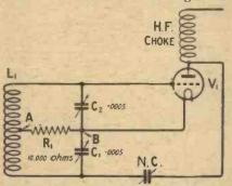
Fig. 1.—Illustrating the split-condenser method of neutralisation.
