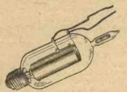
An early type of soft valve, designed by Capt. H. J. Round, in which provision was made for controlling the pressure and temperature of the residual gas present.
