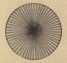
Fig. 2.—The finished diaphragm ready for mounting.
