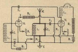
Fig. 2.—In this reflexed version "Parallel Feed" H.F. coupling is used.
