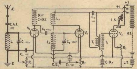
Reaction may be applied in a very simple manner to the circuit L. C., as illustrated.
