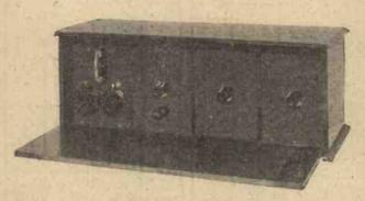
The front of the receiver lets down to expose the panels.
