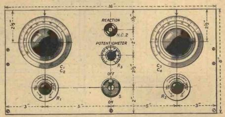
Fig. 4. - There are no terminals on the front panel, and there is comparatively little drilling required.
