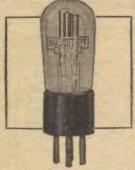
This Burndept Super Valve is of exceedingly low current consumption and is suitable as a detector and for high-frequency amplification. Using one valve, a 30 amperehour battery lasts 200-230 hours. The overall height of this valve is 34 ins., and the maximum diameter of the bulb is 13 ins.
