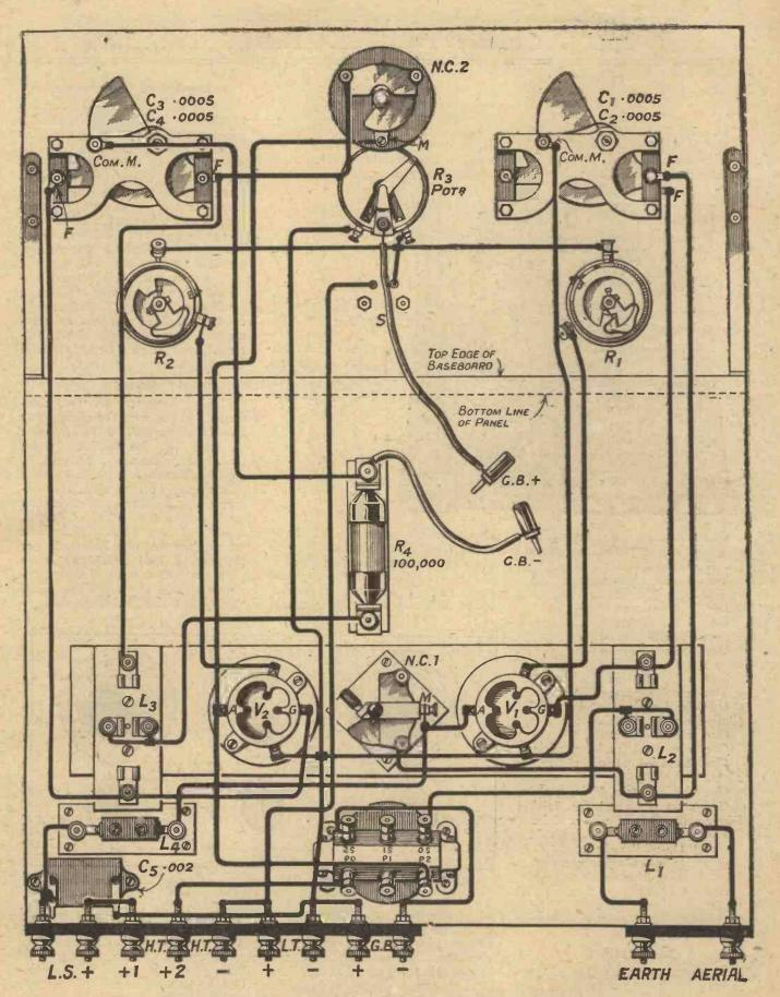
Fig. 3.—The low-tension portion of the wiring should be connected up first.
