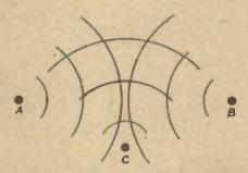
Fig 2.—The provision of a number of stations would ensure that such interference effects as might occur would not produce blind areas.
