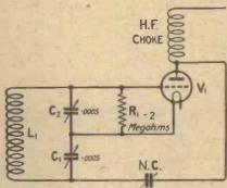
Fig. 3.—This circuit is free from parasitic oscillations, but the position of the grid-leak is not a desirable one.
