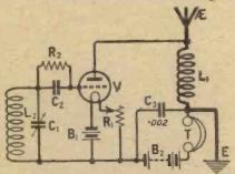
Fig. 1.—This is one of the simplest forms of anode-input circuit, with the grid and anode circuits separated in order to emphasise the salient features of the arrangement.
