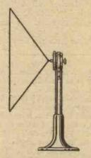
Fig. 7.- A single-cone type completed.
