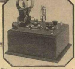
This set, designed for comparative tests of anode current and cumulative grid rectification with different valves, was described in the March issue of "Modern Wireless."
