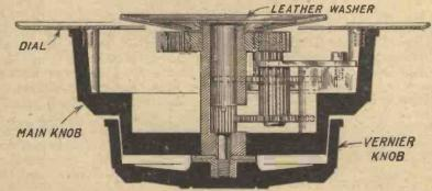
The vernier dial sent in by Messrs. The Mydar Radio Co. has a special gearing which provides an 80 to 1 ratio.
