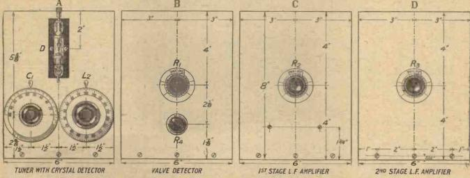
Fig. 1.—The panels are all of the same dimensions and there is very little drilling to be done.
