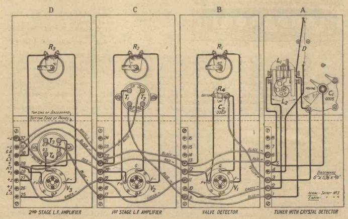
Fig. 3.—Stiff wire is used for the permanent connections and flex for the links between the units.
