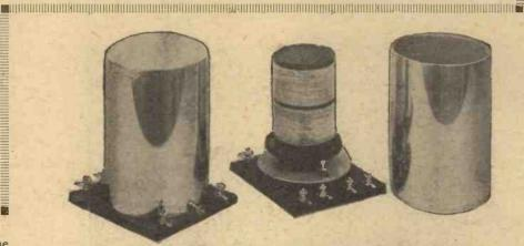
The screened coils, of the type designed by Mr. Reyner, shown here complete and with the screen removed, were found to have a low R/L ratio.
