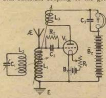
Fig. 4.—This circuit shows how that of Fig. 3 would be arranged if separate coils were used for the various functions.
