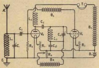
Fig. 3.—This is the circuit of Fig. 2 re-arranged in the manner usual in drawing reflex circuits.
