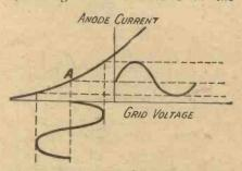
Fig. 1.—With the anode current method rectification takes place owing to asymmetrical variations in the current.
