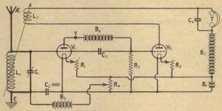
Fig. 4.—In the final arrangement good results were obtained by making the L.F. provide the desired reaction in this way.
