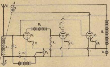
Fig. 3.—Reaction can be obtained by adding a special valve (V3) for the
