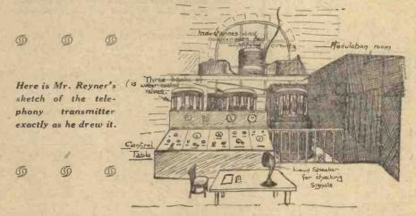
readjustments of the actual strength applied to the transmitter, but this is only a comparatively small adjustment, and the whole service is nothing more or less than a repeater station such as is employed on ordinary trunk telephone services.
