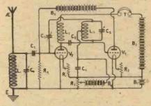
In the article "Reflexing the Prince Circuit" in last week's issue of "Wireless Weekly," Fig. 4 on page 316 was incorrectly shown, the battery B4 being wrongly connected. This diagram is correctly reproduced herewith.
