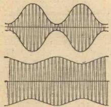
Figs. 4 and 5.— The addition of the permanent field produces wave-forms of this type, which may be compared with those produced by a telephone transmitter.
