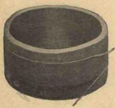
Large diameter relative to winding stength is a factor for low H.F. resistance for a given frequency.
