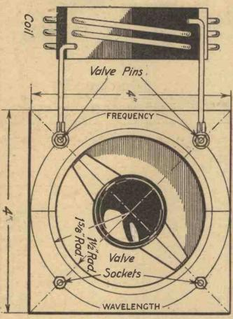
Fig. 2.- The marking of the positions of the valve pins and sockets should be done with care, to ensure that they register with those on the ebonite panel.
