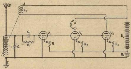
Fig. 2.—This circuit is intended to show how the three functions of a rectifying valve with reaction may be separated in an imaginary manner.
