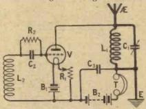
Fig. 2.—Another version of the simple type of circuit illustrated in Fig. 1. Anode and grid circuits are again shown separated, but it is to be understood that L1 and L2 are actually coupled together.
