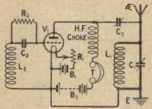
Fig. 6.—A form of reaction used in the Reinartz circuit is shown here.
