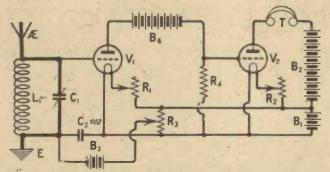
Fig. 1.—This is the conventional form of the Prince circuit, with separate valves for each function.
