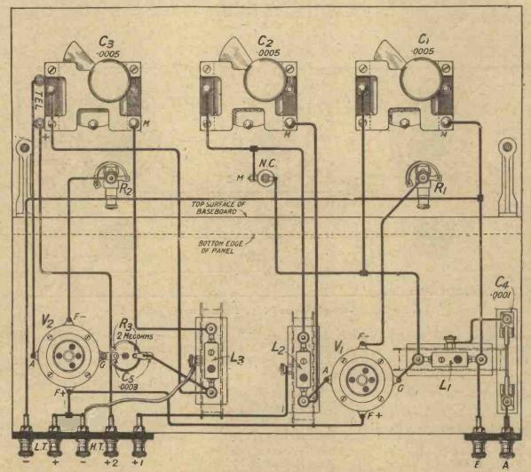
Fig. 2.—In wiring the set it is recommended that the leads to the coil L3 should be done with Azx.
