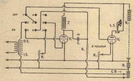
Fig. 1.— This arrangement allows of the valve V2 being in circuit whether one or two stages of L.F. amplification are used.
