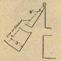
Fig. 6.—In cutting the gap allow an overlap like this.
