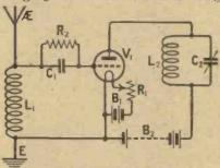
Fig. 3.—This circuit employs a form of trap tuning, by virtue of the coupling which is provided in practice between L1 and L2 (again shown separated here).
