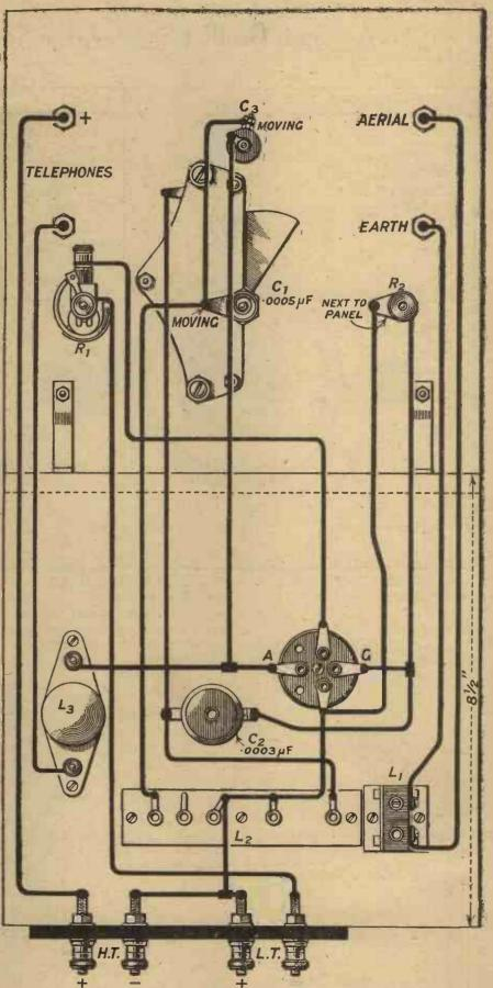
Fig. 3.—This diagram should be carefully followed by intending constructors.
