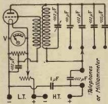
Fig. 1.—The main oscillating circuit.
