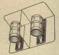
Fig. 4.—This method of partial screening gave a reduction of 60 per cent, in the amount of energy transferred.
