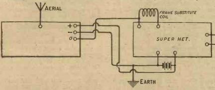
Fig. 3.—When the adapter is used with a superheterodyne the aerial and earth connections are as shown here.
