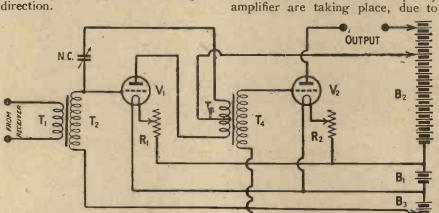
Fig. 3.—A centre-tapped or similar L.F. transformer is needed in this circuit.
