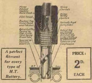
The diametrical expansion and compression of the CLIX WANDER-PLUG ensures rigid full-length, full-surface contact, with 90% of the efficiency of a soldered joint.
