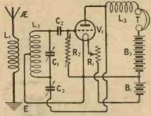
The circuit of the receiver is reproduced for reference. It will be seen that a very simple reaction scheme is used.
