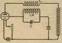
Fig. 1.—In this diagram LR represents the inductance and resistance of the coil in the grid circuit of the valve.
