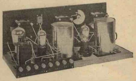
The use of screened coils permits the set to be made very compact.
