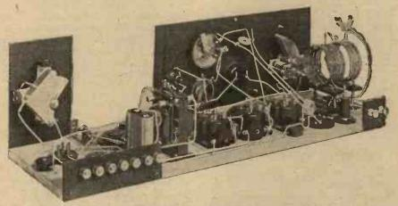
The long-wave oscillator forms a separate unit in the lay-out.
