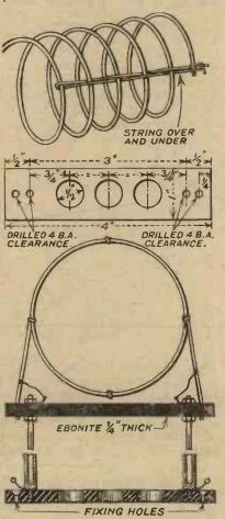
Fig. 4.—The coils are quite simple to construct.
