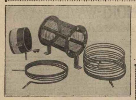
ANY people have been puzzled by the apparent difference of opinion concerning the use of skeleton formers for making up "low-loss" coils. Some people claim that the use of a former in which all possible material has been cut away, using just the bare framework on which to wind the coil, is simply a waste of time, at ordinary radio frequen-
