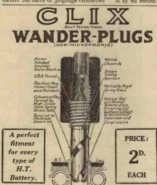
The diametrical expansion and compression of the CLIX WANDER-PLUG ensures rigid full-length, full-surface contact, with 90% of the efficiency of a soldered joint.
