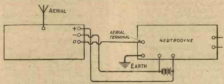
Fig. 2.—Showing how the adapter is connected to a neutrodyne set. The connections of the L.T. circuits are shown, but those of the H.T. terminals are omitted in this diagram, and also in Fig. 3.
