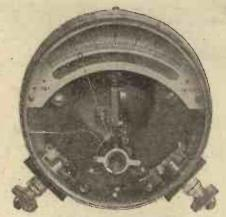
A micro-ammeter is required to indicate the change in anode current of the oscillating valve.
