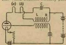
Fig. 4.—The oscillatory circuit used in the experiments from which the photographic records were obtained.
