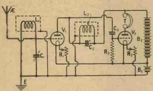
Fig. 1.— Screened coils gave a perceptible improvement in even this simple circuit.
