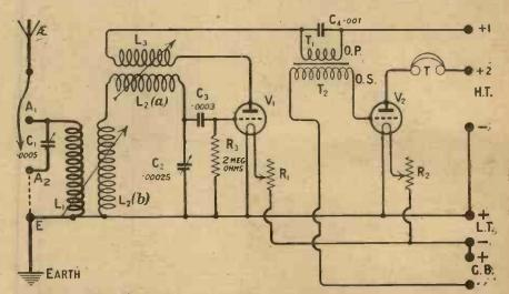
Fig. 1.—The circuit is quite a typical "split-secondary" arrangement.
