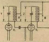
Fig. 4.—The essential portion of Fig. 3, redrawn to indicate the relationship between the portions A and B of the two anode coils.
