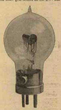
This double-grid valve, which is a product of Messrs. Radio: Valves, Ltd., employs a terminal on the metal cap for connection to the inner grid.
