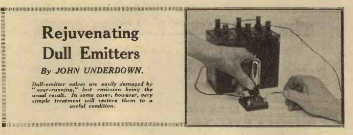
ANY experimenters who have graduated in the brightemitter school do not fully realise that although the filament of a dull-emitter valve may be continuous and appear to light correctly, the valve may nevertheless have lost its emission and be practically useless whilst in that condition.
