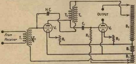
Fig. 2.—This circuit is the low-frequency counterpart of the Cowper neutrodyne.
