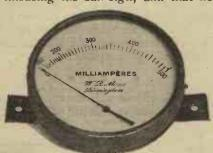
A low-reading hot-wire meter of this type is useful for indicating the small aerial currents obtained at the higher frequencies.
