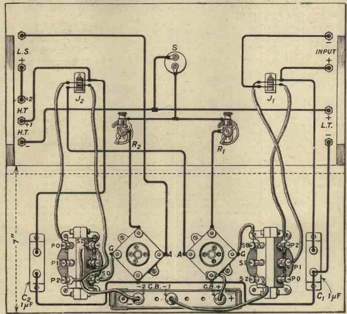
Fig. 3.—Note the placing of the two valve-sockets. A considerable simplification of wiring resulted from this arrangement. It should also be observed that certain of the connections are made with flexible leads.
