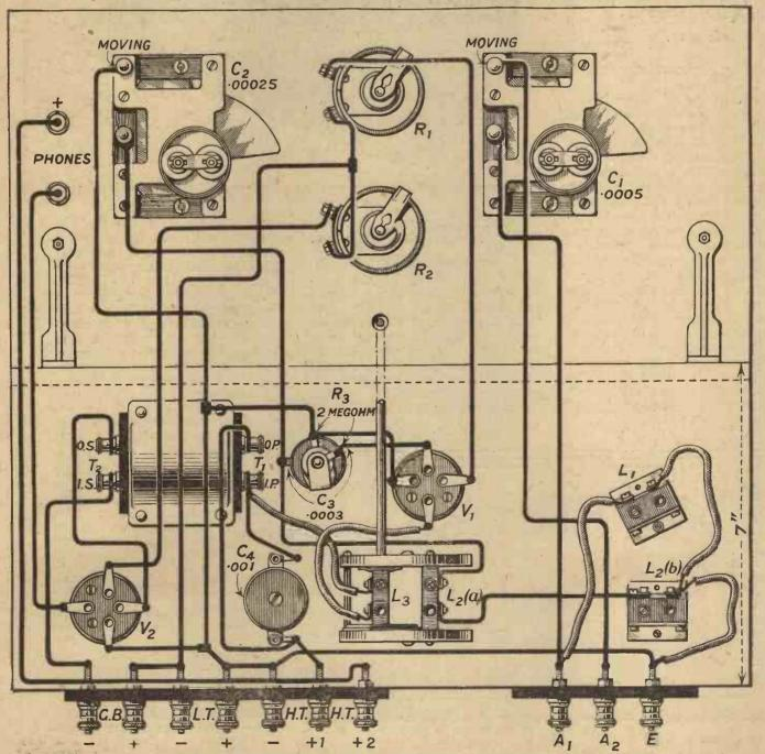
Fig. 3.—In carrying out the wiring it is advisable to use flex for the connections to the moving coil sockets.
