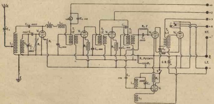
Fig. 1.—The condenser in the aerial circuit is of the small neutrodyne type, while C<sub>8</sub> is supplied with the intermediate transformers.
