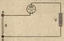
Fig. 1 (B).—Here the valve and external resistance are shown in their correct relationship. Compare with Fig. 1 (A).
