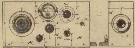
Fig. 2.—Two separate ebonite panels are used, but they could be combined in one of suitable size if desired.
