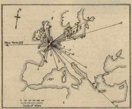
The lines on this map join the author's station to various points at which he has been heard. The numbers indicate the relative strength of signals at each point, the poorness of results to the south being clearly shown.
