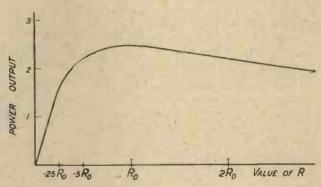
resistance of the valve from plate to filament, and R is a variable resistance which can be varied from zero to infinity. Fig. 1B. shows the same circuit with the plate-filament resistance replacing Ro.
