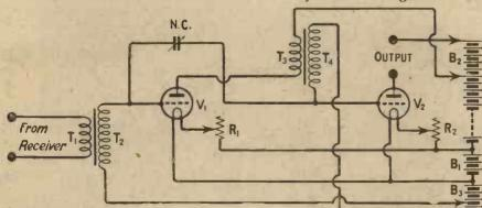
Fig 1.- A simple scheme resembling the Hazeltine neutrodyne arrangement.
