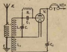
Fig. 2.—In the earlier versions the telephones were used as an H.F. choke.
