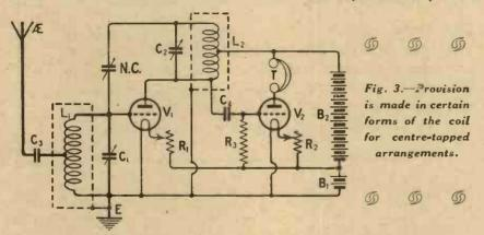
pletely removable, after which the coil itself may be removed from its socket, and either replaced by another coil or rewound or altered in any way required. In this particular instance, Messrs. Peto-Scott have provided a six-pin base which provides for practically all the ordinary types of circuit.
