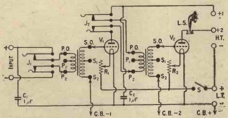
Fig. 1.—Plugs and jacks are provided to permit telephones to be used with one note-magnifying value and to enable them to be connected directly to the input.
