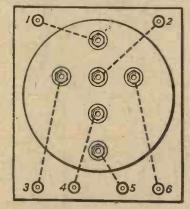
Fig. 4.—The standard connections of the coil base.
