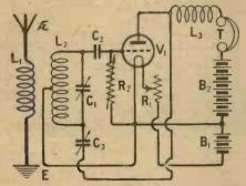
Fig. 1.—Reaction effects are obtained by adjustment of C3, without affecting seriously the setting of C1.
