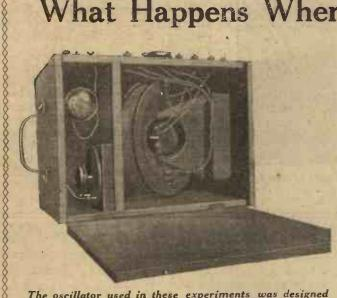
The oscillator used in these experiments was designed for low frequencies. The valve may be seen in the compartment on the left.
