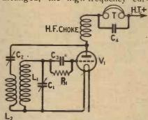
Fig. 3.—Better results are obtained by including a choke in series with the 'phones.
