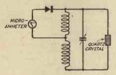
Fig. 2.—The frequency of the subsidiary oscillator is checked by means of a crystal control circuit.
