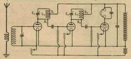
Fig. 3.—Taking the tappings S1 and S2 from slightly different points upon the coils L3 and L4 will overcome the tendency to parasitic oscillations, with little effect on oscillation at the main frequency.
