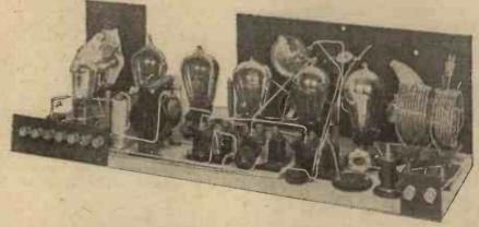
This view shows how the aerial lead from the series condenser is attached to the appropriate tapping point on L2.
