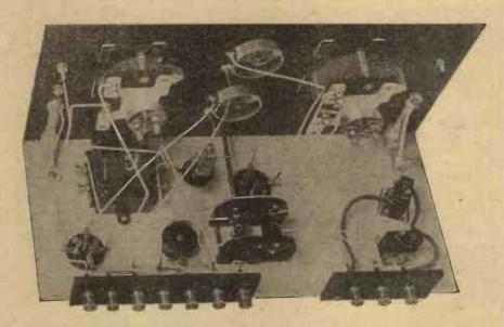
The coil-holder is of the long-handle variety, the knob appearing on the front of the panel.
