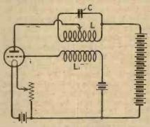
Fig. 2.—The use of an anode tap makes possible an adjustment for the maximum oscillatory current without alteration of the coupling.
