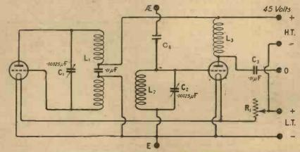
Fig. 1.—The complete circuit of the two-valve adapter. L1 and L2 are coupled together.
