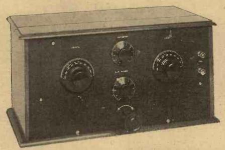
There are only two tuning controls, and the reaction is adjusted by means of a slow-motion coil-holder. All the battery terminals are at the back of the receiver.
