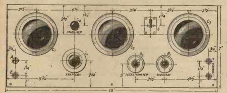
Fig. 2.—The panel lay-out gives a very convenient arrangement of controls.
