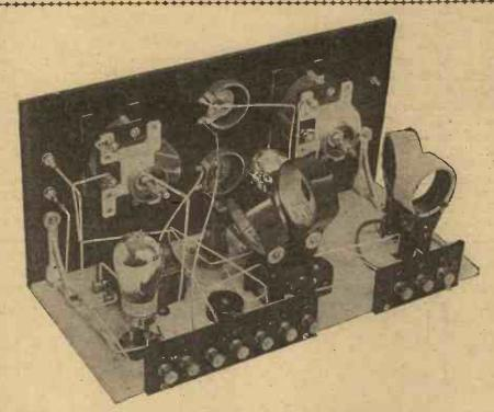
The aerial and secondary coupling coils are adjusted in position by swivelling their mounts.
