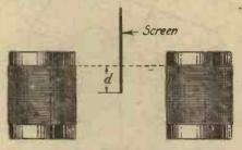
Fig. 2.—The effect of introducing a single shield between the coils to a distance "d" was investigated, and the result is expressed in Fig. 3.
