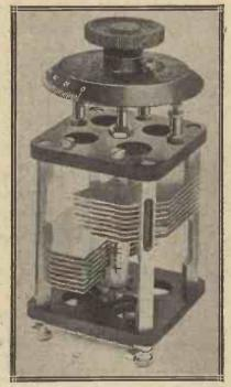
Dielectric material is sometimes "economised" in the electrical sense by drilling large holes in the end plates.
