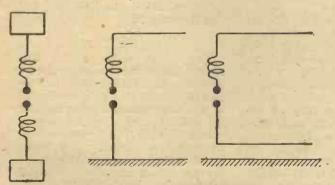
Fig. 1.—The early transmitters made use of arrangements closely similar to that of the modern aerial and earth screen. (Right and left above.)
