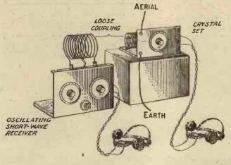
If the short-wave set is placed beside a crystal receiver strong harmonics of the local station can be picked up with ease.
