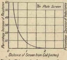
Fig. 2.—Using a tin-plate screen the effective resistance of the coil increases rapidly as the screen is brought near to the coil.
