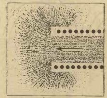
Fig. 4.—Iron filings arrange themselves in this way in the field of a solenoid coil.
