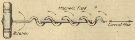
Fig. 2.—A useful rule for the direction of a magnetic field can be memorised with the aid of this diagram.
