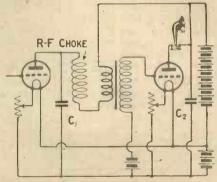
Fig. 3.—Mr. Harris recommends the use of the radio frequency choke illustrated in some circumstances.
