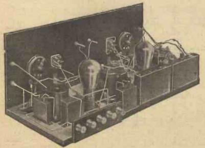
It is preferable to use separate grid-bias batteries for each stage, while the spacing out of the wiring and components requires considerable attention when a good deal of power is to be handled.
