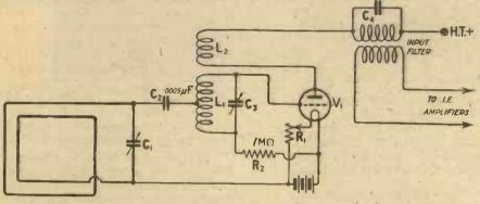
Fig. 1.—The conventional form of the Tropadyne oscillator circuit, which presents several practical difficulties.
