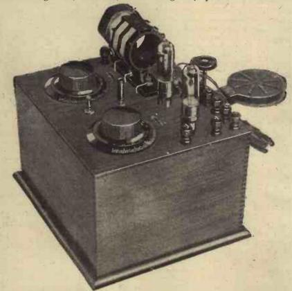
The "Huntsman Two" receiver, described by Mr. Harris in the March issue of "The Wireless Constructor," employs a split grid coil circuit.
