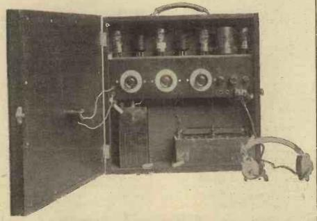
An ingenious portable set designed by Mr. Guy C. Beddington, whose name is familiar to "Wireless Weekly" readers in connection with the Prince trigger circuit. The frame aerial is wound inside the door of the cabinet. The door can be slipped off its hinges and replaced with another containing the frame for 5XX.
