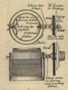
Constructional details of the bearing.
