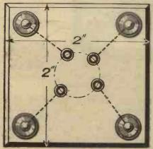
Fig. 2.—The drilling diagram for the valve-holder.
