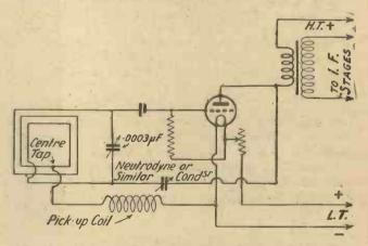
Fig. 6.—The use of reaction from the first detector may be arranged in this way, and may prove very effective.
