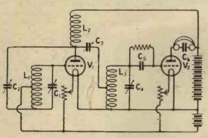
Fig. 5.—This circuit, although og being stabilised; only applies half of the available voltage to the grid of V1.
