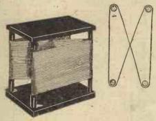
An astatic coil of simple construction due to Mr. Harris.
