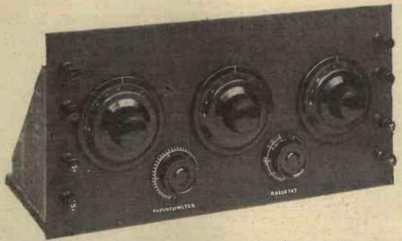
The special terminals employed are already engraved. The controls can be marked in the ordinary way with panel transfers.
