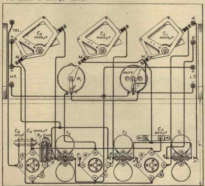
Fig. 3.—The practical wiring diagram. Note that for clearness the lower soldering tags of the transformers ("B" and "P") are drawn as if projecting more than is actually the case. Either the terminals or soldering tags of the valve sockets can be used.
