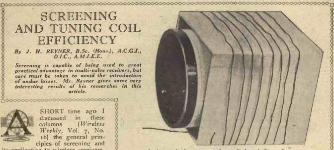
An improvised screen can be made by winding a few turns of wire round a cardboard box.
