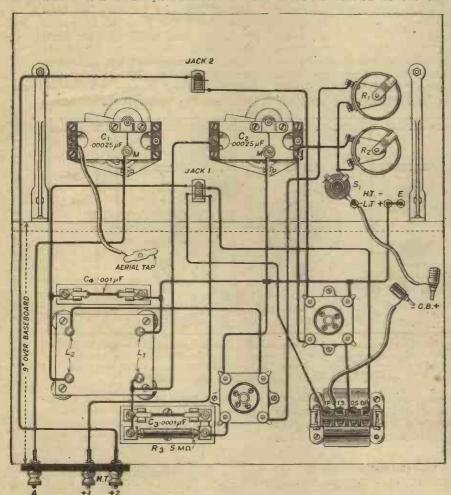
Fig. 3.—The "platform" for the coils should be kept as free from the other components as possible, all wires being taken well to the sides of it.
