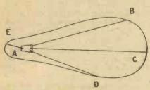
Fig. 10. - Illustrating the distribution of a single frequency from a horned loud-speaker situated at A.
