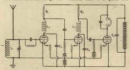
Fig. 7.—How a resistance amplifier may be compelled to function in a correct manner by means of chokes and by-pass condensers.
