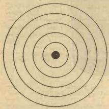
Fig. 1.—The field around a straight wire takes the form of a series of concentric circles, along which iron filings would set themselves.
