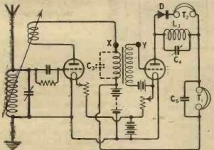
Fig. 4.—Signals in the telephones T2 demonstrated the presence of an H.F. component in the anode current of the second valve.
