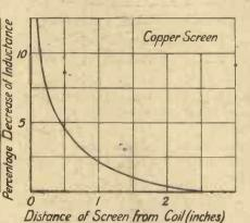
Figs. 4 and 5—When a copper screen is employed the increase in resistance is considerably reduced, but the change in inductance is only slightly affected.
