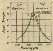
Fig. 6.—The last test was to insert the added resistance in the aerial circuit.
