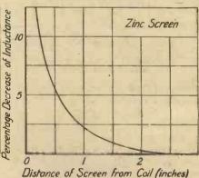
Figs. 6 and 7—The use of zinc for the screen gives results similar to those for copper. If the screen is not nearer than two inches the effect is practically negligible.
