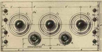
Fig. 2.—Drilling the panel is a very simple operation, the necessary dimensions being given here.
