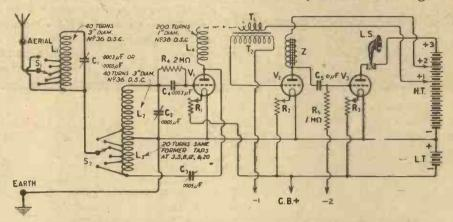
A simplified version of the circuit employed, showing how the switching of the coupling turns of the wave-trap and tuning coils is effected. Note the position in the circuit of the reaction condenser.
