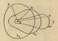
Fig. 11.—The outlines X, Y and Z represent the relative distributions of three different frequencies from the loudspeaker at A.
