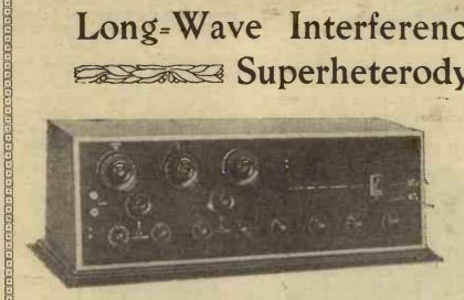
An eight-value superheterodyne designed by Mr. Scott-Taggart, incorporating a stage of tuned H.F. in front of the first detector.
