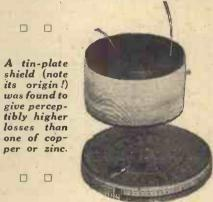
merely preliminary, and refer principally to static screens. They are interesting in that they show how near a metal object may be brought to a coil without having any serious effect on the efficiency of the circuit.
