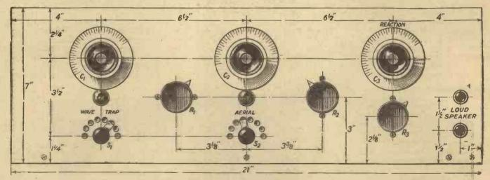
In making an exact copy of the original set this drilling diagram should be used. The only terminals on the front of the set are for the loud-speaker, those for aerial and earth and batteries being placed on strips attached to the rear edge of the base-board.
