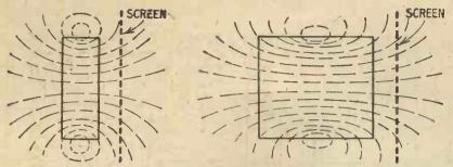
Fig. 10.—With a long coil the external field is a smaller proportion of the total field, so that the effect of the screen is not so marked.
