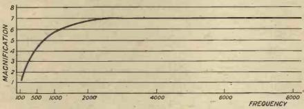
Fig. 4.—Showing the effect of using a choke coupling of unsuitable impedance.
