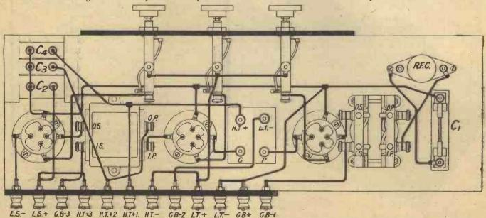
Fig. 2.—The lay-out of the set is given in detail in this wiring diagram. The O.P. terminal of the first transformer and one of the terminals of the condenser C<sub>1</sub> serve as input terminals.
