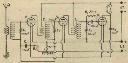
Fig. 1.—The abserce of special neutrodyning arrangements renders the circuit notably simple.
