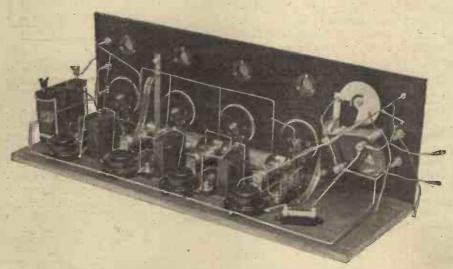
The design of a set with three resistance stages calls for some care in lay-out.
