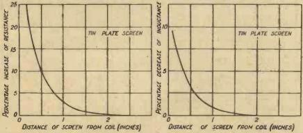
Figs. 8 and 9.—The screening effect depends on the shape of the coil, and is smaller with a long coil than with a short one. Compare these curves with those in Figs. 2 and 3.
