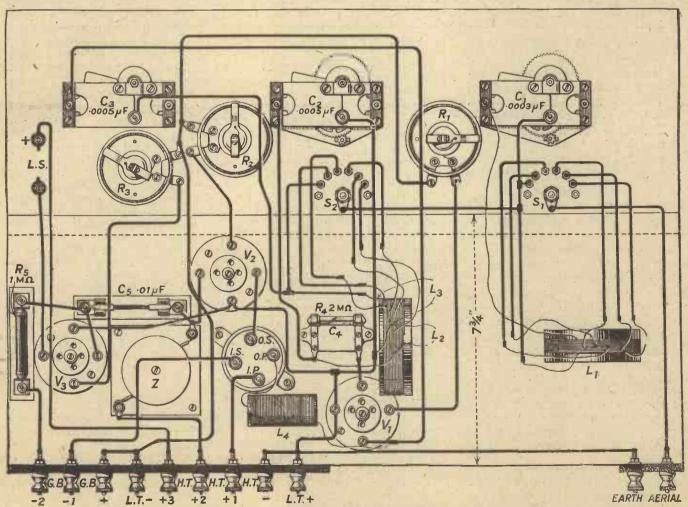
A complete wiring diagram is provided, and it is advised that this be followed with reasonable exactitude, since it is important to avoid inter-action effects between the wave-trap circuits and those of the receiver proper.
