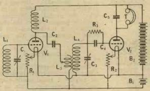
Fig. 3. -In this circuit a shunt coupling scheme is employed.
