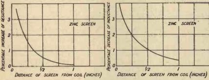
Figs. 12 and 13.—The variation of resistance and inductance is much smaller when the screen is placed at the side of the coil.
