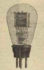
The latest type of D.E.4 valve has a pipless bulb.
