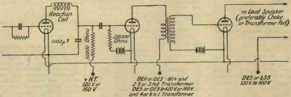
Fig. 1 .- This circuit arrangement is recommended by Captain Round, and he gives here the necessary practical details for operating it successfully.
