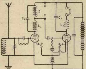
Fig. 5. - A high-frequency choke (L2) may be included to eliminate the passing-on of H.F. potentials.
