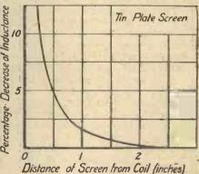
Fig. 3-Due to the presence of the screen the effective inductance of the coil is also altered, the variation being as shown above.
