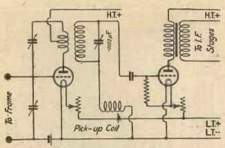
Fig. 3.—The first neutrodyne circuit tried proved somewhat unsuitable for the set under test.
