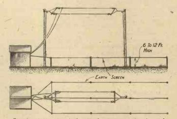
Fig. 2.—A comparatively simple arrangement of aerial and earth screen which can be made to serve experimental purposes very successfully.
