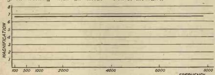
Fig. 3.-The "curve" given by a perfect resistance amplifier.
