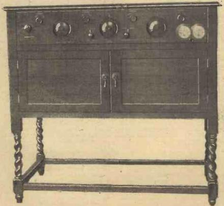
The modified "Family Four" receiver, built by Mr. Amos, incorporates measuring instruments in the battery circuits.
