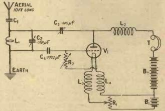
Fig. 2.—This circuit oscillated over the whole scale of C2 with either a one-turn or a half-turn coil as L1.
