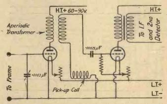
Fig. 2.—An aperiodic transformer was tried, and found to give considerable amplification, without the addition of another tuning control.
