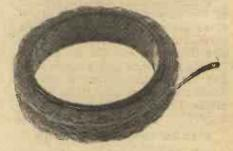
Coil "B" was a small honeycomb wound on an ebonite ring.
