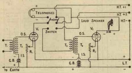
With the switch in the "one valve" position, the filament circuit of the second valve must be broken by means of the rheostat R2.
