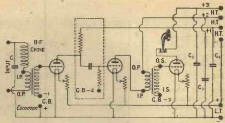
Fig. 1.—The circuit incorporates two stages of transformer coupling and one of resistance-capacity.
