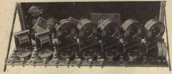
A special lay-out of the intermediate frequency coupling units is adopted in this superheterodyne (Igranic) to minimise interaction effects.
