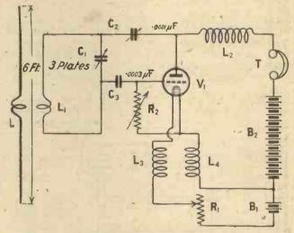
Fig. 3.— The use of an aerial circuit of this type permitted oscillation on still higher frequencies.
