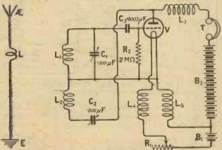
Fig. 1.—With this circuit it was found advisable to place the coil L at least a foot from the secondary, L1.
