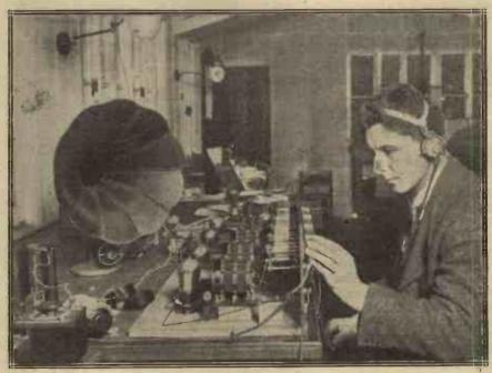
One of the sensitive receivers used at our Elstree laboratories for finding the distant stations on the occasion of the B.B.C.'s fifteen minutes' silence.
