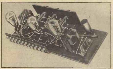
The amplifier is built on experimental lines, with facilities for easy testing of different values of components etc.
