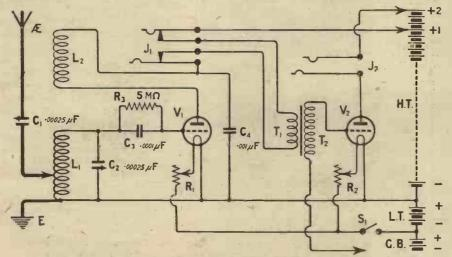
Fig. 1.—A simplified circuit diagram of the receiver. The switch S1 is provided so that the adjustments of the rheostats need not be upset.
