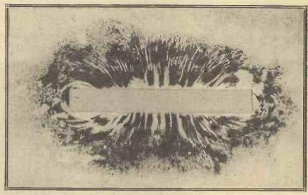
A photograph of a coil field as indicated by the iron filings method.
