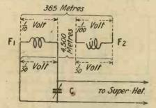
Fig. 1.—Illustrating the relative magnitudes of the e.m.f.'s induced in a tuned and an untuned frame by a signal of resonant frequency and one of widely different frequency.
