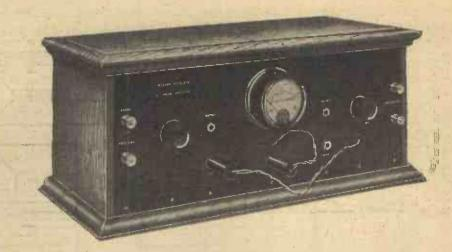
It is wise in building a power amplifier to include a milliammeter on the panel in order that the correct adjustment of grid bias, etc., may be made most easily by observation of anode current.
