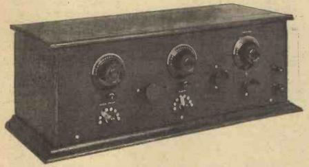
The wave-trap and main tuning condensers are of the geared variety, the author finding a plain pattern adequate for reaction control.
