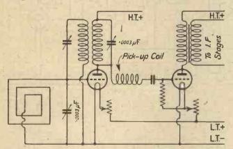
Fig. 7.—The "Cowper" neutrodyne method was tried and found very stable, but the degree of selectivity was not high.
