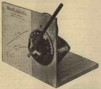
Extension handles are helpful on the higher frequencies, since it is difficult to eliminate hand-capacity effects by any other simple method.
