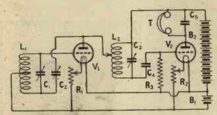
Fig. 8.—High selectivity is obtainable with this circuit.
