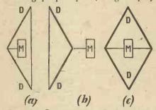
Fig. 13.—Certain types of conical diaphragms are prone to give distortion as a result of phase differences in the sounds arriving at a distant point from opposite sides of the diaphragm.
