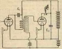
Fig. 1.—The by-pass and reservoir condensers C1 and C2 are here shown in their conventional positions.
