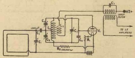
Fig. 2.—The difficulty of finding the exact centre of L1 may be overcome by the use of the two small condensers C4 and C5.
