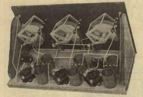
This view with the valves removed shows clearly how the parts are laid out on the base-board.
