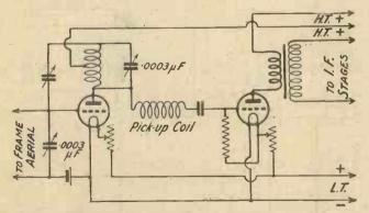
Fig. 4.—A circuit which gave very good signals, but hand capacity effects were troublesome.
