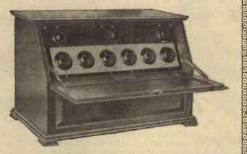
The "Straight-Eight" receiver, which was designed by Captain Round, incorporates six tuned circuits, and gives a high degree of selectivity.
