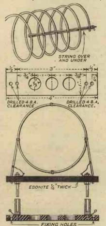
Constructional details of the coils and coil socket.
