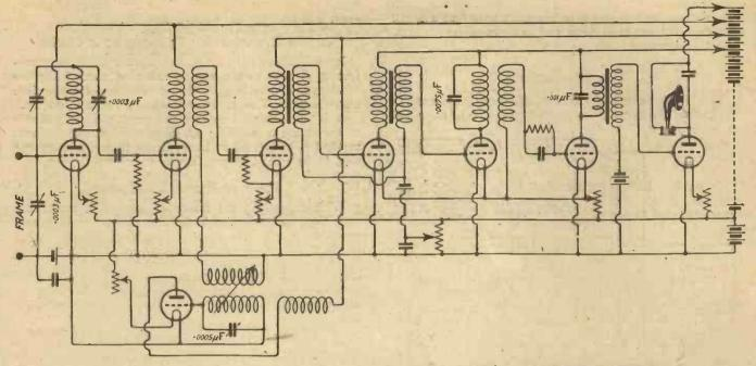
Fig. 5.—The most successful arrangement tried. Two stages of H.F. precede the first detector.
