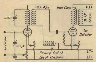
Fig. 1.—The first circuit tried by the author. When used on a frame aerial this proved exceedingly unstable.
