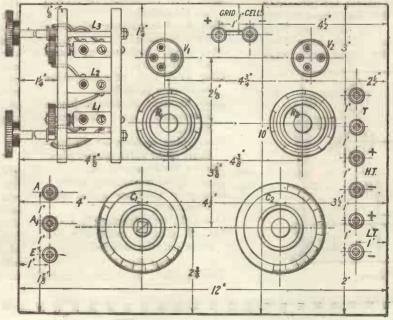
Fig. 4.—The panel layout. Blueprint No. 83a.
