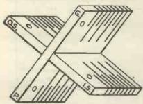
Fig. 2.—The former assembled and the arms marked.
