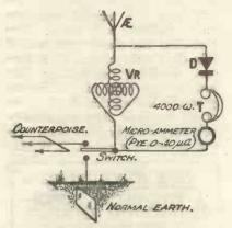
Fig. 3.—The circuit used for measuring the effect of counterpoise.
