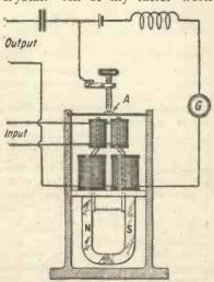
Fig. 1.—The patent drawing of S. G. Brown's microphone amplifier. The instrument Dr. Pickard found to be a sensitive detector of oscillations.
