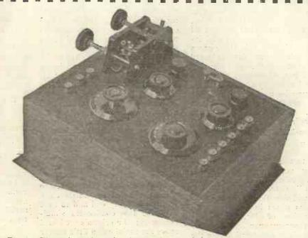
Fig. 3.—The disposition of the components upon the panel may be observed from this photograph of the set without its coils and valves.
