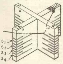
Fig. 3.—Commencing the secondary winding.
