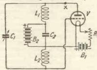
Fig. 30.—A single circuit oscillator using two separate inductances in series.
