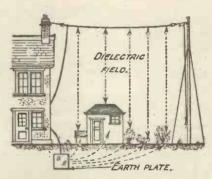
Fig. 1.— Illustrating the current paths in earth, and partly conducting objects.
