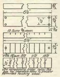
Figs. 1, 2, 3, illustrating the wood strips, the ebonite bridges and position of terminals.
