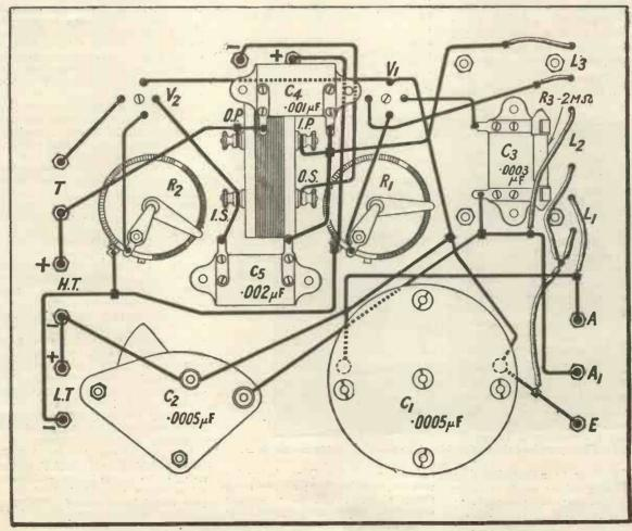
Fig. 5.—Practical back-of-panel wiring diagram. Blue print No. 83b.
