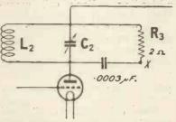
Fig. 2.—Showing that R3 is virtually in parallel with L2 C2.
