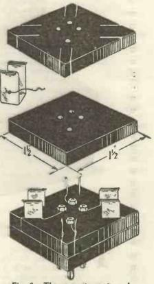
Fig. 6.—The separate parts and assembled adaptor.
