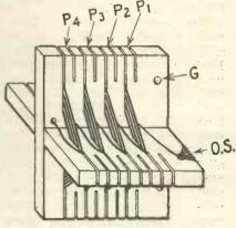
Fig. 4.—The secondary winding completed.
