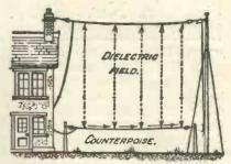
Fig. 2.—The effect of insulated counterpoise.
