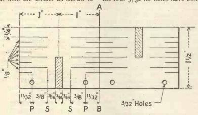
Fig. 1.—The lay-out and drilling dimensions of the ebonite sheet.
