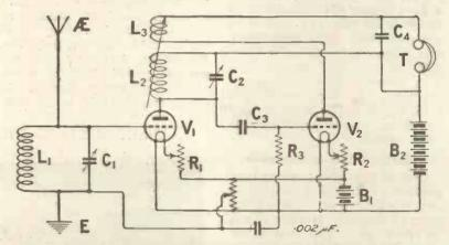
Fig. 1.—A well-known arrangement to illustrate the position of C3 and R3 in relation to one another.
