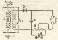
Fig. 5.—A copy of the circuit contained in a patent issued to Dr. Pickard on oscillating crystal circuits.
