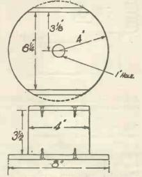
Fig. 4.—Constructional details of the disc and side pieces.
