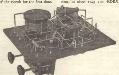
Fig. 7.—The well-spaced wiring of the receiver may be seen from this photograph.
