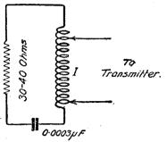
A NON-RADIATING ANTENNA EMBODYING INDUCTANCE, RESISTANCE, AND CAPACITY COMMONLY KNOWN AS AN "ARTIFICIAL" OR DUNMY AERIAL.
