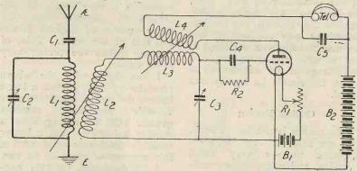
Fig. 1.—A loose-coupled circuit employing a "split secondary" for easier operation and adjustment.
