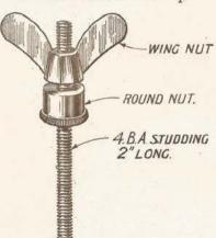
Fig. 4.—How terminals can be improvised.
