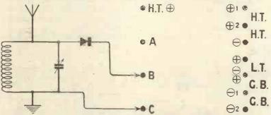
Fig. 7.—Connections for crystal receiver.
