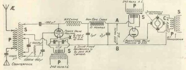
Circuit diagram of the transmitting circuit used by Mr. Goyder.
