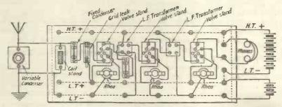
Fig. 17, A detector and two note magnifiers wired up on the layout board,
