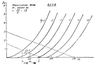
Fig. 9.—Curves for the D E.5B valve.
