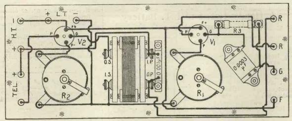
Fig. 8.—Practical back of panel wiring diagram.
