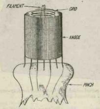
Fig. 2.—The electrodes of a power valve.
