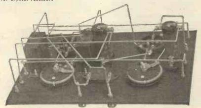
Fig. 8.—Perspective view of back-of-panel wiring.
