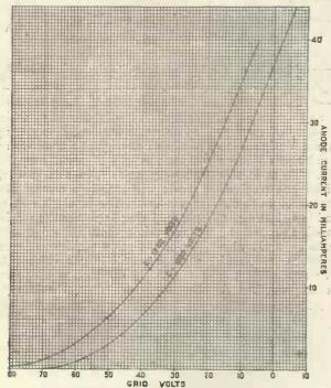
The T.50 will dissipate 50 watts on the anode.
