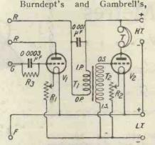
Fig. 5.—Circuit of the detector and note magnifier panel.
