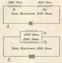
Fig. 5.—Illustrates the effect of resistances in series or parallel.
