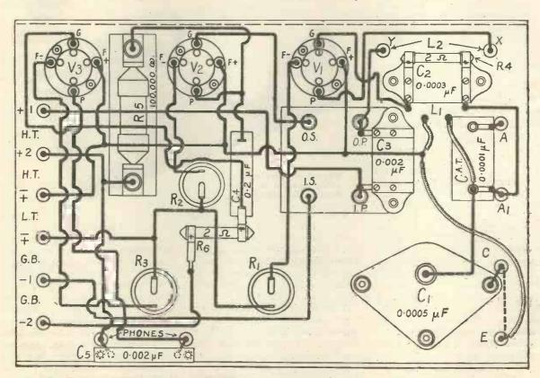
Owing to an error in the photogravure process the wiring diagram which appeared on page 25 of our photogravure supplement was shown incorrectly, the grid and anode of the second valve being joined together. The corrected diagram appears above.
