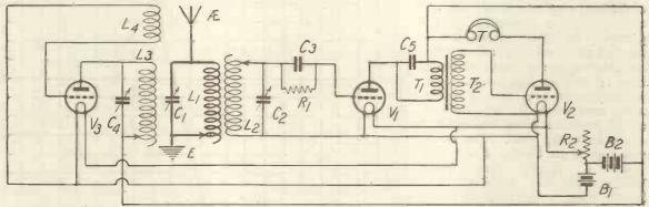
Fig. 8 .- One set of batteries only may be used for oscillator and receiver valves.
