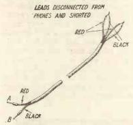
Fig. 1.—The leads arranged for a continuity test.
