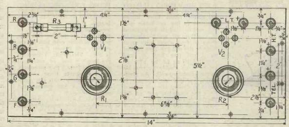
Fig. 7.—The layout of the panel and drilling dimensions.
