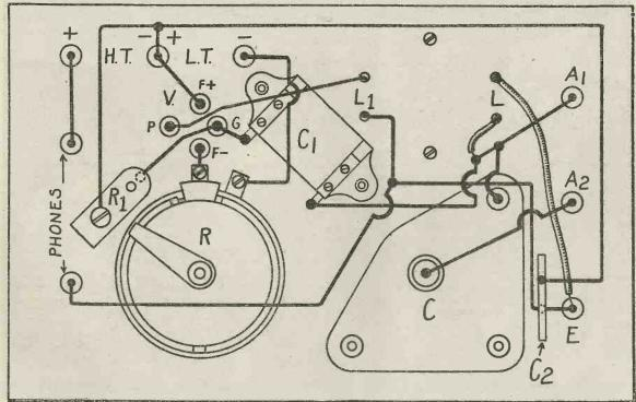
Fig. 6. Practical back-of-panel wiring diagram.
