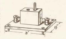
Fig. 16.—Anode or choke coil stand.
