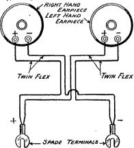
Fig. 1.—Telephone lead connections.
