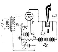
Fig. 1.—An interesting method of obtaining grid bias.
