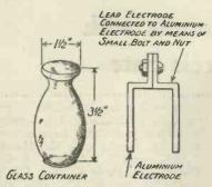
Figs. 1 and 2.—Illustrating the jar and method of connecting the electrodes.
