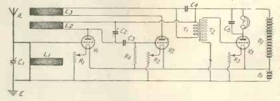
Fig. 2-A double reaction circuit for the "Omni."
