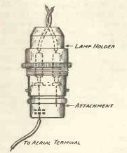
Fig. 2.—Principle of the plug-in attachment.
