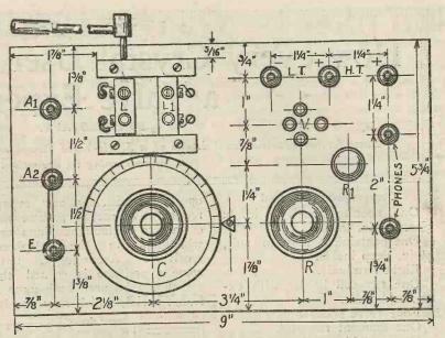
Fig. 7.—The layout of the panel showing dimensions.
