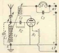
Fig. 3.—The theoretical circuit.
