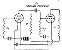
Fig. 2.—How units are coupled.
