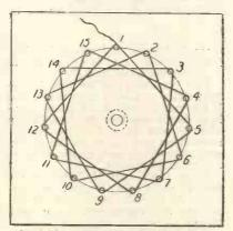
Fig. 1.—One complete "layer" of the coil.
