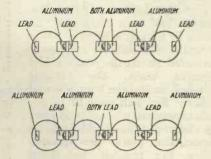
Fig. 3.—The complete rectifier with electrodes in position.
