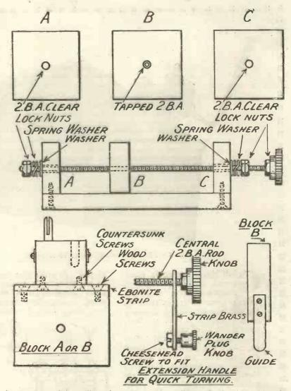
its most useful quality—it needs a large number of turns to move the block B a small distance. This can be remedied by adding a handle to the knob, made of a strip of brass, and fitted with a small auxiliary knob as indicated in the lowest figure.
