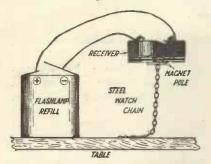
Fig. 4.—A polarity test for telephone connections.
