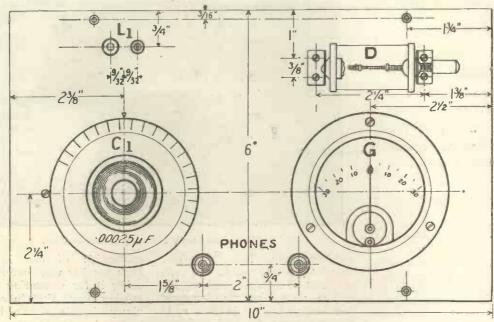
Fig. 4.—Half scale drawing of top of panel.
