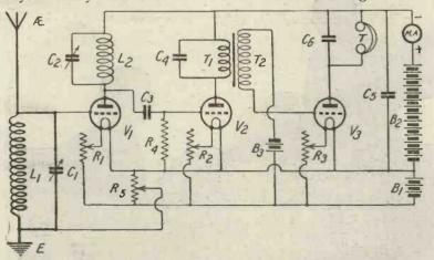
Fig. 1.—Indicating position of milliammeter when using a common H.T. voltage for all valves.
