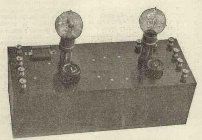
A detector and note magnifier panel which has been used for fifty-metre reception. Note external grid leak clips.
