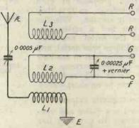
Fig. 6.—Three coil tuner for the Fig. 5 circuit.
