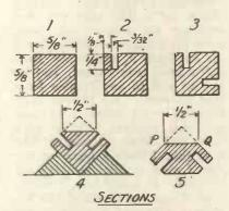
Fig 6.—Preparation of the corner ribs.
