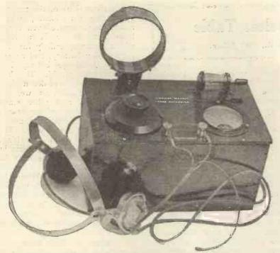
The telephones are used for calibration. Indications of resonance are visual.
