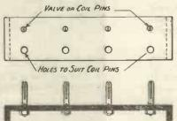
Fig. 1.—How the rack for plug-in coils is made.
