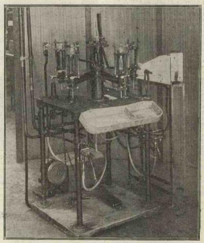
A "pinch" making machine at the Marconi Osram valve works.
