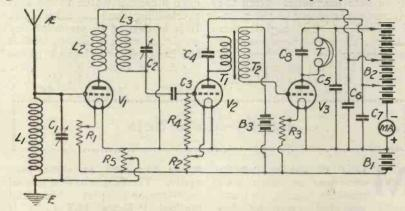
Fig. 2.—Showing position in which milliammeter should be used when employing three separate H.T. tappings.
