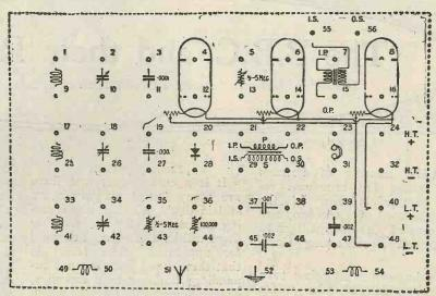
Fig. 2.—The terminal board.
