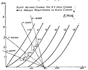
Fig. 7 .- Plate voltage change for 4-volt grid changes with various resistances.
