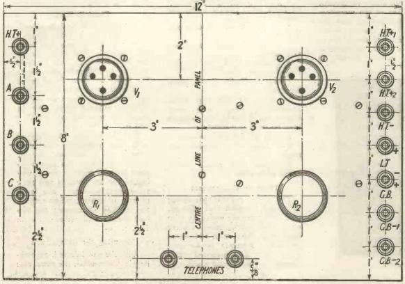
Fig. 5 .- Drilling plan to half scale.
