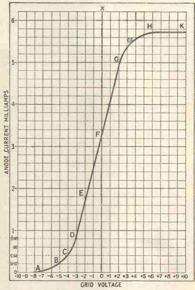
Fig. 10.-A characteristic curve of a three-electrode vacuum tube.
