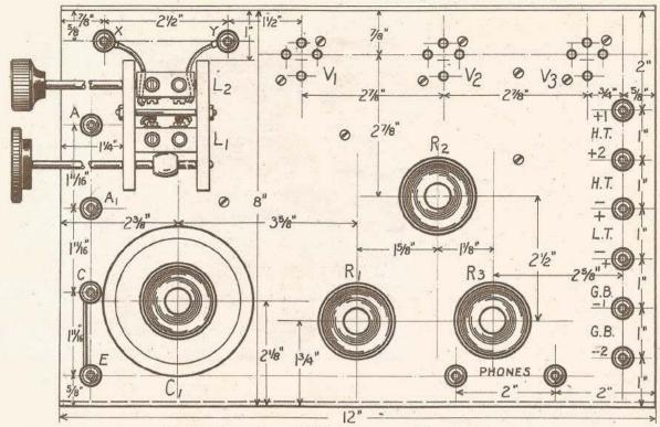
Fig. 6 .- Front of panel drilling diagram. Blueprint 68a.
