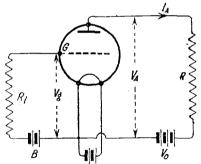
Fig. 1.—A resistance amplifier unit.
