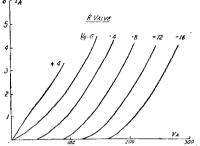
Fig. 5.—Curves for an R valve.
