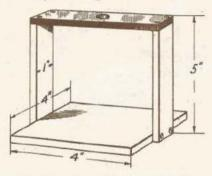
Fig. 15.—Stand for "one-hole" fixing components.
