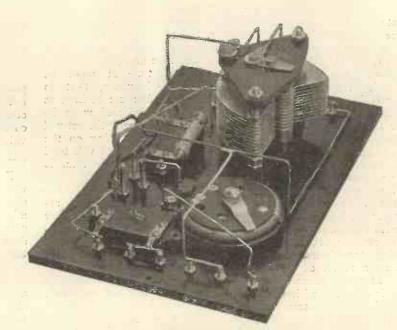
Fig. 2.—Back of panel wiring.
