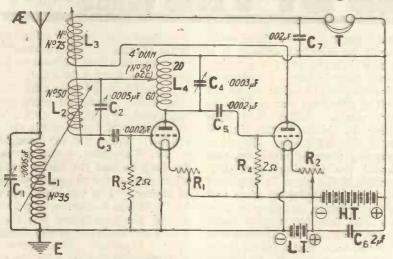
Fig. 3 .- A practical "neutral-grid" broadcast receiver.
