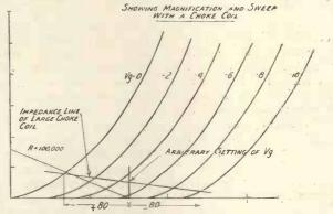
Fig. 10.—Showing magnification and sweep with a choke coil.
