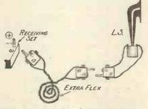
Fig. 2.—Method of making extensions.
