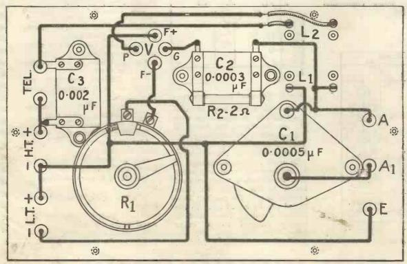
Fig. 6.-Practical wiring diagram of the instrument.
