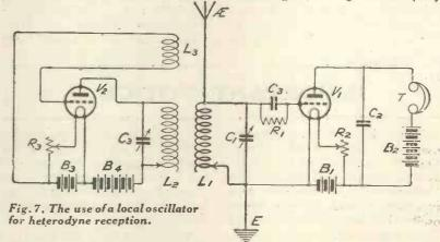
results in a greater selectivity, but heterodyne reception enables us to differentiate between two or more continuous wave stations all working on wavelengths very close to one another. The following example will make this clear.
