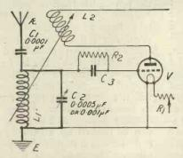
Fig. 1.—A simple aerial tuning circuit using constant aerial tuning.
