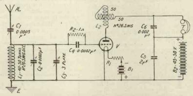
Fig. 2.—A circuit which will tune all short-wave B.B.C. stations on one inductance. The variometer may be loaded with a 0.0003 μF fixed condenser for higher ranges.
