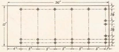
Fig. 3.—Drilling details of the board.
