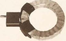
Figs. 9 and 10.—This is a good method of attachment (covered by Burndept patents) employing a binding of adhesive tape and a segment of fibre.
