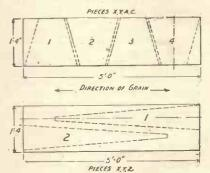
Fig. 3.—Cutting out the parts.
