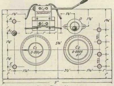
Fig. 4.-The panel lay-out.
