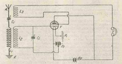
Fig. 3.-A double-grid value arranged in such a manner that both grids take active part in the operation of the circuit, in addition to lessening the space charge.
