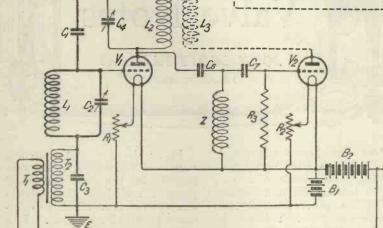
Fig. 2.-Introducing reaction, without the risk of causing interference.
