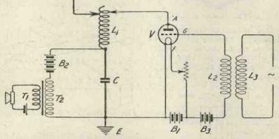
Fig. 51.—A theoretical arrangement in which the output of the value is varied by altering its anode voltage.
