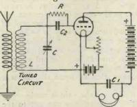
Fig. 11.—A more conventional circuit using the triode valve. An improvement upon Fig. 9.
