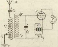
Fig. 2.- A successful trench set operating without a high-tension battery.
