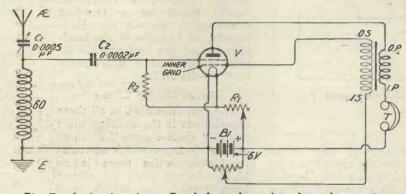
Fig. 7.—A circuit using a Dutch four-electrode valve. A re-action coil may be connected in the anode circuit of the valve.
