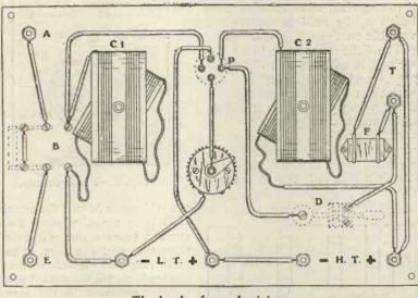
The back-of-panel wiring.
