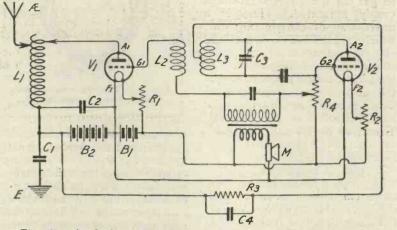
Fig. 50.—A telephone transmitter using a power value V1 and a master oscillator V2.
