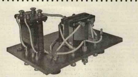
Fig. 2.-Note that the transformers are arranged at right angles.
