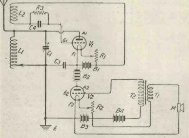
Fig. 46.—The microphone potentials vary the current in the anode circuit of V1 by varying the resistance of V2.
