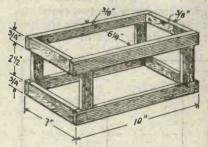
Fig. 10.—A dimensioned view of the framework.
