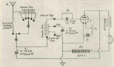
Fig. 1.-The single value circuit diagram. The fixed aerial condenser is made of flex wire.
