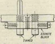
Fig. 1 .- A suggested method of mounting coil sockets.
