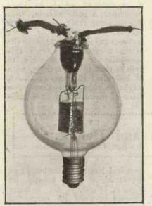
An original De Forest Audion, the first three electrode valve. The plate and grid leads issue from the top of the bulb.
