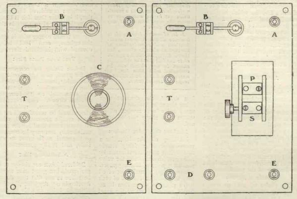
Fig. 1b.-Top-of-panel arrangement of variometer set.
