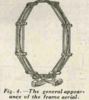
strip is now wound on clockwise, beginning at the supporting strip marked I in Fig. I. It is secured at each crosspiece with a dab of seccotine. Care must be taken to wind on the strip with the flat side downwards. When a complete turn has been made on one side of the hoop the strip is taken across to the other and a second is wound on.
