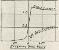
Fig. 1.-Characteristic curve of a double-grid valve.
