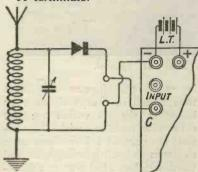
Fig. 3.—Connections for a crystal set.
