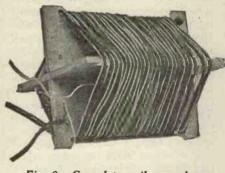
Fig. 8.—Complete coil wound upon second type of modified Harris former, the former being made of wood.
