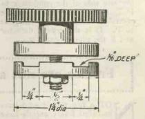
Fig. 3.—Details of the switch knob.
