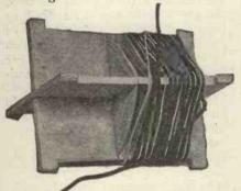
Fig. 10.—The coil shown in Fig. 8 with greater part of outer winding removed to show inner coils.
