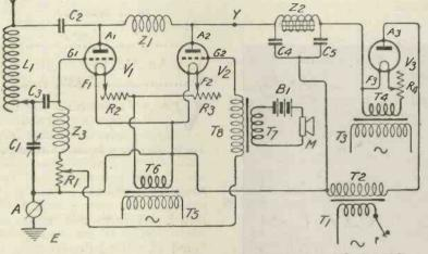
Fig. 45.-A choke control transmitter using rectified A.C. for H.T.
