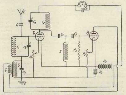
Fig. 1.—A dual circuit employing an effective method of overcoming low frequency reaction.
