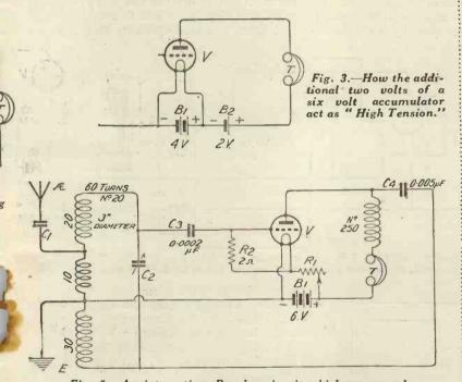
Fig. 5.—An interesting R valve circuit which gave good results at 13 miles.
