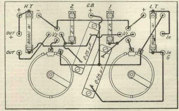
Fig. 5.—The detailed wiring diagram. Blueprint No. 38.
