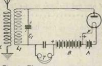
Fig. 4.—The circuit used by Dr. Fleming employing the two electrode valve.
