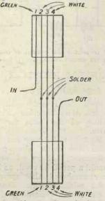
Fig. 2.—Showing how the joints are made.
