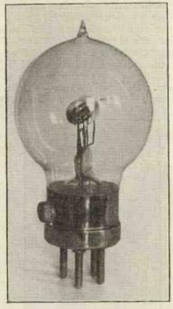
The Phillips' four-electrode value used in these experiments.
