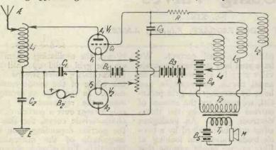
Fig. 54.—Another form of the Fig. 53 circuit; in which a single source of filament current is used.
