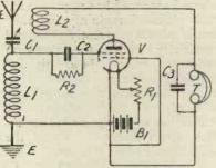
Fig. 3.-A circuit using a dcuble grid value.
