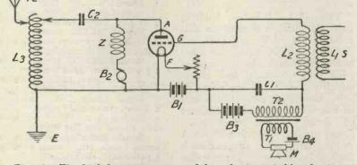
Fig. 48.—The high frequency output of the value is varied by altering the grid potential by means of the microphone.
