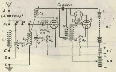
Fig. 4.-The circuit arrangement of the receiver.
