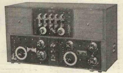
A Marconi portable receiver for waves from 300 to 6,000 metres. It is resistance capacity coupled.
