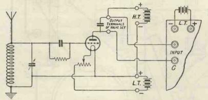
Fig. 2.—How to connect up a valve detector to the amplifier. The whole of the detector circuit is shown for clearness.
