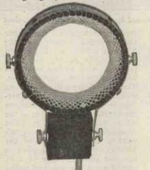
The "Diamond" Sunflower coil, a new type of tuning inductance. 7/22's cable. This gave on an efficient loud-speaker undistorted speech with every word audible the length of a large garden. Accordingly, with ordinary types of apparatus such an aerial should give a fair measure of loud-speaking for, *e.g.*, a small room, with this cable.
