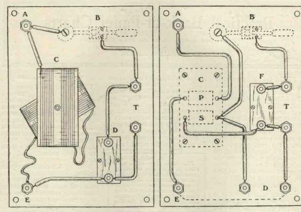
Fig. 1a.—Back-of-panel view of a variometertuned crystal set.
