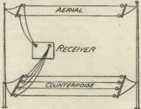
Fig. 4.—Diagrammatic representation of a counterpoise earth.
