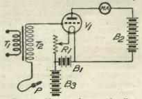
Fig. 2.—Showing how grid cells are used. The milliameter M.A. indicates the effect of a given grid potential.
