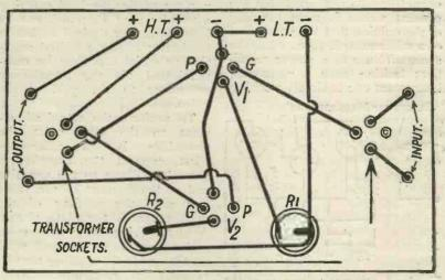
Fig. 5.—Working diagram of the internal connections. 450 March 12, 1924
