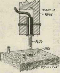
Fig. 1.-Details of the pivot.
