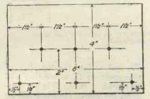
Fig. 28.—Layout of the panel and drilling dimensions.
