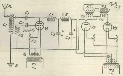
Fig. 24.-- A complete value transmitter in which a full wave rectifier is employed.
