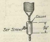
Fig. 1.-Illustrating the drill "stop."
