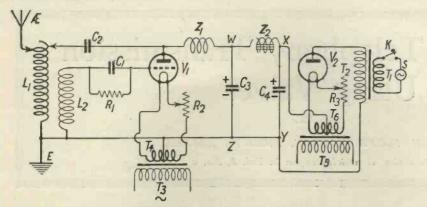
Fig. 22-A circuit for high-power transmission
