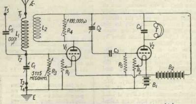
Fig. 1.—A useful circuit for short wave reception in which are incorporated terminal arrangements for varying the methods of aerial tuning.
