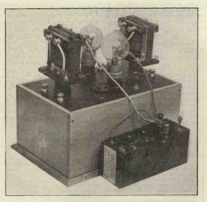
Fig. 1.—Note the method of applying negative bias to the grids of the values.
