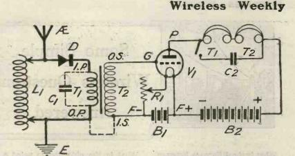
Fig. 27.- A circuit formed by connecting the units already described. The valve V1 acts as a low-frequency amplifier of the signals received on the crystal circuit.
