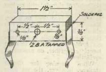
Fig. 3.—Constructional details of the slider.
