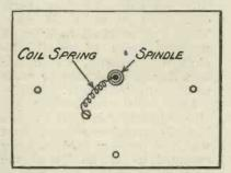
Fig. 5.—How to fit a spring contact to a condenser spindle.
