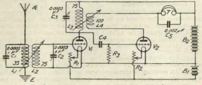
Fig. 2.—One of the best methods of eliminating A.C. hum.
