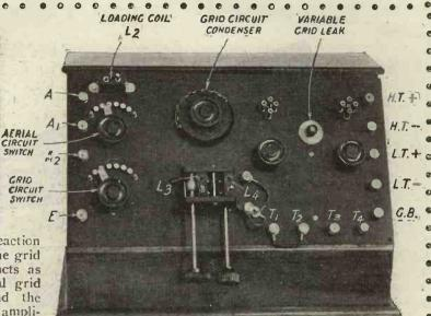
this method of tuning, the aerial is connected to A2, leaving A and At free. In this case the only tuning that has to be done is effected by means of S2, and the variable condenser, using the reaction coil as before.
