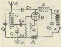
Fig. 18-A single-circuit arrangement involving a pair of condensers in series, a middle connection being taken to the filament.
