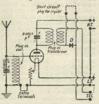
Fig. 2.—The simple circuit used. Extra terminals are for the reflex transformer when fitted.
