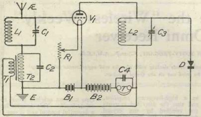
Fig. 2.-A single-value dual circuit which may be obtained on the Omni Receiver.
