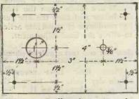
Fig. 24.—Drilling dimensions of the panel.
