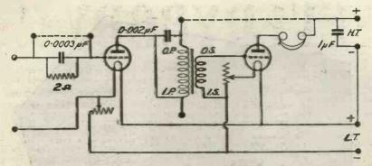
The Circuit used. Note additional terminals for transformer primary.
