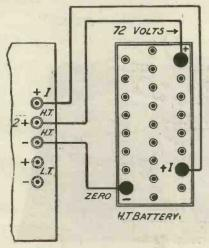
Fig. 4.-The H.T. terminal arrangement.
