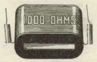
Fig. 2.- A typical 1,000 ohm bobbin.
