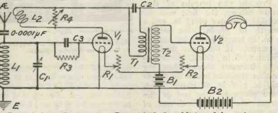
Fig. 2.- A similar circuit to Fig. 1, with the addition of the resistance R4, The condenser C2 is now fixed.
