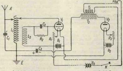
Fig. 21-A complete transmitting circuit using rectified A.C.
