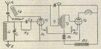
Fig. 1.-A two-valve circuit using direct reaction on the aerial.
