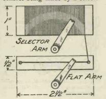
Fig. 1 .- Showing method of mounting the vernier attachment.
