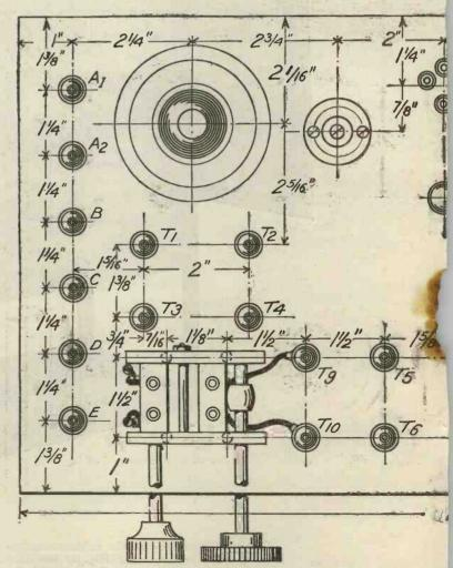
Fig. 3.—A half-size drawing, showing the layout of the parts on the 1
