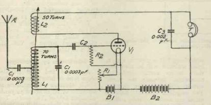
Fig. 1.- A specially useful circuit where interference is troublesome.
