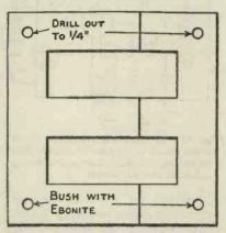
Fig. 1.—Illustrating how the holding bolts should be insulated from the core.
