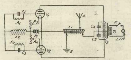
Fig. 25.—Use of A.C. for transmission employing both half-cycles.
