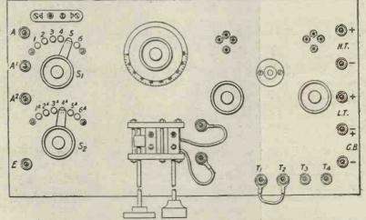
Fig. 7.-Showing the lay out of the parts upon the panel. 461
