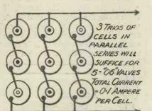
Fig. 4.—Method of connecting dry cells for five ".06" values.
