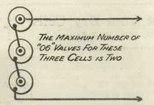
Fig. 3.—Arrangement of dry cells for two ".06" valves.
