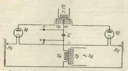
Fig. 23.—A full wave rectifier employing two 2-electrode values. 484
