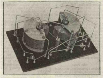
Fig. 4.-Underside wiring. Stiff wire is used throughout.
