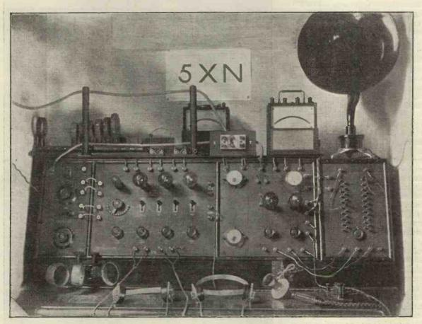
Our photograph shows the transmitting and receiving station of Mr. Everitt, of Eltham, S.E.9. The microphone is seen by the side of the transmitting key. The receiver (on the left) is a standard Burndept instrument.
