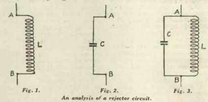
Now let us join our inductance and condenser in parallel, as shown in Fig. 3, and let us suppose that the resistance of both branches of the circuit is really Next let us apply an zero. alternating E.M.F. across the points A, B. Alternating cur-rents will flow through both L and C. The current in L lags behind the applied E.M.F. by 90 deg.; that in C leads it by the Therefore, the same amount. currents in these two branches are 180 deg. out of phase, i.e., they are exactly opposite in phase.
