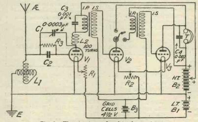
Fig. 3.-The circuit employed in the receiver.
