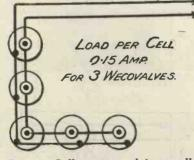
Fig. 2.—Cells connected in parallel for supplying current for three Wecovalves.
