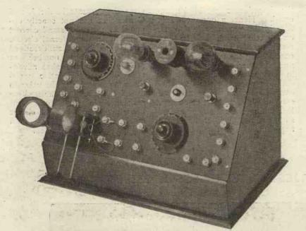
Fig. 1.—A photograph of the complete set, with valves, coils, and transformer in position.
