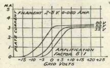
Fig. 4.—Characteristic Curves of the D.E.3-type valve.
