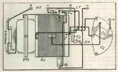
Fig. 6 .- Wiring diagram of the receiver.
