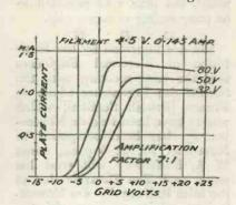
Fig. 1.—Characteristic curves of the Penton valves.
