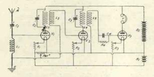
means of which a positive potential can be applied to the grids of the high-frequency valves, will probably effect a cure. Alternatively, the method known as reversed reaction may be used. This consists in using a reaction coil so connected that it damps the oscillations in the aerial circuit, instead of assisting them.
