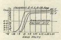
Fig. 3.—Curves obtained with the ARo6 type valve.
