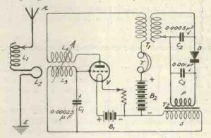
Fig. 3.—Circuit arrangement of the receiver.
