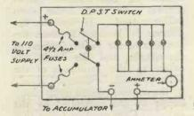
Fig. 1.—Showing connections of charging board.
