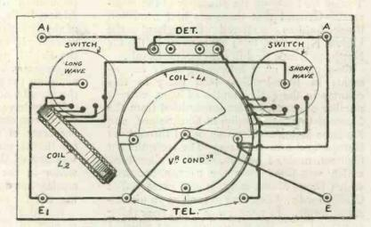
Fig. 6.—A "back-of-panel" wiring diagram.
