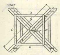
Fig. 3.—Showing details of reels.
