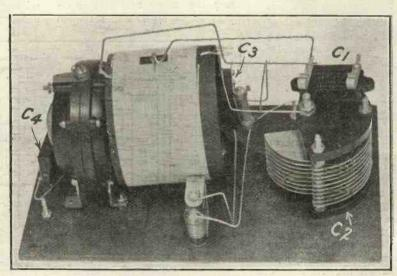
Fig 2.—A view of the internal arrangement of the set. Note the position of the centre tapping on the coil.
