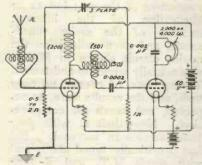
Fig. 1.—A complete short-wave receiver, 150/220 metres.
