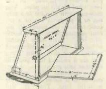
Fig. 6.—Constructional details of the containing cabinet.
