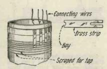
Fig. 6.—Showing how to tap coils by the method described.
