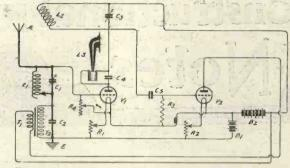
Fig. 2.—The ST150 Circuit with the stabilising resistance shoun between grid and filament of the first valve.
