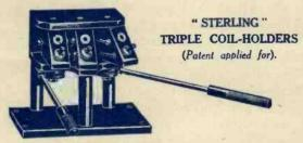
These coil-holders give the best tuning results with any standard plug-in coils. The extended handles provide the usual lateral adjustment, and also control the new patent "Sterling" Vernier adjustment. The sloping face of the coil-holders allows the coils, when inserted, to be inclined at an angle upwards, thus minimising hand capacity effects.
