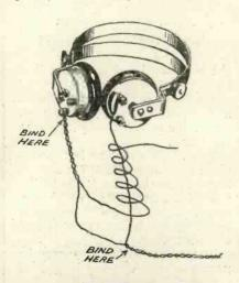
Fig. 4.—Illustrating the method of connecting the 'phones.
