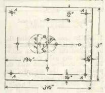
Fig. 8.—Dimensions of panel and positions of drill holes.
