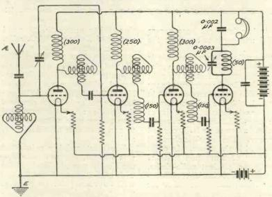
Fig. 3.—Four tuned-anodes. Illustrating the stability obtainable:
