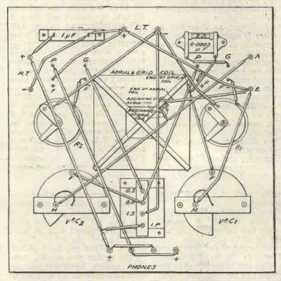
Wiring diagram of the receiver.
