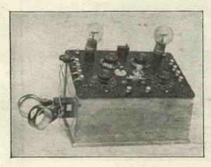
Fig. 3.-An ST150 Receiver in panel form.
