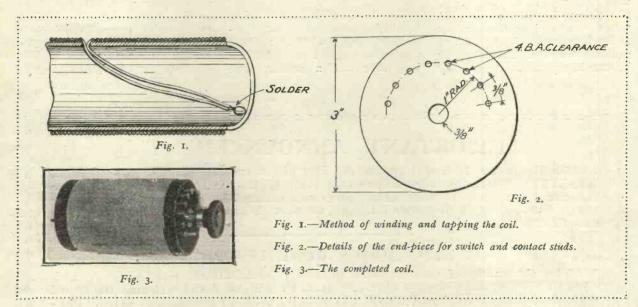
For all-round efficiency on the short wavelengths the single-layer coil stands by itself. Its capacity is of the smallest, since the difference of potential between adjacent turns is very small indeed. It can be exactly duplicated without difficulty, and it is very easy to make.
