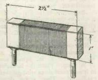
Fig. 6.—The finished resistance.
