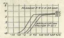
Fig. 2.—Curves given by the B5 type valve.
