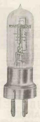
Three ordinary dry cells in series will run one of these valves for 800 hours. current consumption is 0.06 Filament voltage 2.4 to amp. Plate voltage 30/80. 3.0.
