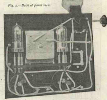
by means of plug-in coils and a series condenser in order to ensure the efficient reception of the shorter wavelengths. Aerial reaction is employed, and readers are warned that when using this receiver for purposes of broadcast reception, every effort must be made to prevent the receiver from energising the aerial, by careful and deliberate adjustment of such reaction.
