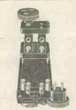
No. 11. Tuned Anode and Reaction Panel 12/6
