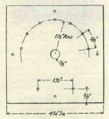
Fig. 3.—Dimensions of panel.
