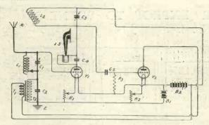
Fig. 1.—The ST150 Circuit.
