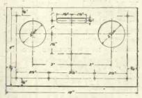
Fig. 4.—Drilling plan of wooden panel.
