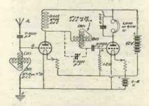
Fig. 4.—A practicable non-oscillating broadcast receiver.
