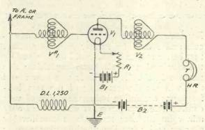
Fig. 4.—The Circuit "D" a replica of the Autoplex
