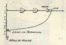
Fig. 2.—Arrangement for fixing counterpoise at house end.
