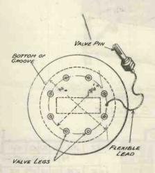
Fig. 2.—Plan of the bobbin.
