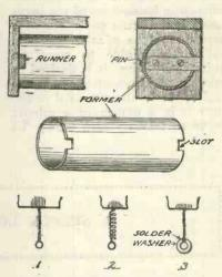
Fig. 6.—Details of the Former and Runner.
