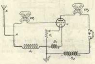
Fig. 1.—The Circuit Diagram of the Autoplex Receiver. With hard valves, the usual gridleak and condenser may be found necessary.
