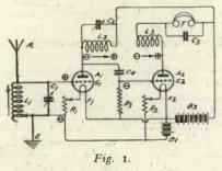
There is, however, rarely any necessity for a trial and error method of connecting the leads to the reaction coil, and such a method is often inconvenient when a panel set is being constructed, and may be obviated by noting the following rules which are based on the two coils which are to be coupled being wound in the same direction.
