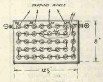
Fig. 1.—Showing method of connecting the cells.
