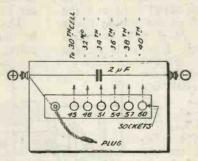
Fig. 2.—The plug and socket arrangement.
