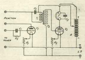
The desired effect can be obtained by using a tapped H.T. battery, as shown.
