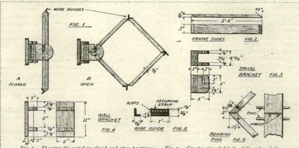
Fig. 1.—Showing the aerial in closed and open positions. Fig. 2.—Constructional details of the sides of the frame. Fig. 3.—The suivel bracket. Fig. 4.—Details of the wall bracket. Fig. 5.—Constructional details of the guides securing the aerial winding. Fig. 6.—Dimensions, etc., of the bearing pins.
