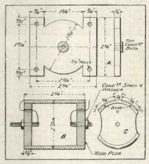
Fig. 2.—Constructional details of the variometer.
