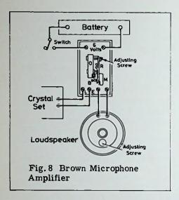
poles could be worked to the reed without actually touching, the greater the magnification obtained from the instrument.
