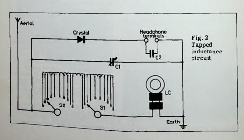
by the rotating arms S1, S2. The loading coil LC was used when receiving long wave and was a plug-in type No. 150 or 200. The loading coil was sometimes short circuited, by the means of a switch, when receiving the ordinary broadcast band. Condenser C2.002 $\mu$ F. across the headphones, was a by-pass for any high frequency pulsations of current.
