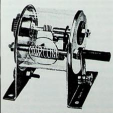
Fig. 7 The Marconiphone automatic crystal detector
