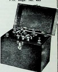
Clear and loud reception is readily obtained over a range of 25 miles under favourable conditions. Receives on wavelengths between 200 and 500 metres. Special type Cat's-Whisker Detector and super-sensitive crystal. Special provision made for the addition of a Valve Note Magnifier.
