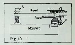
its position owing to the pull of the permanent magnet. The Disc adjustment may not be sufficient to overcome this, and a slight turn of the adjusting screw towards "Open" will be necessary, but is should be realised, of course, that a fresh adjustment of the Disc may be needed.
