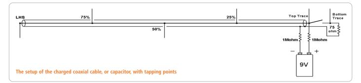
capacitor, made of 50 ohm coaxial cable, is slowly charged up to 8V from a voltage supply via a large resistor. It is then suddenly discharged by closure of a reed relay into a long 50-ohm
