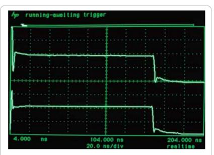
Figure 1: Bottom Trace: The bottom trace probe is across the 75 $\Omega$  terminator used as a trigger. It shows a pulse of the half battery voltage (actually 8V after the 2 x 1M $\Omega$  resistors and the probe loading);
