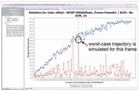
Figure 3: Worst-case response times (by decreasing priority of the frames) obtained by analysis (blue curve) versus maximum values collected by simulation. The trajectory that was simulated here is the one leading to the worst-case response time for a specific frame. As the black circle shows, the worst-case response time for that frame is close to what can be obtained by simulation
