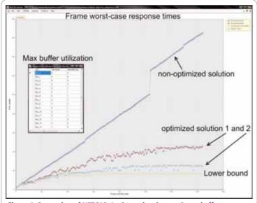
**Figure 1:** Screenshot of NETCAR-Analyzer, showing maximum buffer utilization and CAN frame worst-case response times (by decreasing priority) for different offset configurations. This graph shows the typical gain one can expect with offsets engineers to use more and more bandwidth, a trend that has never decreased since. CAN bus data rates have doubled (e.g. 250kbit/s for a body network when it used to be 125kbits) and load levels have increased too (to greater than 50%, see [4]).
