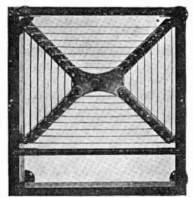
Primary of Transmitting Jigger showing bare Strip Winding.
