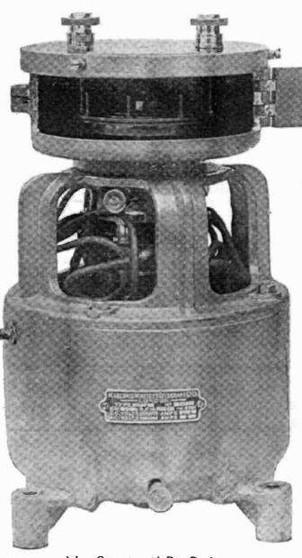
1 k.w. Converter with Disc Discharger.
