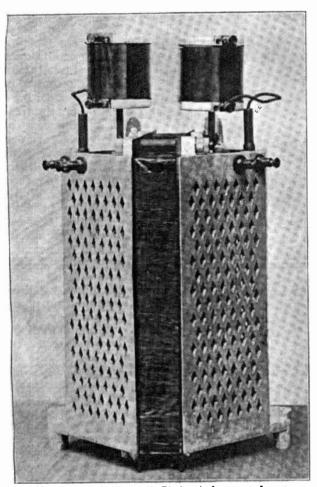
Transformer, k.w. with Choke Colls mounted on top.
