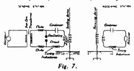
the big weight comes down to hit it, and it follows that the period of oscillation of both must be the same (or in harmonics)—that is to say, both oscillatory systems must have the same time-period, or, in other words, they must be tuned.
