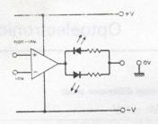
Where the status of the input need only be indicated by a single on/off l.e.d. the other may be removed and replaced by a shortcircuit. If negative feedback is applied then for small differences at the inputs neither l.e.d. will be significantly illuminated.
