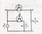
Performance data  $R_1$ ,  $R_2$ : 1.5k $\Omega$  V: 0 to 4V r.m.s. Signal frequency: 10kHz Opto-isolators TIL112  $I_F$  (not shown) 20mA for both opto-isolators. Graph obtained with these values.
