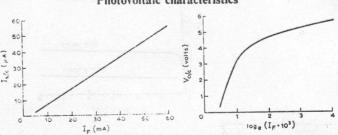
Graph left shows that, over a wide range of  $I_F$  (corresponding to  $I_F > 10 \text{mA}$ ),  $V_{0,c} \propto \log I_F$ . Graph right shows  $I_{S/c} \propto I_F$
