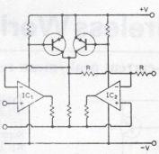
resulting p.d. across R1 falls below level at which Tr1 conducts when input is zero or negative.
