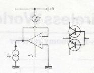
• Using an existing amplifier, add a separate emitter follower to the output, monitoring the current only in the collector of one transistor. A second transistor may be added to retain both polarities of output and present undistorted waveform to oscilloscope if required, and to maintain closed feedback loop, avoiding saturation on negative-going inputs (middle circuit).
