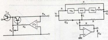
IC1, IC2: General-purpose op-amps tend to oscillate due to additional gain of transistors in feedback path. Heavier compensation of amplifiers such as 301, 748; shunt capacitance from output to inverting input if speed not important. R2, R5: may be omitted if other means used to avoid oscillation (they reduce loop gain in conjunction with R3, R4).
