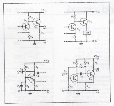
in the circuit shown bottom left. In this arrangement the trigger pulses are applied to the collector of Tr<sub>1</sub> via the small coupling capacitor C<sub>3</sub>.
