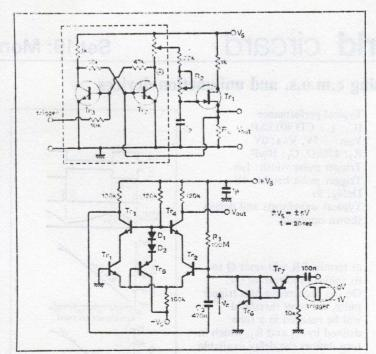
An advantage is that the initial voltage across C2 is always the same at the start of a period no matter the pulse
