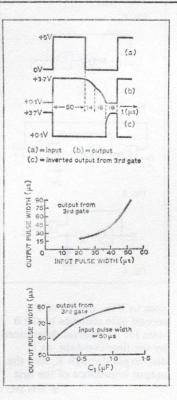
logic 0 and 1 respectively. causing its output to switch to 1 where it remains until the trigger pulse returns to the 0-volt level. During this interval, capacitor C1 discharges towards 0 volt through R1 and the output impedance of the first gate and is recharged to the 1 level after the trigger pulse has returned to the 0-volt level.
