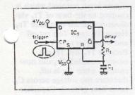
Typical performance IC1: 1 × CD 4013AE V<sub>DD</sub>: +5V, V<sub>ss</sub>: 0V  $R_1$ : 470k $\Omega$ ,  $C_1$ : 10 $\mu$ F
