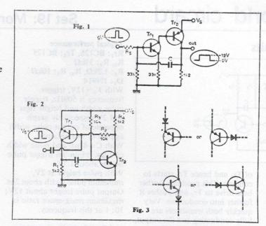
width will depend on  $V_s$ , since in the quiescent state of C is uncharged. In addition the  $V_{\rm CEsat}$  of  $Tr_2$  will affect the height of the pulse which should be  $V_s - V_{\rm CEsat}$ . The 0V level should be well defined. In the circuit over the  $V_{\rm CEsat}$
