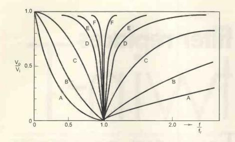
Fig. 3. Positive feedback improves Q of the null filter. These curves show measured frequency response with various amounts of feedback, K.
