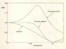
Fig. 1. Amplitude correction scheme uses a filter with a response which is almost exactly complementary over a wide range of frequency to the sin(x)/x roll off inherent in the d-to-a converter. This cancels the roll off to a surprising degree of accuracy, considering the simplicity of the scheme, although the response deviates markedly above half the sampling frequency. However, by this stage, the stopband response of the normal analogue reconstruction filter should give adequate rejection.
