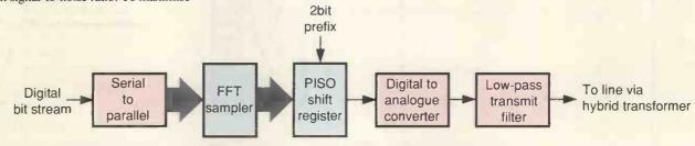
Discrete multi-tone modulation system. While there is nothing new in the processors, vlsi device development for dmt is still at an early stage of development.
