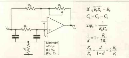
Fig. 1. Basic circuit of the null filter. The resonance dip, d, is amplified to a complete null by the op-amp.
