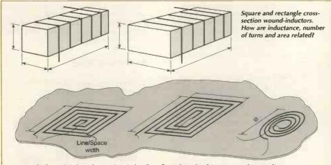
PCB etched or printed conductors in spiral coil configuration, circular, square and rectangle geometries.
