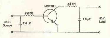
Fig. 6. Circuit for specified gain <optimum gain.
