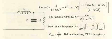
Fig. 1. Impedance and frequency for zero phase of the deceptively simple circuit with series L, cable capacitance and resistive speaker load. Above and below zero-phase frequency, impedance is inductive and capacitive respectively.
