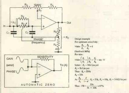
Fig. 5. Wide band tuning. The filter can be used to provide orthogonal tuning in a wider range using a ganged potentiometer.
