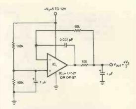
Fig. 1. False or "pseudo" grounds can be made any value desired. When dynamic currents are high, use this simple op-amp follower.
