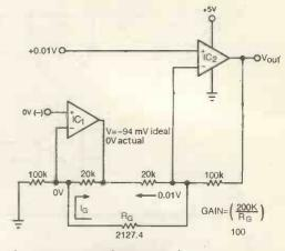
Fig. 4. Two op-amp instrumentation amplifier normally uses two supplies. Using a single supply constrains the design's common-mode range.
