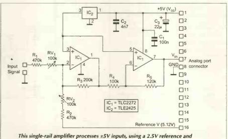
This single-rail amplifier processes ±5V inputs, using a 2.5V reference and the 5V supply from an interface connector.
