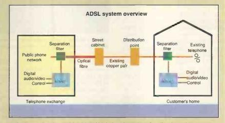
Telephone television. With adsl, 16kbit/s data from the subscriber is used to access a one-way broadband video signal from the exchange.
