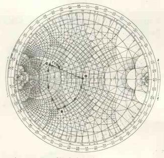
Fig. 10. Input matching for low noise.
