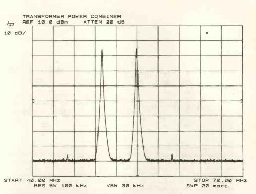
Fig. 3. The spectral plot delivered by the practical implementation of Fig. 2 demonstrates the splitting action, giving equal outputs at ports 2 and 3.
