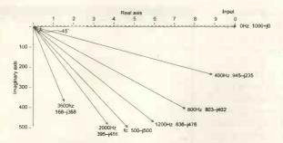
Fig. 6. A few of the output voltage phasors represented by the Nyquist Plot of Fig. 45 show how the almost semicircular curve is traced.
