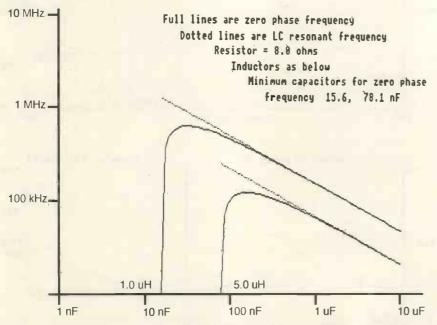
Fig. 2. Zero-phase frequency against C, with L of 1 $\mu$ H and 5 $\mu$ H and an 8 $\Omega$  resistor in the circuit of Fig. 1.
