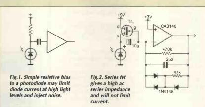
much less than  $V_{dg}$ . Two diodes in the feedback path provide progressive limiting for large signals. A New Fishponds Bristol
