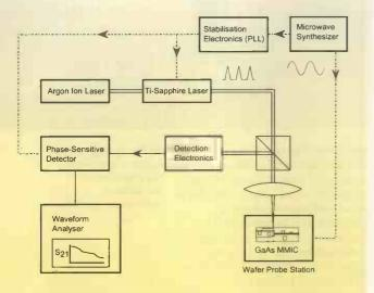
Electro-optic probe station for GaAs microwave integrated circuit measurement.
