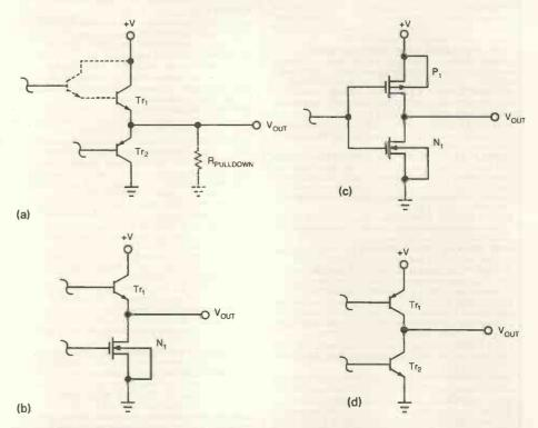
Fig. 7. Output-stage topologies used in single-supply op amps. The bipolar complementary emitter-follower stage (a) is active only to within a diode drop of each rail at best. The bipolar emitter-follower, nmos common-source output stage (b) has by nature, an asymmetrical voltage swing. The cmos stage (c) is, by definition, fully complementary. Complementary-bipolar common-emitter stage (d) is another rail-to-rail output stage.
