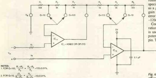
Fig. 6. Instrumentation amplifier that shrugs off switch resistance, enabling gains to be switched.
