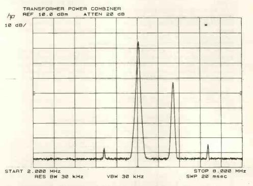
Fig. 4. Demonstrating the isolating action. Port 3 is connected to the spectrum analyser while port 1 has 5MHz signal applied (centre) and, at the same time, port 2 has a 6MHz tone applied. Both signal generator output levels are equal. The isolation achieved is about 30dB.
