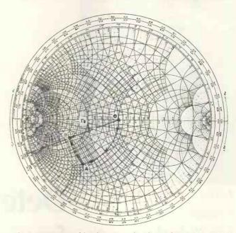
Fig. 2. Output matching for narrow band, match-for-optimum-gain,  $S_{12} = 0$ .
