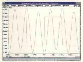
Fig. 13. When filter input is a 1kHz square wave, well below the pass band, only the 3kHz sine wave component comes through strongly. This transient analysis plots the filter's 1kHz square input and 3kHz sine output.
