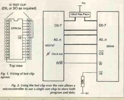
controller can use sleep mode. Do not leave i/o pins floating, as that increases current drain. The  $1M\Omega$  resistor pack stops the data bus floating.
