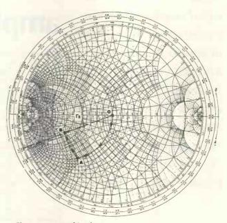
Fig. 4. Input matching for  $S_{12} \neq 0$ .
