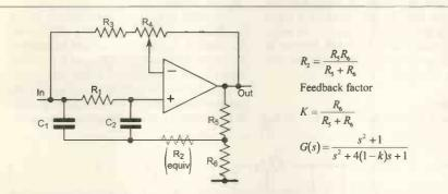
Fig. 4. Positive feedback can improve the circuit. Part of the op amp output is fed back to  $R_2$ .
