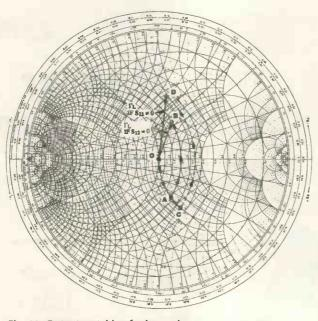
Fig. 11. Output matching for low noise.
