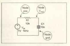
Fig. 1. Nodes of this simple low-pass filter are named, ready for entering in as a SpiceAge netlist.
