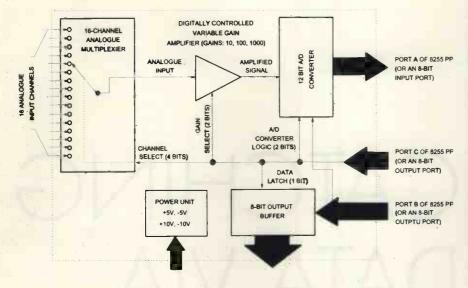
plexer unit is built around two DG508 eightchannel analogue multiplexer ICs, namely  $IC_{1,2}$ . These provide 16 channels of analogue inputs.
