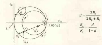
Fig. 2. Plotting V<sub>1</sub>, a circle in complex notation, and multiplying by  $1+R_4/R_3$  in the namplifier gives a zero for V<sub>0</sub> at frequency f<sub>0</sub>.
