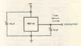
Fig. 2. Use a reference IC that can source and sink current if a precise pseudo-ground voltage is needed. This circuit can handle load currents both into and from the 2.5V source. Low-esr by-pass capacitors help keep the circuit's ac impedance low.
