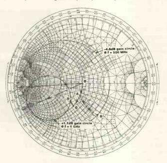
Fig. 7. Input matching for broadband design.
