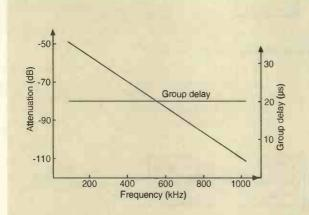
Fig. 1. Rf characteristics of unshielded twisted-pair telephone. While the attenuation might be anticipated, the constant group delay characteristic is fortuitous for a digital system.
