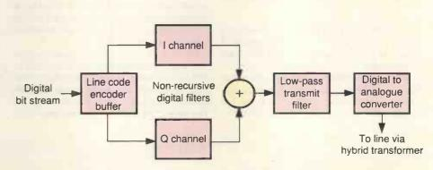
The basic cap modulation system depends on relatively low cost, readily available vlsi chip sets.
