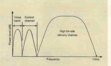
Fig. 2. Frequency-division multiplexing for adsl. This shows clearly adsl's ability to support simultaneous voice, telephony and the subscriber's demand and programme delivery channels.
