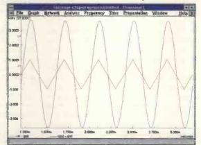
Fig. 12. Band-pass filter of Fig. 10 in action. A 2.5kHz triangle wave is filtered to a 2.5kHz sine wave, all harmonics are filtered out because they are well above the pass band.
