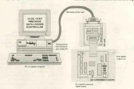
ging system – an a-to-d conversion board and an interfacing card. The former deals with analogue signal multiplexing, amplifying and analogue-to-digital conversion; the interfacing card manages communication between the ato-d board and the computer.
