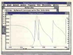
Fig. 11. Transient analysis shows peak response at 2.5kHz, and a fall-off on either side of this at the specified rate.
