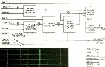
Fig. 4 The STEL2173 Numerically Controlled Oscillator from Stanford, usable for synthesis of up to 400MHz, provides 32-bit frequency resolution (i.e. 0.23Hz at 1GHz clock) and very fast frequency hopping - although the external digital to analogue converter required will add to the settling time.
