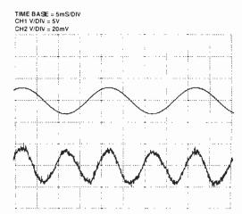
Fig. 3. 5V pk-pk 50Hz input test signal to circuit of Fig. 2 (upper trace) and outphased distortion products (lower trace).
