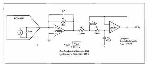
Fig.4. Current-output digital-to-analogue converter, with an OPA2604 converting the current to a voltage and another acting as a low-pass filter.
