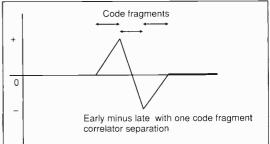
Error signal that advances or retards tracker. Differencing the signals from two correlators that have a small time offset yields a error signal that can control a tracker to keep the receiver in lock with the transmitter.
