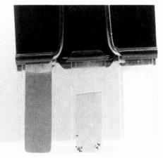
Before, between and after (right to left) exposure to UV. The layered viologen compound left in the dark, exposed to sunlight for 2h, and irradiated with a UV lamp for 2h.
