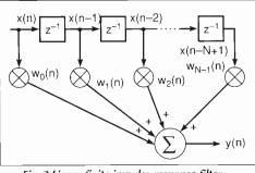
Fig. 3 Linear finite impulse response filter structure
