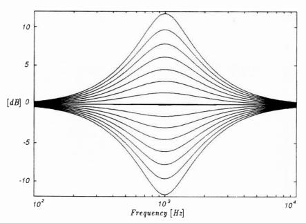
Fig.2. Frequency responses of a single 1kHz equalising section at various code values (0F, 1F, 2F, ..., 7F, 89, 90, A0, ..., F0). Maximum boost and cut is 12dB. Because of the x/(1-x) law, the steps are not equidistant; the lowest is around 1.5dB and the highest is around 2.2dB.
