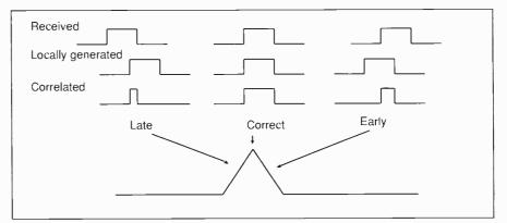
Correlation response of a squared pulse. Recovering a spread-spectrum signal relies on the fact that it can be de-spread when multiplied by the same spreading code again. More than one chip of the code in timing error means no signal, and a single correlator does not know which way to adjust to find the peak. without post processing or p-code.
