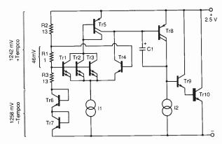
Closing the feedback loop with a bias string. The resistor values refer to multiples of  $750\Omega$ .
