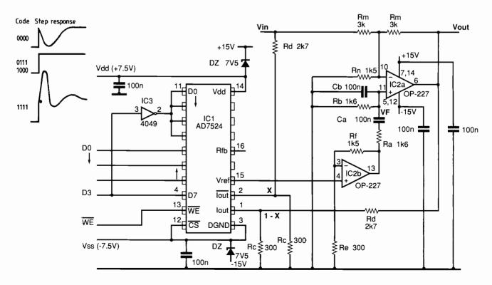
Fig.1. Circuit diagram. Note the ±7.5V DC power supply for the D-to-Aand the data control logic.
