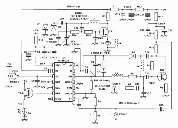
Fig. 8. The GEC-Plessey NJ88C33 evaluation board provides a reference oscillator, a 60 to 80MHz VCO and a simple loop filter to complete a minimal frequency synthesiser loop. The two units allow analysis of different loop variables as well as the selection of comparison frequencies for fast frequency-lopping loops.
