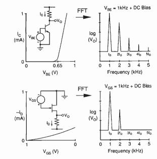
Fig.2. Odd harmonics sound worse than even ones. Fet devices exhibit a square-law transfer characteristic, as against the bipolar exponential curve and therefore generate mostly even-order harmonics.
