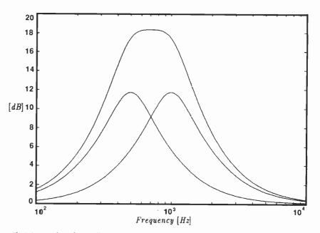
Fig.3. Interaction of two adjacent (one octave apart) sections at maximum boost. The resulting boost is 18dB. If this is undesired, more selective and more complex filter types must be used.
