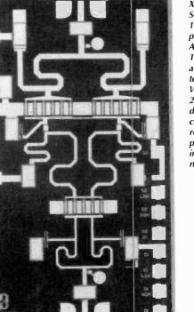
*X-band mmics: Harris Microwave Semiconductor integrated X-band GaAs mmic is 100% tested on wafer for dc and rf performance.*
