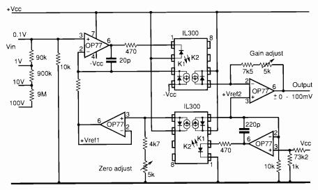
ferential isolation amplifier. Additional isolation comes from the bridge connection of the amplifier on the output side, which combines the inverting and non-inverting inputs to provide a single ended output. Siemens<sup>1</sup> has published differential input circuits operating in both the photovoltaic and photoconductive modes, the former offering a bandwidth of 50kHz combined with a CMRR at 10kHz of 140dB.
