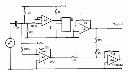
Fig. 2. Test circuit used for evaluating the IL300 operating in positive unipolar photovoltaic mode. Ideally, there should be zero resultant signal at output 2.
