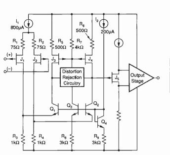
Fig.3. Layout of one section of an OPA2604. The comparatively high input-stage current of 800µA gives higher transconductance and reduces voltage noise.
