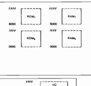
Fig. 1. 64kbyte memory system provides 64kbytes of physical ram virtually overlapped by 64kbytes of physical eprom.
