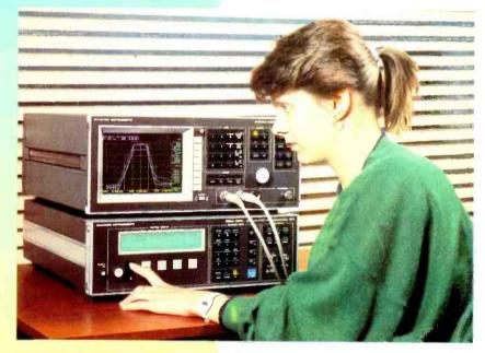
Stephen Gledhill explains how sweep oscillators built around scalar analysers provide a powerful system for analysis of microwave devices. Evaluation of microwave components and sub-systems such as filters, amplifiers, mixers, attenuators, limiters, cables anc waveguides often requires measurement of frequency response.
