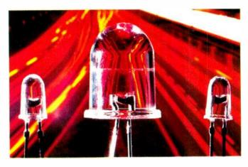
Bright leds. Leds from Hewlett-Packard in a material whim sically called transparent-substrate aluminium gallium arsenide (TSAIGaAs, for not very short) are much brighter than the average, putting out up to 15 candela at 20mA and at a very narrow viewing angle. They are red (637nm), are compatible with cmos/mos and dissipate 130mW. Jermyn Distribution, 0732 740100.
