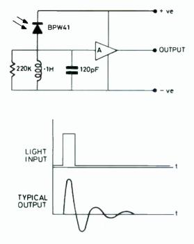
Fig. 4. Inductive loading in (a) provides a signal frequency impedance of 100K2 while giving a very lowresistance path for background lighting photocurrent. Output is shown in (b).
