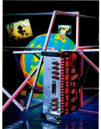
Radstone Technology has added image processing to its mainstream VME products. The first module is a three-board subsystem designed to capture and manipulate images in realtime.
