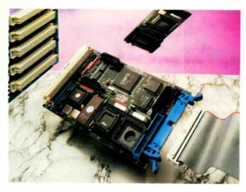
Arcom's latest VME single-board computer uses Intel's i486 as the central processor instead of the Motorola devices at the heart of most of its rivals. The company hopes this will help it to supply boards for VME, PC and STE buses which can work with each other in large systems.
