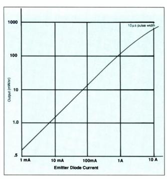
Fig. 1. Emitter current versus infra-red radiant intensity for the ZME41 diode.
