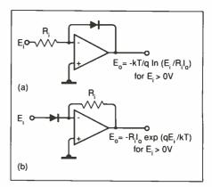
Fig. 2. (a) Logarithmic ampl; ifier with junction connected into negative feedback loop; (b) antilog amplifier.
