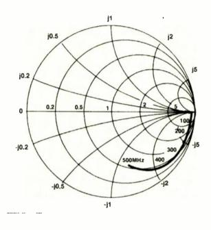
Fig.2. Inputimpedance matching network, of which C<sub>1</sub> forms a part, looks like 50ohms to the source (chart normalised to 50ohms)
