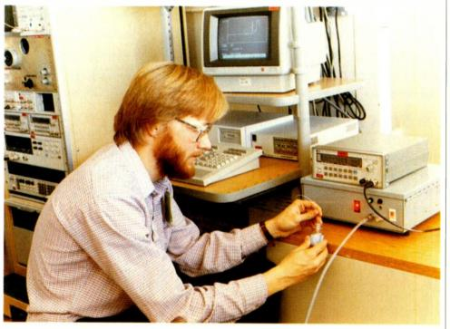
Using an acoustic wave sensor's ability to detect methanol in real-time.
