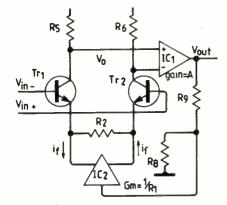
Fig. 3. The cross-quad is represented by the transconductance amplifier  $U_2$ , having  $G_m=1/R_1$ , which feeds currents  $-i_i$  and  $+i_i$  into the input stage.
