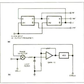
you are using the phasing or the Weaver method. The mixer in (a) maintains good phase integrity at clock rates ranging to several MHz. Clock and operating frequencies are equal in the mixer circuit (b), which gives an advantage over the flipflop design.
