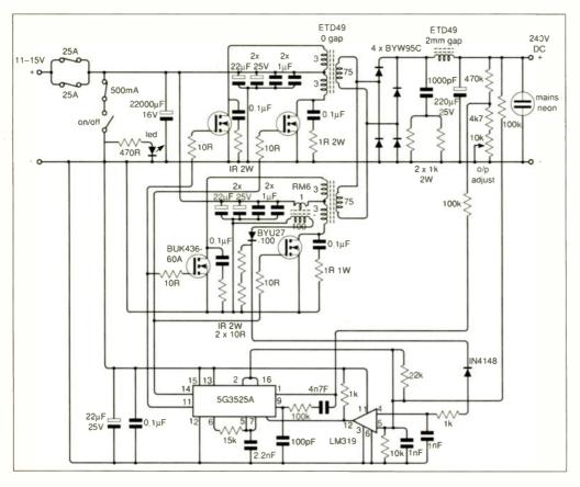
A standard push-pull inverter runs at 25kHz, with regulation obtained from the voltage-mode SG3525A pulse-width modulator from SGS-Thomson. Current-limit shutdown is achieved by sensing the current in the centre tap of one of the transformers (not both, since they are identical), an op-amp comparator driving the shutdown IC input. Threshold of current limit at the comparator is reduced when the inverter input is very low to compensate for delay in shutdown.
