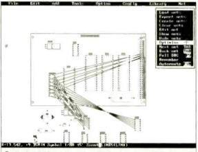
Optimized placement by displaying ratsnest per component. Lines indicate the unrouted nets.
