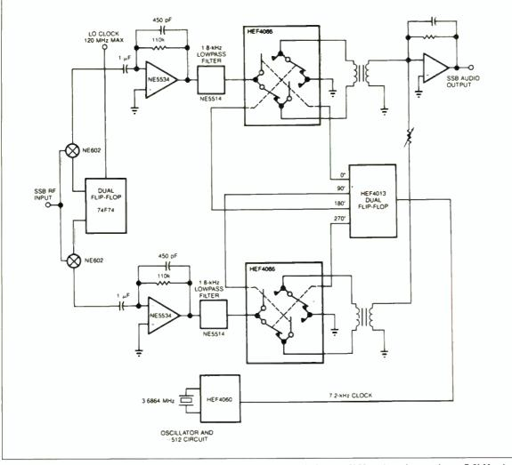
Fig. 8. To minimise power drain, you can use HEF4066 cmos analog switches in the subscriber stage of this experimental Weaver receiver circuit.
