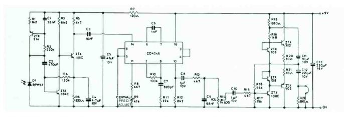
amplifier stage. Consequently the range can be easily extended by either raising the amplifier gain by adding further stages or by increasing the received signal level using a lens with the transmitter led. An experimental system using both techniques operates at over 40m.
