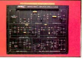
Each F.A.C.E.T. module comprises a number of clearly identified circuit blocks with highly accessible circuit nodes. Connections are made with iumper leads.
