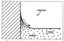
Fig. 1. Using a vapour of water-soluble organic compound directed at the product surface to absorb water.
