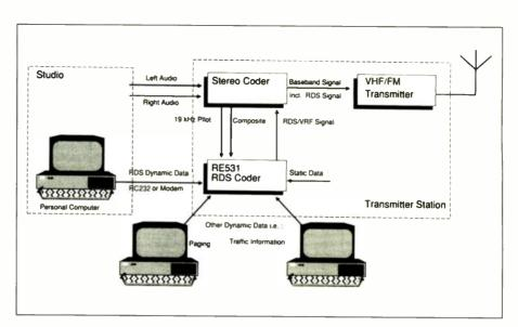
Fig. 2. An RDS network configuration downloading data from PCs to the coder.
