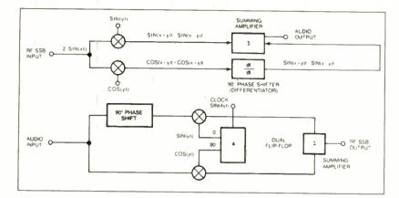
input signal feeds in phase to two RF mixers in the phasingmethod detector (a). A local oscillator (LO) supplies a second signal to the mixers in quadrature. In the generator (b), a divide-by-4 flip-flop provides the sin(vt) and cos(yt) signals for the mixer.
