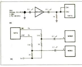
Fig. 5. You can effectively drive the 74F74 and other TTL gates with the circuit shown in (a). The total resistance in the interface circuit (b) establishes a conservative current drain (approximately 10mA) from the 74F74, and the divider tap optimises NE602 operation.
