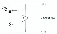
Fig. 3. A commonly used single resistor is the simplest load.
