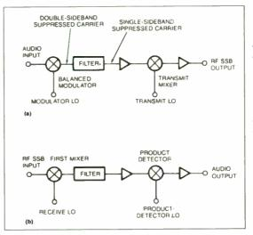
Fig. 1. In the traditional filter method, the generator (a) produces a doublesided signal, and the balanced modulator nulls the carrier. The detector (b) simply reverses the generation procedure to develop the audio output.
