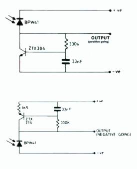
Fig. 5. Two configurations of the same basic active load circuit but with differing output polarities.
