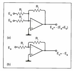
Fig. 1. Basic SAE functions; (a) addition and (b) negation.
