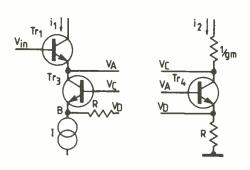
Fig. 1. The circuit is divided into two parts, to analyse the operation of the cascode  $Q_2$ ,  $Q_4$ .
