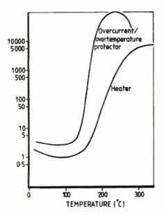
Fig. 2. PTC applications. The steep PTC curve is required for over-current and thermal fuse applications, where the current needs to be switched off quickly. The shallow curve, on the other hand, is more suitable for heaters, where there is a gradual reduction in current as temperature rises.
