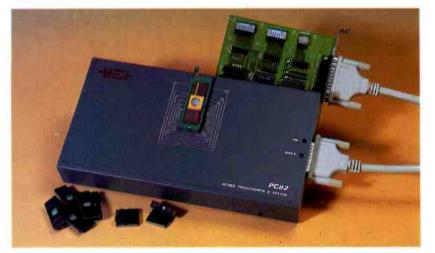
Universal programmer. The complete designer's kit. This will program EPROMS, EEROMS, BPROMS, PALS, GALS, EPLD's, Z8 and 87XX microprocessors. A unique feature is the testing of logic parts such as 74LS393 etc. The PC82 can check and identify parts. Already programmed are the TTL & CMOS logic test vectors. Software is supplied to write vectors for most unique chips. One of the most popular programmers in the USA.
