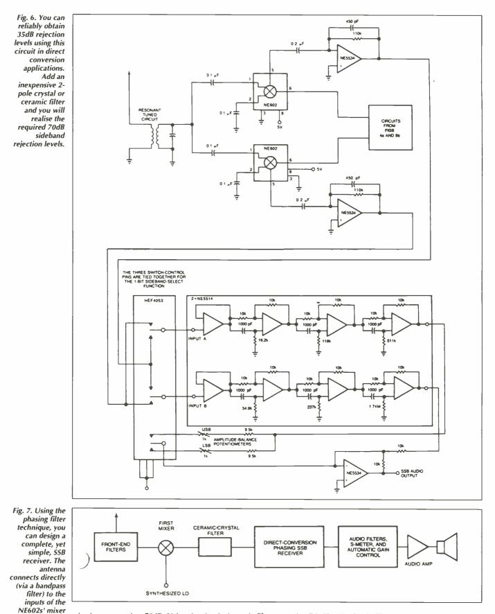
rejection greater than 70dB. Using the circuit shown in Fig. 6, you can reliably obtain rejection levels of 35dB. Add an inexpensive 2-pole crystal or ceramic filter, and you can meet the 70dB requirement. Fig. 7 shows a complete SSB receiver that uses the phasing filter technique.
