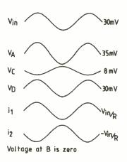
Fig. 2. Linearised cross-quad circuit, together with some waveforms at appropriate points.
