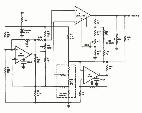
Fig.1. Skeleton circuit diagram of National Semiconductor's LM363 instrumentation amplifier. Two-stage amplifier yields extremely high open-loop gain and gain/bandwidth product, but remains stable at all closed-loop gains.
