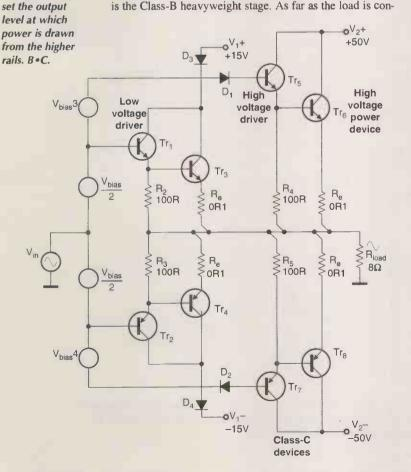
cerned, these two stages are delivering current in parallel. The aim was improved linearity, with the elimination of the bias preset of the Class-B stage as a secondary goal.
