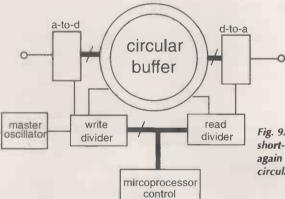
Fig. 9. In pitch shifting, the short-term store is re-used again and again, i.e. it is a circular buffer.
