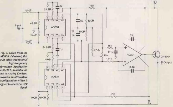
AD834 datasheet, this circuit offers exceptional high-frequency performance. Application note AN212, available on request to Analog Devices, provides an alternative configuration which is designed to accept a  $\pm 2V$
