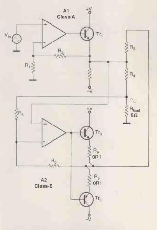
Fig. 1. Sandman 'Class-S' scheme. Resistors  $R_{3,4,5,6}$  implement the feedback loop controlling amplifier  $A_2$  so as to raise the load impedance seen by  $A_2$ .
