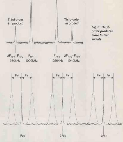
mixer are 980kHz and 1040kHz, and appear close to  $F_{\rm RF1}$  and  $F_{\rm RF2}$ . If the pre-mixer filter selectivity is not sufficiently narrow to suppress the unwanted radio frequency, then the receiver may respond to the third-order products as well as the desired signal.
