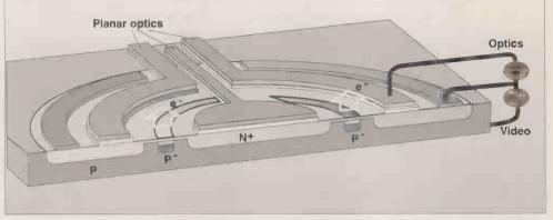
Electrons are emitted from two buried cathodes, each  $1\mu m$  wide and  $25\mu m$  long. Potentials of -30V on the inner disk and +30V on the outer  $100\mu m$  diameter ring produce a field that causes the electrons to leave as a single beam. One of these ring structures, on separate chips, would be required for each electron gun in a colour tube.
