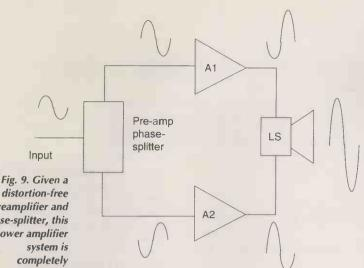
distortion-free preamplifier and phase-splitter, this power amplifier system is completely distortion free, provided solely that the output amplifiers show only even order distortion – 2nd, 4th, 6th etc. harmonics).
