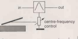
Fig. 6. Normally, a foot pedal is used to control the wah-wah effect's centre frequency.
