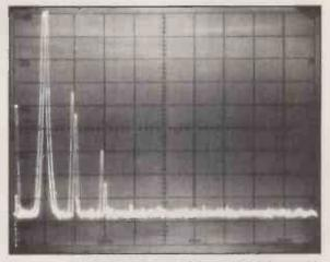
Fig. 6. Showing the performance of the circuit of Fig. 5, with and without 10dB of negative feedback. Span 0 to 10kHz, 10dB/div. vertical, 30Hz resolution bandwidth, 2s/div sweep rate.
