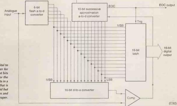
Using a fast digital to analogue converter for the most significant bits and a slower one for the least results in a combined circuit that is still acceptably rapid but less complex and cheaper.
