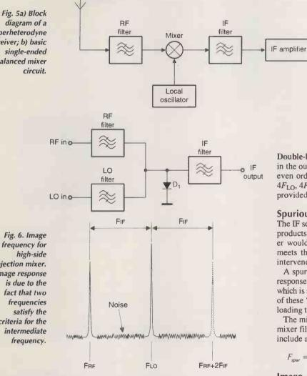
high-side injection mixer. Image response is due to the fact that two frequencies satisfy the criteria for the intermediate frequency.
