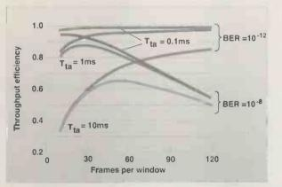
Throughput of the proposed 16Mbit/s IrDA standard plotted against number of frames sent in each transmission window. One hundred and twenty seven frames per window will be allowed, but 60 looks like a better bet, particularly under typical (BER 10-8) conditions. The long turn-around times (Tta), mandated by the current generation of low cost transducers, will also have to be reduced if the 16Mbit/s data rate is to be met.
