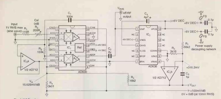
Fig. 4. While using two expensive components, this true rms detector provides an exceptional 80dB dynamic range and a constant bandwidth, which is limited to 2MHz by the AD636. The AD600 variable gain 'X' amplifier has a 35MHz bandwidth.
