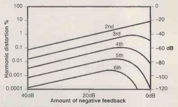
Fig. 1. Effect of different amounts of negative feedback on an amplifier with predominantly second harmonic distortion. (Reproduced by courtesy of Newnes)
