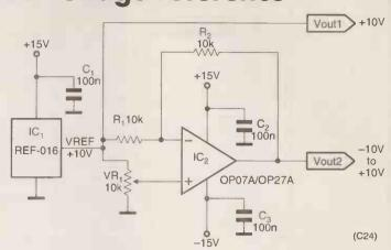
Not only providing a rarely found negative voltage reference, this circuit is fully adjustable from -10V to 10V.
