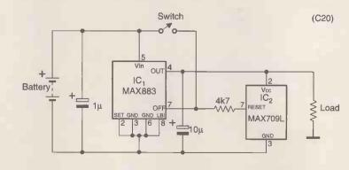
To prevent chatter when battery voltage falls below the threshold of the voltage monitor, the regulator turns off and remains off.
