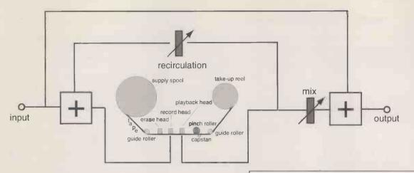
Fig. 1. Early machines produced an echo whose delay time was determined by tape speed and the gap between the record and replay heads. Next generation echo machines fed back some of the replay head output, allowing multiple echoes.
