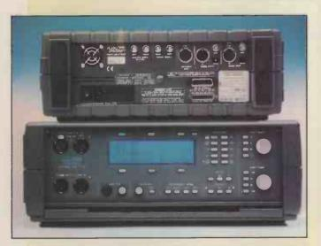
Audio analyser interface. As an option for the Audio Precision Portable One range of audio analysers, Thurlby Thandar can now supply a GPIB interface for both versions of the instrument. The interface controls all the operation of the instruments including the recently introduced digital audio measurement in the dual-domain version for which Visual Basic sample source-code programs are supplied. The Interface is also available as an upgrade.
