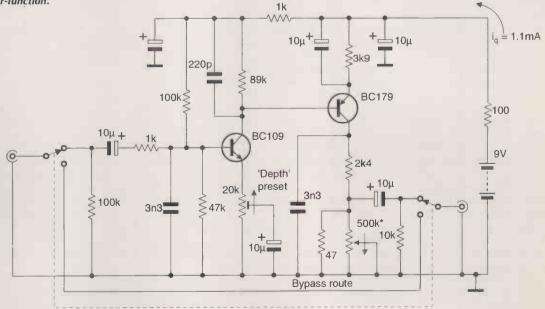
Fig. 5. There are complex digital circuits for producing distortion, but simple analogue alternatives like this one are often preferred. ing asymmetrical distortion, and subjectively this is indeed the case.
