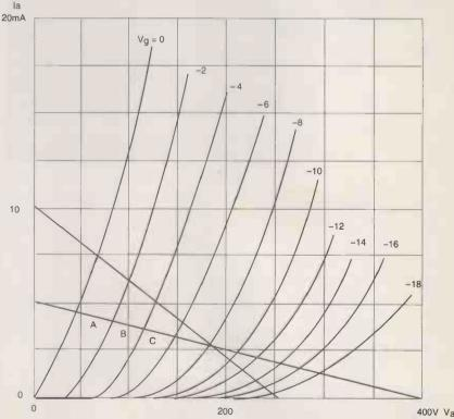
Fig. 2. Anode characteristics of a typical 6J5 triode.
