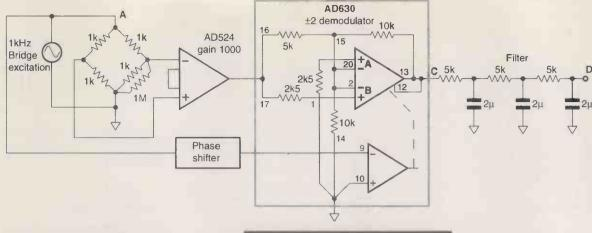
IC from Analog Devices,<sup>6</sup> simplifies synchronous detection. I mentioned this chip in the October 1998 issue, where it was used to recover a wanted signal from overwhelming background noise.
