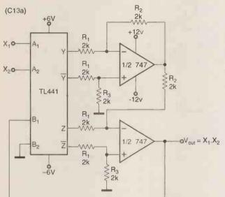
values. If  $R_2 = R_3 = nR_1$ , the output is, for n=1, a multiplier; for n>1 the *n*th power output and, for n < 1, the *n*th root
