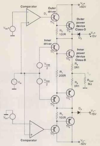
Fig. 9. Class-G output stage with outer devices in Class-D. Described as B+D.
