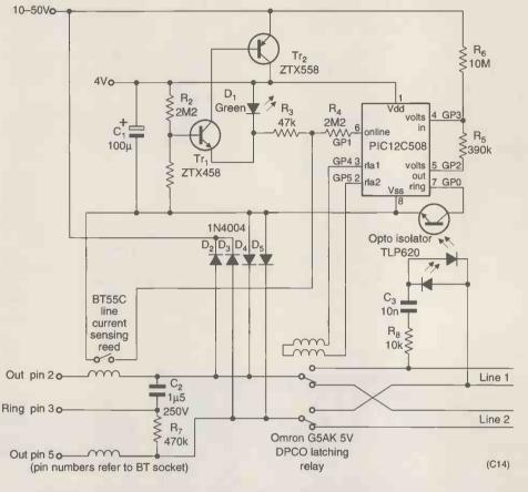
attached 'phone is off the hook to ensure reliable reset for the PIC at startup. The PIC drives a latching double-pole changeover relay, an 8ms pulse at 3.5V minimum from the power supply.
