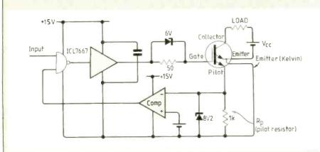
Fig. 2. Using a pilot resistor for overcurrent protection.
