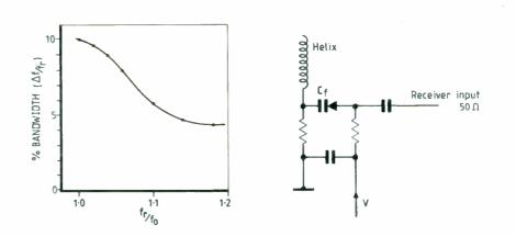
Variation of bandwidth with tuned frequency for a helical antenna, above its natural resonance.
