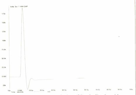
Fig. 4. The transient response of the circuit to a 1V impulse. Note the peak in excess of 175kV – try seeing that on an oscilloscope!
