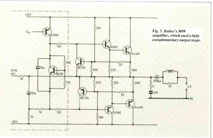
rather more fragile than their nominal n-p-n equivalents, which prompted Bailey to evolve an effective overload protection circuit, also shown in the diagram.
