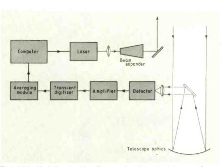
Typical lidar block diagram. Aircraft mounted versions extend the scope of upper atmosphere research. NASA plans a satellite mounted Doppler lidar for wind speed measurement.
