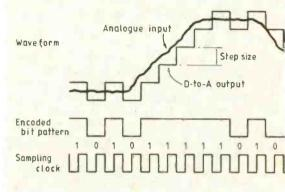
The TMS3477 uses a CVSD (continuously variable slope detection) conversion technique for digitising speech.
