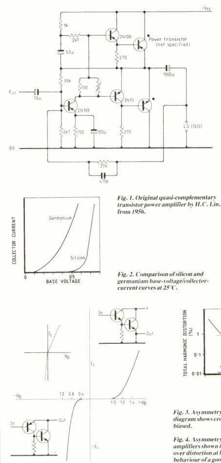
ear. In addition, the reduced gain at the point at which the signal waveform crossed the zero axis tended to suppress low-level signal components and give the amplifier a "thin" sound, lacking in "warmth" and "richness".
