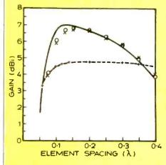
Fig. 1. Effect of reflector-to-radiator spacing according to Lawson (solid line), Mininec (rings), Viezbicke (plus signs, +) and Pozar (crosses, ×).
