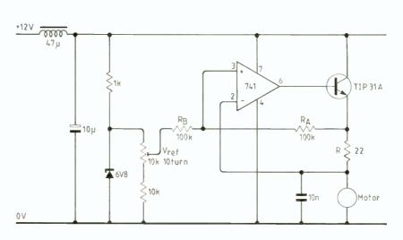
op-amp's input, the same voltage is dropped across R<sub>A</sub>. Current through the resistor flows through R<sub>B</sub> which has the same value as R<sub>A</sub>, so the voltage at the bottom of  $R_B$  must be the same as the voltage applied to the motor. Since this voltage can be controlled by the Cambridge
