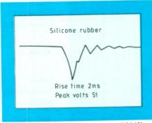
Fig. 2. Voltage output from the PVdF cable on the impact of a steel ball.
