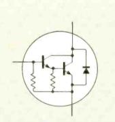
Fig. 10. Internal structure of n-p-n Darlington transistor.
