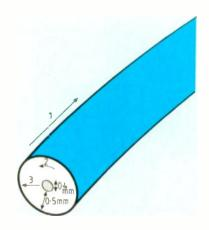
Fig. 1. Dimensions of the Vibetek-20 cable. Stress (for example, a mechanical stress in the so-called 1-direction, along the cable) results in a charge or electric field in the radial direction, the 3direction.
