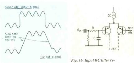
Fig. 15. Effect of slew-rate limiting. stricts rate of input voltage change to that of rest of circuitry.
