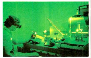
A frequency doubled YAG laser probes the upper reaches of the atmosphere with the optical equivalent of radar. These new instruments are revealing secrets about high altitude haze layers, significant contributors to the greenhouse effect. Page 1057.
