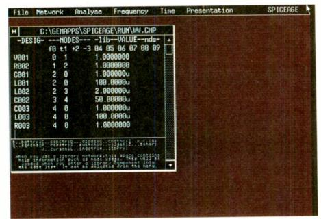
Fig. 1. A simple passive band-pass filter circuit, as entered into Spice.age.
