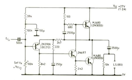
per and lower halves of the output pair, as shown in Fig. 7(a). Because the output transistors can then be of identical type (and  $F_t$ ), the worsening of THD with increase in frequency can be lessened.
