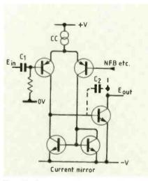
Fig. 13. Current mirror presents high dynamic-impedance load.
