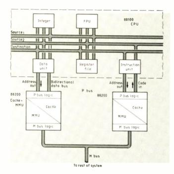
In Motorola's M88000 risc family, the 88100 CPU talks to the rest of the world through the P-Bus Harvard architecture.
