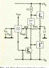
Fig. 11. Use of symmetrical supplies avoids need for blocking capacitor.
