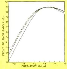
Fig.3. Front-to-back radio of the Yagi-Uda array: Lawson (solid line), Mininec (broken line) and Pozar (dots and dashes).
