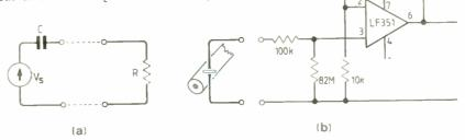
Fig.3. Sensor model (a) and a possible preamplifier design (b).
