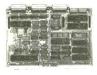
An 80188 target board with 256k bytes EPROM, 256k bytes battery backed RAM, 256k bytes D-RAM, two serial ports, three counter-timers, RTC, watchdog timer, optional mains power supply and case.
