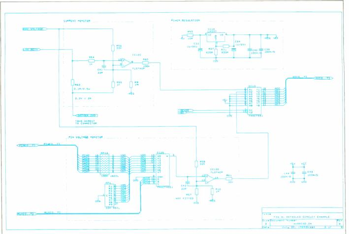
Fig.3. Actual circuitry for the 'connectors and bus decoding' panel, for example, in Fig.2 are detailed separately to avoid cluttering the main worksheet.
