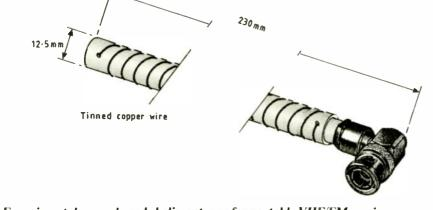
Experimental normal-mode helix antenna for portable VHF/FM receivers (BBC Research).
