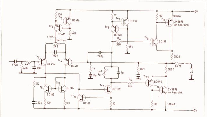
Some temperature compensation for the output transistor forward bias can be obtained from a suitable degree of thermal contact between the output devices and  $Tr_9$ .
