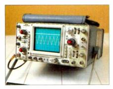
TEKTRONIX 475 200 MHz Dual Beam
