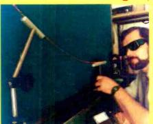
not marvellous compared to the performance of optical fibres at shorter wavelengths, but it should permit a whole new degree of freedom for surgeons using  $CO_2$  lasers. What's more, ERA Technology and Cogent are already predicting considerably improved performance when the waveguide is manufactured using precision machine-drawn fibres. They are at present looking for suitable partners to develop the technology further.
