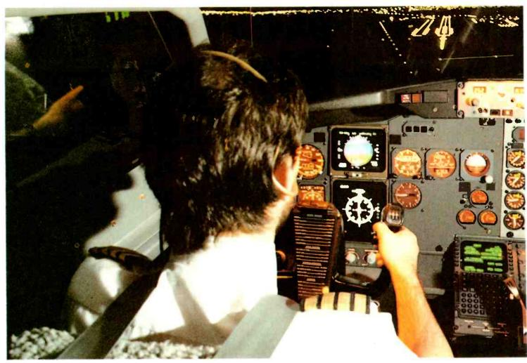
The flight simulator is a device for the instruction and training of aircraft crews. It allows them to carry out operations which might, in a real aeroplane, be dangerous to the aircraft and the crew. The financial aspect is important, in that there are considerable savings in flying time, fuel and wear and tear; the use of revenue-earning aircraft for training is also reduced. It has been estimated that the cost of training using aircraft can be up to ten times that of simulator training.
