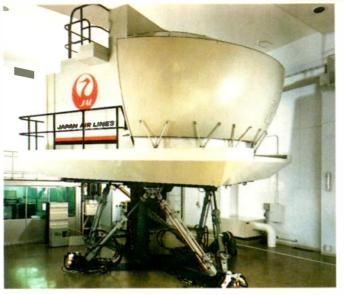
Simulator by Rediffusion Simulation for JAL, showing the curved, wrap-around screen for the WIDE image display. The jacks impart the motion sensation.
