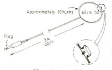
3. resistor, ends of flex tied and resistor soldered between
