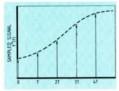
Fig.6. Modelling the sampled signals as a train of weighted impulses. Suppose the signal to be sampled is represented by the dotted lines. Provided that the samples are of infinitely short duration, the sampled signal can be modelled as a train of weighted impulse functions depicted by the vertical arrows.
