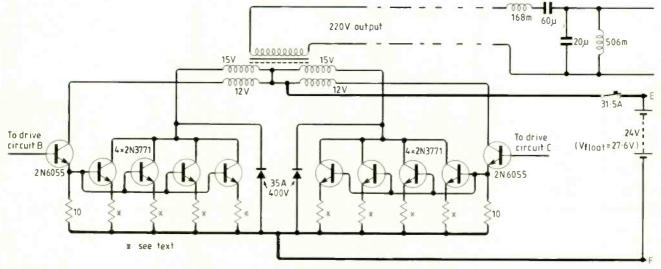
Fig.1. The inverter circuit. Winding information is given in Table 1, with filter choke details in Tables 2 and 3.
