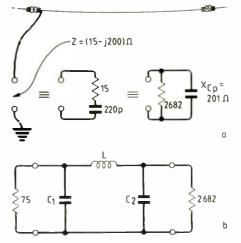
Fig.9. This shows a typical application. In (a) a non-resonant aerial and its terminal equivalent circuit is converted to the parallel form by the transformation. A  $\pi$  network then matches it to 75 $\Omega$ .
