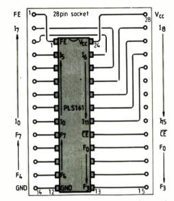
Device types other than the PLS100/101 can be programmed by making modifications. With minor software modifications, using a piggy-back socket like the one shown here allows 24-pin PLS161 p.I.as and PLS162/3 address decoders to be programmed.
