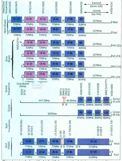
Above: transponder layout for Intelsat VI, the consortium's high-capacity satellite.
