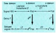
Fig.4. The t, s and z domain representation of delayed signals.
