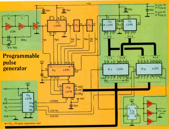
A few t.t.l. devices provide a softwareprogrammable pulse generator for Apple IIe computers. Both the pulse's mark/space ratio and frequency are programmable.
