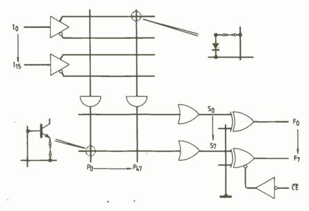
Fig. 1. Logic-equivalent path of the fuse-programmable logic array.
