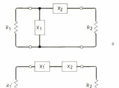
Fig.4. The transformation of the L circuit shown here employs the series-to-parallel conversion, which simplifies calculations considerably.
