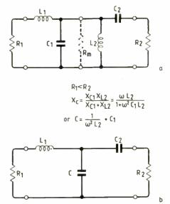
Fig.7. By making a kind of 'hybrid' with the Ls. as in (a), assymetrical T-networks, such as the lossy L shown in (b) can be obtained.
