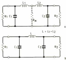
Fig.8. By turning round the L-networks, the  $\pi$  circuits result, as seen here in (a) which forms the low-pass  $\pi$  type matching network.
