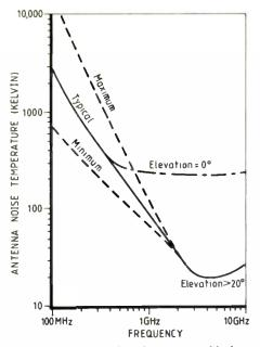
Fig. 2. Antenna noise decreases with frequency, falling to a minimum at about 5GHz.
