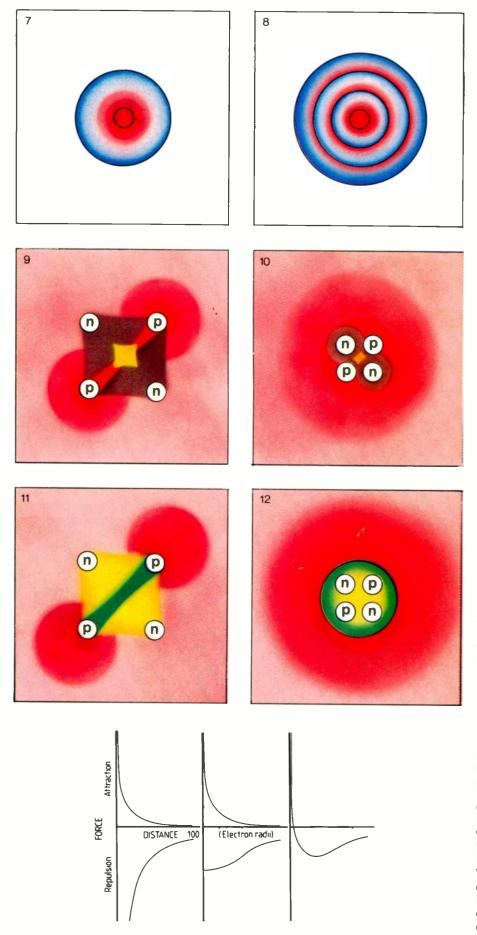
Fig.1. Conventional and modern views of forces in the atom. The graph at (a) shows the traditional "square-law" repulsive force and the attractive interaction above the axis. In the second graph, the repulsive force departs from the square law and is limited, with the result shown in the third graph that the attractive force predominates at nuclear distances to give a stable structure.
