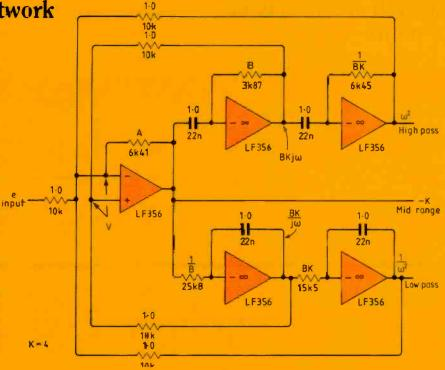
$$\left|T_{L}\right|^{2} = \frac{\frac{1}{\omega^{4}}}{\frac{1}{\omega^{4}} + K^{2} + \omega^{4}}$$
