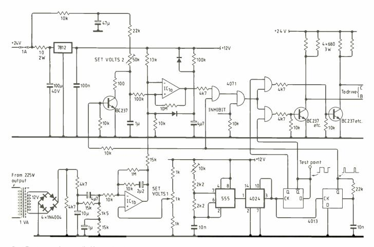
Fig.4 The inverter is controlled by varying the power transistor conduction periods by means of the waveforms at B and C.
