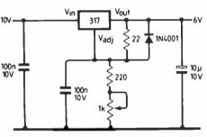
Fig. 4. Regulator i.cs provide some of the voltages needed to program the p.l.d.
