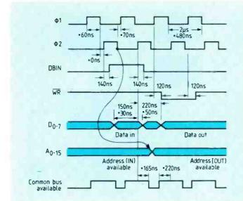
Fig.2. Timing characteristics relevant to connection of an 8080A microprocessor to a common synchronous bus.
