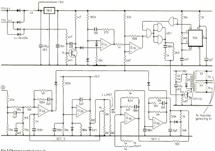
Fig.3 Charger control circuit.
