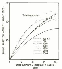
Fig. 6. Image displacement with interchannel intensity ratio in proposed system (-20dB/decade filter).
