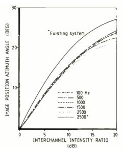
Fig. 5. Image displacements with interchannel intensity ratio in proposed system (60dB/decade filter).
