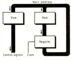
Fig 1. Read-only memory and a register make up the simplest form of microcoded machine.
