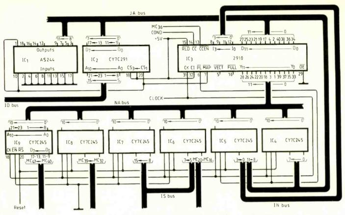
Fig.3. This controller, based on the 2910, is optimized to work with the a.l.u. of Fig.5 to produce a simple 16bit c.p.u.
