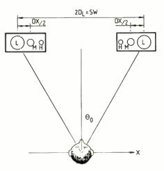
Fig. 2. Geometric arrangement of proposed method of improving image sharpness.  $\theta_0 = 30$  degrees, SW=230 cm.
