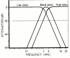
Fig. 4. Filter response characteristics.
