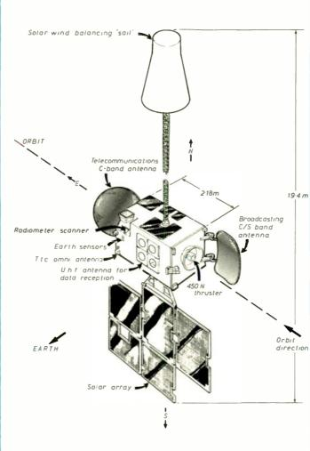
India's second multi-purpose satellite has an asymmetrical structure with a solar array on one side and a balancing solar-wind 'sail' on the other. Diagram shows the orientation of the spacecraft in its geosynchronous orbit, with its antennas facing the Earth (somewhere off the picture to the bottom left). Overall height is 19.4m.
