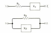
Fig.3. The impedance seen between 1 and 2 in both these circuits is the same, so that transformations can be made between them as desired.
