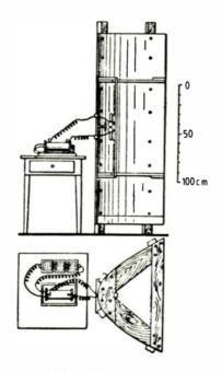
The parabolic reflector arranged on a wooden frame. (After W.F. Magie: A Source Book of Physics, McGraw-Hill, 1935.)
