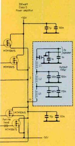
Requirements for a class-D power amplifier are much tighter than those for conventional amplifiers. Output devices must be capable of passing high currents and have an extremely low on resistance. This design, providing 200W continuous power into a  $4\Omega$ load, is one of about 50 designs illustrating the merits of Tmos power fets in Motorola's Tmos power-fet design ideas book. Output of 200W is obtained for a 1.5V
