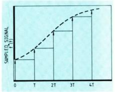
Fig.7. Modelling the sampled signal as a train of weighted pulses. The effect of the a-to-d converter is to take a sample in zero time and to hold this snapshot constant until the next sampling instant occurs one period later.
