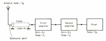
Fig.3. Example receiver system. Individual noise temperatures must be referred to a reference point then they can simply be added together.
