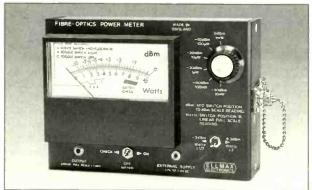
The Ellmax Fibre-Optics Power Meter is an accurate, sensitive, low-cost instrument, incorporating a pointer scale giving readings in both dBm and  $\mu$ W. It measures power levels from 1mW (0dBm) down to below 1nW (-60dBm) at its calibrated wavelength of 820nm, and contains a large area detector in a connector housing. Connector options include SMA and STRATOS. Battery life is typically 500 hours.
