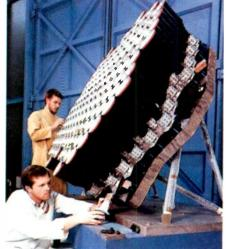
A section of Intelsat VI's antenna feeds. These determine the complex-shaped coverage areas of the satellite's footprint.
