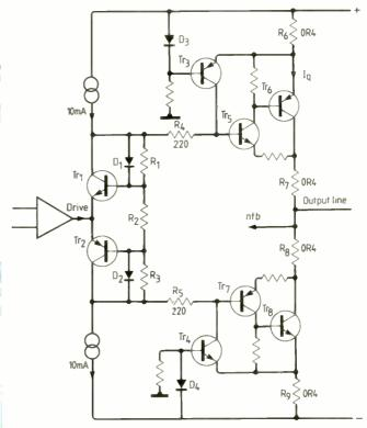
Fig.1. Simplified Blomley amplifier in which  $Tr_{1,2}$  alternately switch on and off but in which  $Tr_{3,4}$  remain conducting due to  $R_3$ . Both circuits feature a fixed voltge-source bias; hence, some part of the circuit must switch if  $I_{out}$  is to exceed  $I_q$ . A true n.s.b. system must include a dynamic variable bias working in opposite direction to the drive, giving bias voltage compliance.
