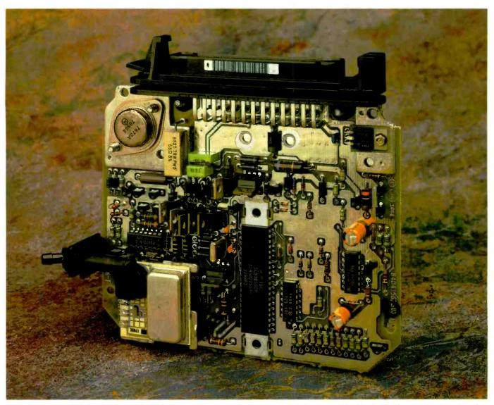
This programmable ignition controller designed for mounting in the engine compartment has an integral pressure sensor and ignition-coil drivers.
