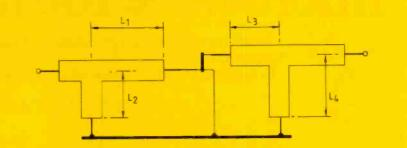
Fig.6. Basic construction of a single-stub matched amplifier.
