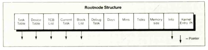
Fig.3. Root-node structure is used by Tripos to keep a record of all aspects of the system. This block is in a fixed position in memory.
