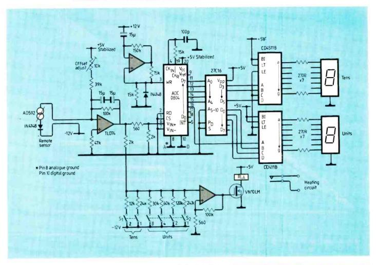
set the temperature and the heating circuit is switched by a relay: the switch comparator provides around 0.5°C hysteresis. Range of the voltmeter is 0-39°C.
