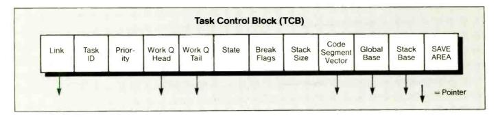
Fig.4. Each task within the system has an associated task-control block containing all information required by the system to manage the task.
