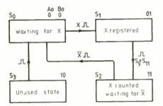
Fig.1 State diagram describes the action of the X register circuit which stores an X pulse by a state change from SO to S1. When the difference counter enters either state S8 or S12 it counts the X pulse by moving to state S9 or S11. The difference counter then clears the X register by moving it from S1 to S2.
