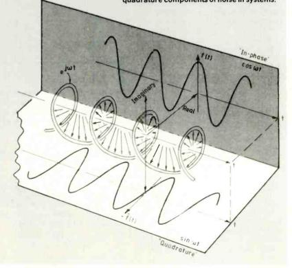
not look on j as a number at all. Instead look on it as operating on a number, like + or does. Operate on +4 with - and the direction of 4 is turned through  $180^{\circ}$  from pointing to the right along the real axis, to pointing along the left, or negative direction.
