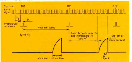
Fig.6. Angle-based ignition with missing tooth reference reduces cost of sensors and eliminates the need for current limit.
