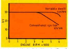
Fig.2. Variable-dwell ignition significantly improves the available ignition potential at higher engine speed and during cranking.
