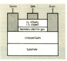
A concentration of electrons induced in the undoped layer of the hemt becomes highly mobile.
