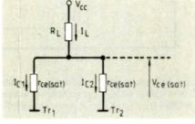
Fig.1. The behaviour of two transistors carrying an overall current  ${\bf I}_{\rm L}$
