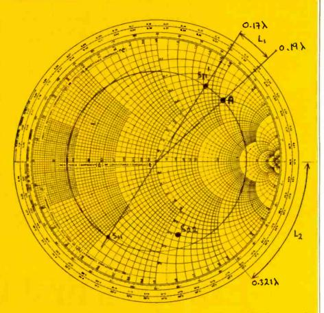
Fig.7. Calculation of a stub matching network. Reflection coefficients of the fet are used to find the required wavelengths.
