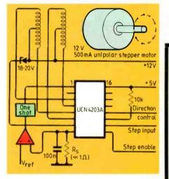
bipolar drivers for 500mA and 2A motors, an a.c. driver for 2A motors and a unipolar two-phase driver for 500mA motors. Brief specifications of fourteen small stepping motors from five North American manufacturers are given.
