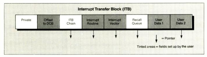
Fig.6. This structure is used by the external interrupt handler to indentify the source of an external interrupt. Each block contains an interrupt routine responsible for servicing a particular kind of interrupt.
