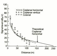
Fig.2. In a stratified medium the relative orientation of the transmit and receive antennas can have a significant effect on the received signal level. Figure 2 shows the signal passing through a near-field/farfield transition as indicated by the change in orientation from coaxial to coplanar horizontal of the loop antennas.
