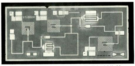
Fig.3. The completed amplifier layout. The gallium arsenide chip is only 1.4 by 3.2mm.
