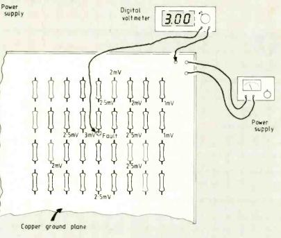
lead resistance has no effect so long as the current source is adequately good and the voltmeter input impedance is sufficiently high. There is no requirement that the lead lengths or resistances be equal in this system. Fig.1(c).
