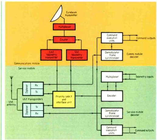
Fig. 1. Spacecraft equipment in the tracking, telemetry and command system used for remote control of the European Communications Satelite.
