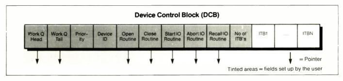
Fig.5. One of these blocks is used for each device in the system. It contains information needed by Tripos to deal with device requests from tasks within the system.
