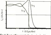
Fig.4. Turn-off currents for two typical transistors
