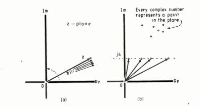
Fig.2. The construction in (a) is called the Argand Diagram. You can think of the arrowed line ('phasor') turning from the 'Re' axis to pointing along the 'Im' axis when operated on by j. All the points on the horizontal line j4 in (b) represent a subset of the complex numbers. In general, the complex numbers describe all the points in the z plane.
