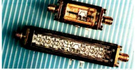
Three cascaded monolithic amplifiers are incorporated in the Thorn EMI 2 to 6 GHz microwave amplifier compared with the much larger amplifier it replaces. Apart from the reduction in size, there is a 30:1 reduction in the number of component bonds required, with a saving in both assembly time and cost.
