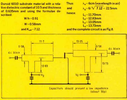
Fig.8. The completed amplifier. The NE72084 fet comes from NEC.
