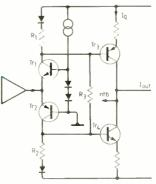
Fig.2. Skeleton circuit of the Margan amplifier. This is very similar to the Blomley design, although the Blomley system does leave each output transistor permanently conducting, while allowing the drivers to switch off.
