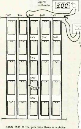
of which way to go. Always follow the increasing voltage as this demonstrates that current is flowing in that direction.
