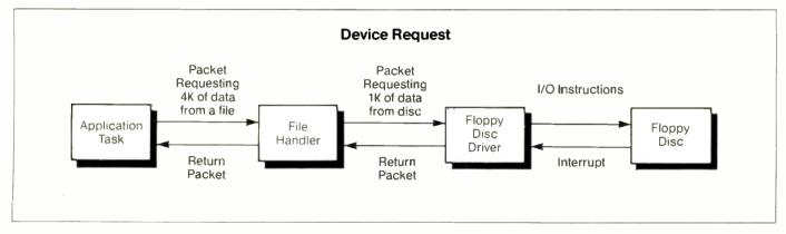
Fig.1. The file handler forms high-level interfacing between the applications task and floppy-disc driver. Low-level interfacing between the file handler and disc is carried out by the disc driver. This technique facilitates device-independent i/o.
