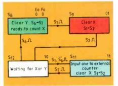
Fig.3. Difference counter counts the first X by moving from state S8 to state S9. When the X register has been cleared, counter is moved to S12 where it waits for either an X or a Y to be stored in the registers. Every X stored before a Y will cause the difference counter to move to S11 producing one difference pulse. A Y will cancel the first X and return difference counter to state S8.
