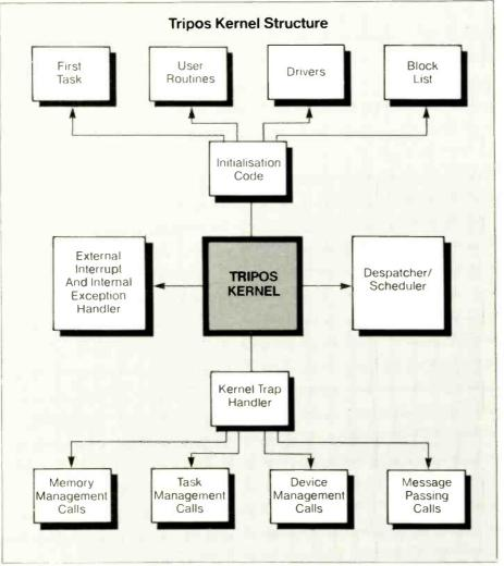
Fig.2. Tripos is structured in concentric layers. These layers become more machine dependent the nearer they are to the centre. Innermost is the kernel, 4Kbyte in size and written in assembly language.
