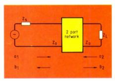
Fig.4. Incident and reflected waves in a transmission line.
