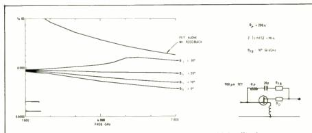
Fig.1. Gain against frequency for a field-effect transistor with feedback.
