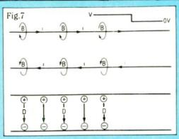
to the right. During this time, extra negative change appears on the surface of the bottom conductor in the next one foot length, to terminate the lines (tubes) of electric flux which now exist between the top (signal) conductor and the bottom conductor.
