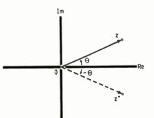
Fig.3. The complex conjugate is the mirror image of the original complex number reflected in the real axis.
