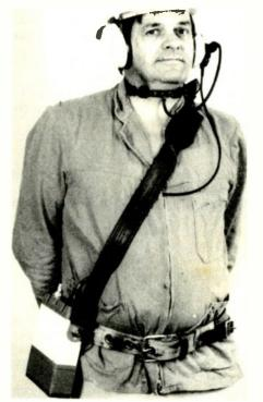
Fig.6. The most recent s.s.b. mediumfrequency underground radio equipment, using a throat microphone. The unit contains a noise-blanking system.
