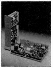
p.c.bs offer auxiliary outpurs of 5, 12, 15, 18, 24 and 48V. 'Power trading' between outputs is a standard feature.
