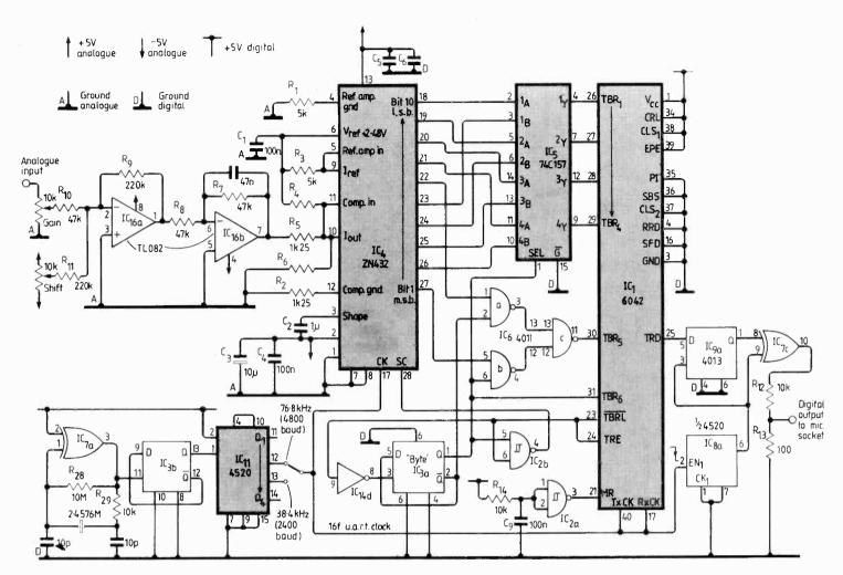
Fig. 1. Record section. Analogue signals are converted into a 10bit digital word and fed to the uart in sections.
