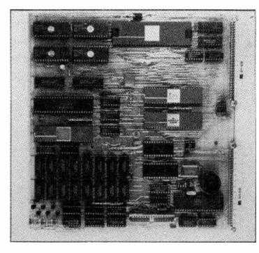
external video source. The board carries 512K of D-RAM plus 128K of system rom and has room for 64K of user rom. An 8M-byte plug-in expansion board with a floating-point co-processor is promised. Also on the way is a Transputer co-processor.
