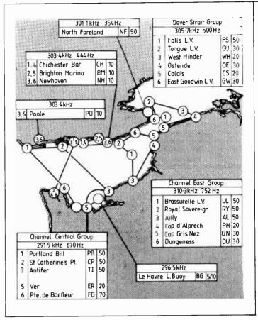
Fig. 2. Radio-beacons covering the English Channel. Most are arranged in groups of six, transmitting in turn on the same frequency. Each table shows the carrier and modulation frequencies of the group and the names, callsings and protected ranges of the individual beacons.
