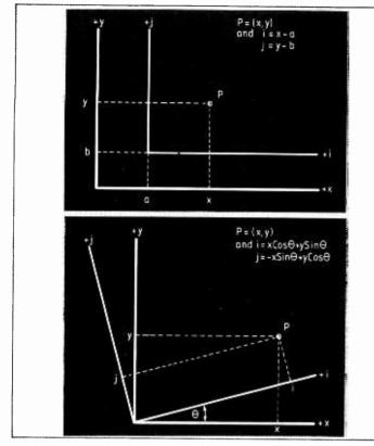
Fig. 2. Translation of (ij) coordinate system (a) and rotation of the (ij) coordinate system (b).
