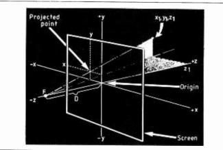
form the same angle at F, they are similar triangles. This means that the ratio of any two sides, is the same for both triangles. So for the point x,y
