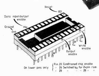
In some ram sockets, mainly in 6502-based computers, the output-enable signal is active during memory writing, which means that SmartWatch cannot be used without hardware modification. Next month we'll show such a modification and a SmartWatch control program for the BBC microcomputer.
