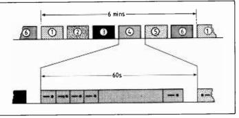
Fig. 4. Transmission sequence of a group of six radio-beacons. Transmissions start on each minute of the clock and are identified by callsigns transmitted in Morse code.
