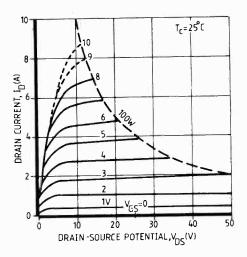
**Fig. 3.** Typical I<sub>D</sub>-V<sub>Ds</sub> curves for 2SK134 show that maximum drain current is limited to seven amps.
