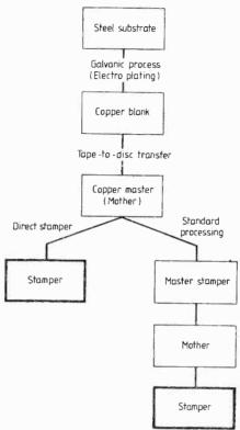
In contrast to lacquer masters, numerous matrices can be produced from a direct metal master, permitting easy correction of defects which may appear in the plating steps en route to the stamper. Process gives a significant time economy in the plating process, especially when making a stamper directly.
