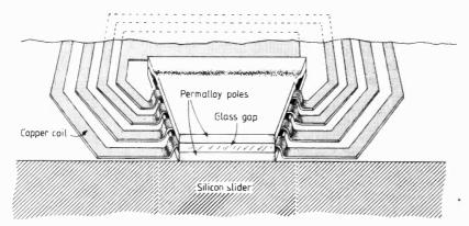
Fig. 1. Thin-film head made using microcircuit technology on a silicon substrate which becomes the slider.
