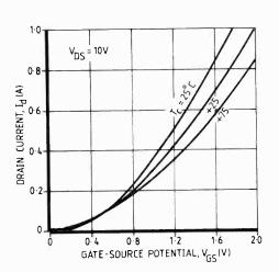
**Fig. 1.** Negative temperature coefficient of the drain current above 100mA prevents thermal runaway with Hitachi 2SK134/2SJ48 type mosfets and avoids use of temperature-tracking circuits.
