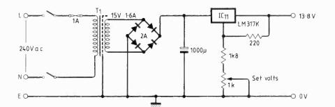
Fig. 4. Power supply, which also charges external battery.
