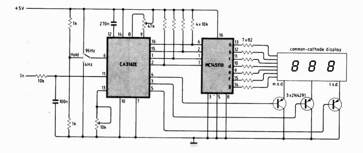
MC14511B is not able to display the "-" (minus) and the "E" (overload) characters. With negative input signals the most significant digit will be blanked, and with overrange input signals all digits will be blanked. Francisco J. Herrero
