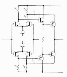
**Fig. 6.** This offers very good linearity and easy control of the second stage current,  $I_2$ .
