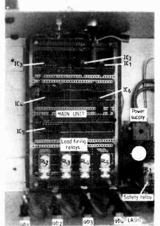
Fig. 5. Main unit construction, on Veroboard, IC<sub>1</sub> and IC<sub>2</sub> are opto-isolators.
