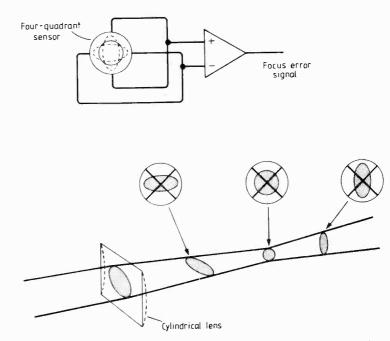
**Fig. 6.** Use of a cylindrical lens prevents a point focus and results in an elliptical image, circular at one point only. Horizontal ellipse causes more light to fall on left and right sensor quadrants, vertical ellipse favours upper and lower quadrants, and a differential amplifier provides focus error signal. Four quadrants are summed for read signal output.
