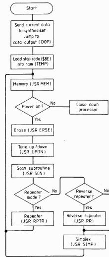
Transceiver software breaks down into these main routines. Mnenonics shown are used in the assembly-language program.
