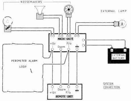
switches to the output contacts of a motion detector or light beam device. All switches must be wired in series.
