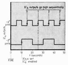
Fig. 2. Counter IC4 timing diagram, showing 20s delay after FIRE input.
