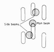
**Fig. 8.** Simple tracking system uses two auxiliary beams each side of the reading beam. Track misalignment causes the two side beam signals to change in amplitude differentially.
