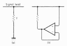
**Fig. 3.** The bootstrap. (a) An unwanted admittance Y shunts the signal lead. (b) The earthy end of Y is driven by the signal at unity gain. Y is still physically present, but no signal current flows through it.
