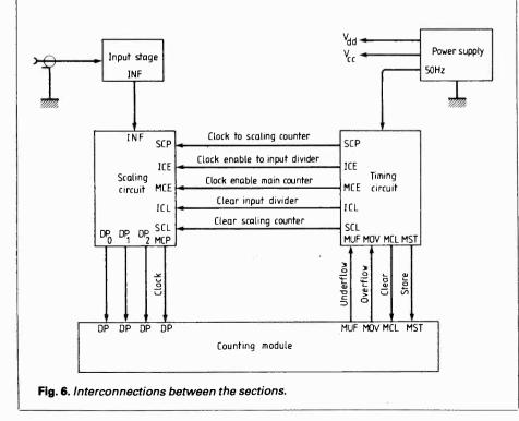
$FF_1$  go high and advances counter IC<sub>9</sub> by one to change the range. As IC<sub>3</sub> is enabled, it can generate the store signal, MST, and the clear signal, MCL. At the same time, through ICL, IC<sub>6,7,8</sub>, both flip-flops and IC<sub>1,2</sub> are all reset and the next count period starts.
