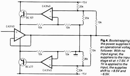
amplifier (surely one only bootstraps passive components?), but the circuit does work as advertised. Indeed, some operational amplifiers have internal bootstrapping of the input stage. If the signal gain from input to supply leads in Fig. 4 is adjusted to be very close to unity, improvements of several orders of magnitude in the input impedance can be obtained. Even ordinary bipolar amplifiers such as the 741 can be given an effective input resistance of many  $G\Omega$ .
