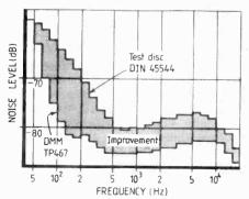
Teldec curves show that new direct metal mastering audibly reduces background noise (measured by third-octave filter). Reference level measurement corresponded to a recorded velocity of 10cm/s for one groove wall. Curve A shows the background noise of rumble test record DIN 45544, and B shows the same measurement with the DMM record TP467.
