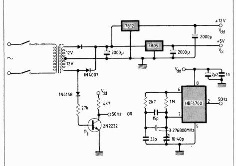
**Fig. 5.** Power supply. Two versions of a 50Hz clock generator are given, one derived from the mains frequency, the other gives quartz crystal precision.
