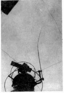
Fig. 12. British Flag. B.1974. Short receiving whip, long co-ax., no impedance matching transformer.
