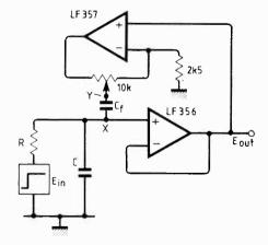
Fig. 5. Capacitance-neutralised voltage follower. R and C are the series resistance and shunt capacitance of the signal source. Signal gain at point Y is adjustable from 1 to 5. The follower stage, here shown as a 356 operational amplifier, is often constructed with bootstrapped supplies as in Fig. 4.
