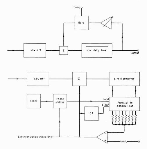
**Fig. 6.** Recirculation loop enhances otherwise noisy output. As data rate is fixed, section of the sequence appears after a fixed time T. The first output is delayed by T so that it reaches the input of the summer at the same time as the next output of the filter arrives. The output of the summer would go on increasing until a threshold is reached, when the gate would open and sync achieved. A t.t.l. version of the recirculation loop is shown at bottom.
