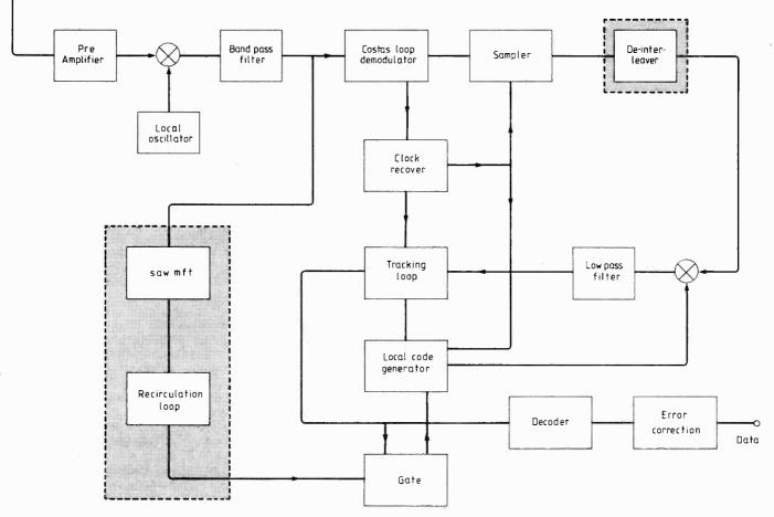
achieve code synchronization so that the local code generator can be synchronized with the received code. As soon as code synchronization is obtained, the tracking loop is switched on and decoding by correlation begins. Further description of acoustic surface-wave matched filters is given later.
