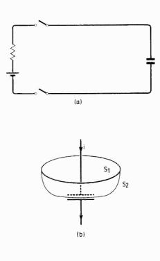
**Fig 1.** The elemental closed loop (a), in which the capacitor creates the difficulty that the current must have two values, depending on whether the surface (b) cuts the conductor or bisects the capacitor.
