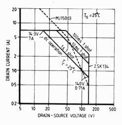
Fig. 4. Compared to a giant bipolar transistor, the mosfet has limited current capability at low voltages, but outperforms the bipolar at combinations of high current and high voltage.
