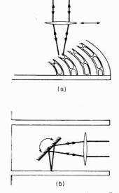
**Fig. 7.** Where space is no problem, fine track-following can be done by lateral lens shift (a). More compact arrangement uses a rocking mirror as shown at (b).
