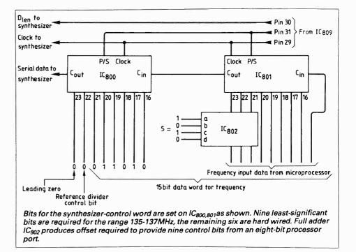
are all that is required to interface the microprocessor to the transceiver, as the circuit diagram shows.
