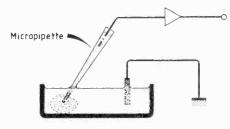
**Fig. 1.** Intracellular recording of potentials from a nerve or muscle cell. The tip of the micropipette is inserted through the cell's membrane. A reference potential is established by an earthed electrode contacting the extracellular electrolyte.
