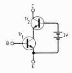
Fig. 7. The cascode configuration is one of the best for large signal handling capability.
