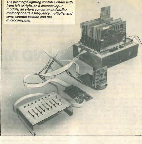
Estimates of the cost of a digital control desk compared with a conventional analogue desk suggest that the former solution is the cheaper alternative for systems with more than 40 channels and 20 master presets. The fixed cost element of the microprocessor system is offset by the absence of a diode-matrix board and the large reduction in the number of faders.
