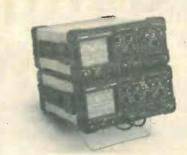
ment can be used as a 35MHz oscilloscope to aid fault location. An IEEE-bus interface is available as an option. Among other new products shown by Philips were two 75MHz lightweight service oscilloscopes, one with a single timebase and the other dual, and an audio-distortion meter for measurements to DIN standards.
