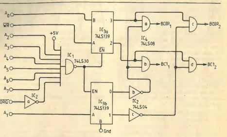
**Fig. 1**. Interface decoding logic for two programmable sound generators.
