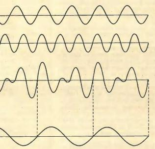
Fig. 2. Schematic method for measuring the autocorrelation function of a signal x(t).
