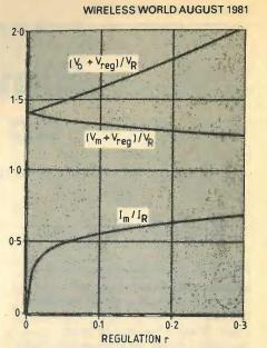
Fig. 3. Graph for a bridge rectifier circuit showing how the maximum available dc current I<sub>m</sub>, the corresponding dc output voltage Vm, and the open circuit dc voltage Vo vary with the regulation of a transformer rated at V<sub>R</sub> and I<sub>R</sub>.
