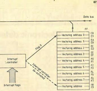
Fig. 6. Basic operation of the 6828 interrupt device.
