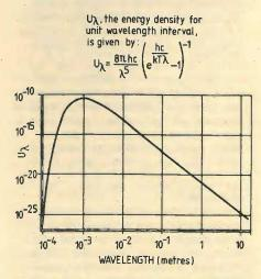
Fig. 2. The black body spectrum for 3K. The units of  $U_{\lambda}$  are joules per cubic metre of wavelength.
