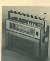
The Fidelity Battery Saver portable radio set which incorporates a battery charger for the dry cell battery.
