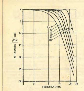
Fig. 9. Amplitude response of the variable low-pass filter. Parameter n is percentage potentiometer rotation
