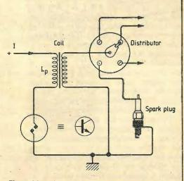
Fig. 2. Many inductive discharge systems simply replace points with transistor
