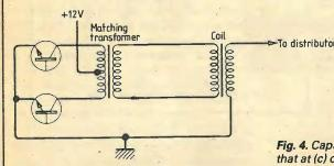
Fig. 3. Bowstock system uses matching transformer and push-pull amplifier to achieve rapid firing rate at full output. (1-coil, 2-transformer)
