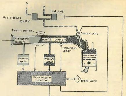
Fig. 5. Basic electronic indirect fuel iniection
