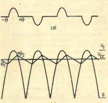
rectifier system. (b) Comparison of |V1cosωt| and VDC when C is infinite. (c) Waveform of current i1 into the capacitor. (d) Waveform of transformer secondary current it. (e) Comparison of /V1coswt/, voltage across a finite capacitance and the dc output voltage.
