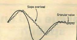
Fig. 10. Slope overload and granular noise in delta modulation.
