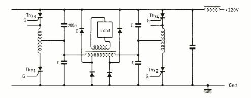
5. Bridge inverter. The commutation transformer may be wound with 28 SWG insulated wire, 130 turns centre-tapped, on a ferrite pot with a 12mm centre core and an outside diameter of 37mm. The power transformer has a 220V primary and a 220V secondary tapped at 10, 110 and 210 watts. The prototype used 30 SWG wire with 5 turns/volt.
