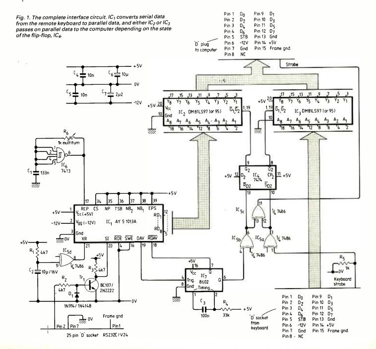
required for connecting the remote keyboard to the interface.
