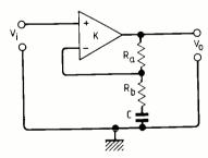
Fig. 1. Basic voltage-controlled voltage source.
