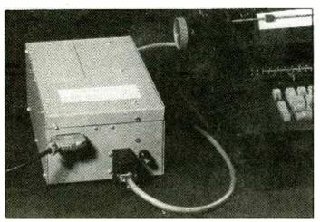
Primary/secondary insulation is tested to 4kV r.m.s. at 50Hz. The price is around £148.50. Technical Selling Services, Unit 5, Brunel Gate, West Portway Indust. Est., Andover, Hants SP10 3SL.
