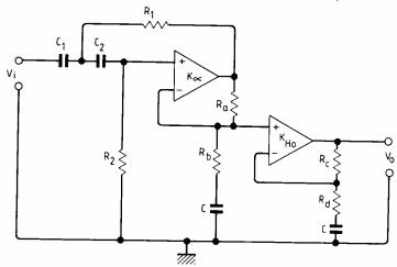
as in the case of the high-pass filter, it is found that, given that  $R_1 = R_2$  and  $C_1 =$  $C_2$ , identical design equations, namely, equations (10) to (12), appear for the three filter parameters. A common set of simplified design equations may therefore be applied to both high-and-low-pass filters.
