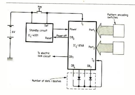
Although the design of a conventional digital lock is reasonably straightforward, a high security device requires around ten i.cs. By using a microprocessor the hardware can be reduced to two i.cs and the flexibility can be enhanced. This design uses a 8748 microprocessor with a 4001 c.m.o.s. i.c. to reduce the standby current. The 8748 is programmed with up to 16 Morse code signals, and these must be repeated serially via a single switch to energise an electric lock.
