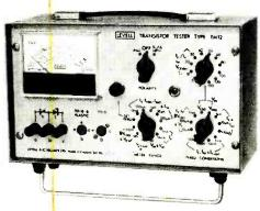
Tests bipolar transistors, diodes and zener diodes. Measures leakage down to 0.5 nA at 2V to 150V. Current gains are checked from  $1\mu A$  to 100mA. Breakdown voltages up to 100V are measured at 10μA, 100μA and 1mA. Collector to emitter saturation voltage is measured at 1mA, 10mA, 30mA and 100mA for  $I_C/I_B$  ratios of 10, 20, 30. The instrument is powered by a 9V battery.
