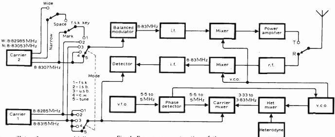
an oscillator, frequency multipliers, to get this frequency up to the transmitter frequency, a modulator, a power amplifier and a tank circuit for aerial matching. In most cases the transmitter stages in amateur equipment use a mix of discrete semiconductors, valves and often i.cs.
