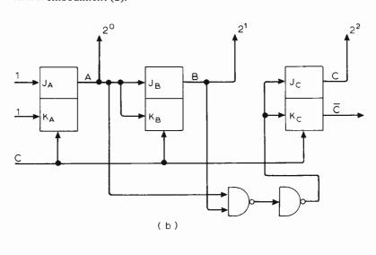
Synchronous 'down' binary counters (maximum length) can be designed in precisely the same manner and the following flip-flop equations are obtained.
