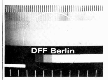
East Germany DDR-F (B, G) SECAM colour — Alternative identification used with the DDR-F electronic test card.
