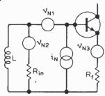
where  $v_{N1}$  is the equivalent noise voltage generator of the transistor,  $v_{N2}$  the equivalent noise voltage generator of the input resistance  $R_{\rm in}$ ,  $v_{N3}$  the equivalent noise voltage generator of the equivalent feedback network resistance  $R_{\rm f}$ ,  $i_{\rm N}$  the equivalent noise current generator of the transistor, and L the inductance of the magnetic cartridge, assumed purely inductive.
