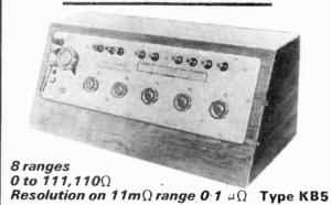
For low resistance measurement with Electronic Null Detector
