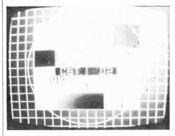
Czechoslovakia CST (D, K) SECAM colour — The FUBK electronic test card is used as an alternative to the PM5544.
