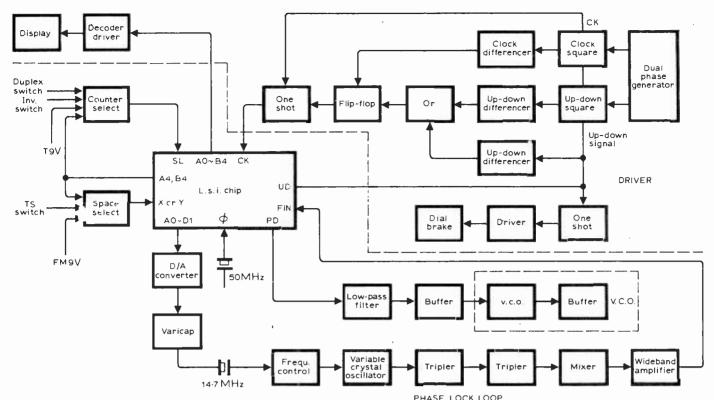
from the clock at CK. Inputs X or Y at 'space select' determine whether the counters are updated in 5kHz or 100Hz steps, and these are selected by the speed switch TS on the front panel of the transceiver.
