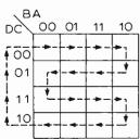
Fig. 1. Karnaugh plots of reflected binary (a) and Gray code (b). Tabulation of Gray code is at (c).
