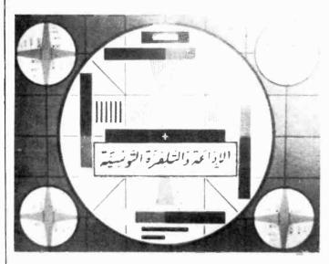
**Tunisia RTT (B) SECAM colour** — Radiodiffusion-Télévision Tunisienne has ten main transmitters, all of which operate in Band 3.
