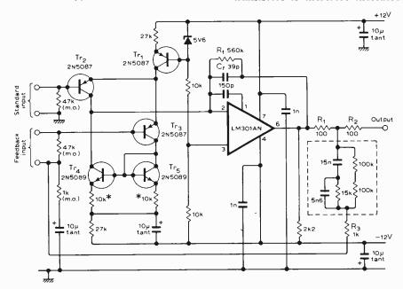
and at this point the use of an operational amplifier becomes attractive in terms of cost and performance. An integrated circuit operational amplifier with shunt feedback and the output stage operating in class A is used in the present design, the advantages of this arrangement being
