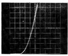
Fig. 12. (a) Superimposed transconductance traces for: (i)  $V_{\rm DG}=0;~V_{\rm BS}=0;~(ii)~V_{\rm GS}=0,~V_{\rm BG}=0~(b)$  Device in forward connection with  $V_{\rm BS}=0~({\rm left})~{\rm and}~V_{\rm BS}=-12V~({\rm right})$  Scales for both photographs: vertical 0.2mA/cm, horizontal 1V/cm
