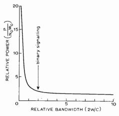
Fig. 2. Actual noise power is usually proportional to bandwidth.  $N_o=$  noise power per hertz;  $W_o=$  bandwidth needed for communicating C bits/s by binary signalling. With bandwidth W and rate C the relative bandwidth is represented by 2W/C.
