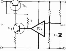
Fig. 3. Further improvement to introduce extra gain and improve line and load current regulation.
