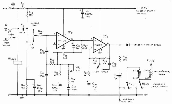
lift time constants are determined by  $C_{12}$  and  $C_{15}$ .
