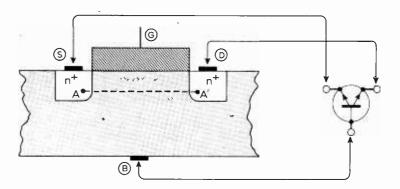
Fig. 9. Showing the existence of an inherent lateral n.p.n. transistor
