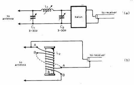
Fig. 4. Impedance matching unit (a) requires a balun (b) for receivers with unbalanced input circuits.  $L_1$  is 5 to 10 turns on a 0.25in dia. former about 0.3in long.  $L_2$  is 10 turns of close-wound bifilar wire on 0.25in dia. former wire gauge can be around 28-30 s.w.g.
