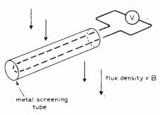
V will be small for fast B changes for an unbonded screening tube since skin effect prevents currents and flux penetrating the tube, hence within the tube  $d\Phi/dt \rightarrow 0$ .
