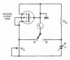
Fig. 10. Test circuit for determination of model parameters
