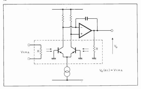
heat to each is equal. Any unbalance is amplified by the operational amplifier forcing the direct output voltage to deliver the same power to the right-hand resistor as the input delivers to the other. Hence the r.m.s. values of the two voltages are equal. A neat idea, though one that requires a very carefully constructed chip if the sensing transistors are each to respond to only one of the heat sources.
