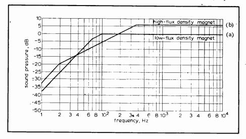
Fig. 2. Schematic curves of effect of flux on axial frequency response of a loudspeaker unit in a closed cabinet: (a) normal flux, (b) twice the flux.
