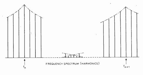
Fig. 3. Part of the spectrum of a typical television signal, showing the n<sup>th</sup> and  $(n+1)^{th}$  harmonics of line frequency. Each of these is accompanied by "sidebands" corresponding to field frequency and these overlap halfway between line harmonics.
