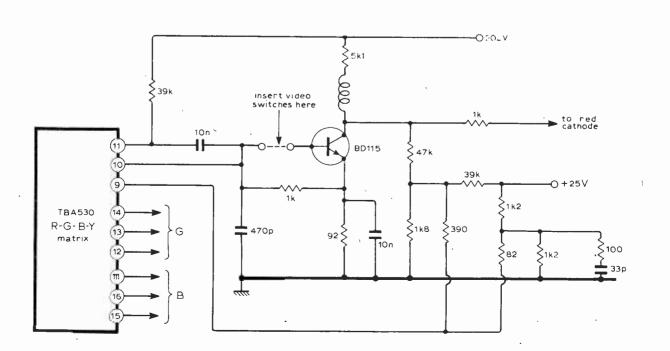
should be noted that the polarity of these and the input electrolytics will depend on the individual receiver design and may not be as shown.) Figure 1 shows a fourth pair of switches which are not required when modifying a receiver of the type described. They are useful, however, when modifying a set which has colour-difference amplifiers (R-Y, G-Y and B-Y), as they can be used to switch off the luminance signal, which would otherwise be present while watching the Teletext display.
