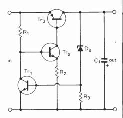
Fig. 5. Practical design of the regulator circuit.
