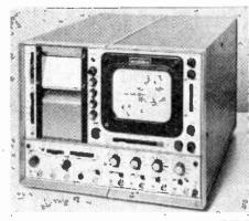
Four-channel recording oscilloscope, the FOR-4 produced by Medelec, can be used as a strip chart recorder, an X-Y plotter or as an alternative to a conventional oscilloscope. A modified version to be shown for the first time includes an automatic repriming circuit which operates in the single shot mode to allow the recording of random transients.
