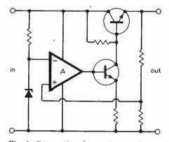
Fig. 1. Conventional transistor voltage regulator.
