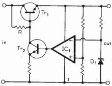
Fig. 2. General design of a feedback controlled regulator.
