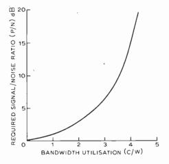
Fig. 1. Required signal  $\bar{l}$  noise ratio, P/N, as a function of bandwidth utilisation: C/W = bits/s per hertz of bandwidth.
