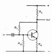
Fig. 6. Stabilising circuit based on a combination of the circuits of Figs. 3 (a) and (b).
