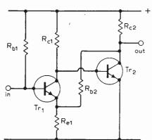
Fig. 10. This alteration to the position of  $R_{b2}$  makes little effect on the performance of the circuit.
