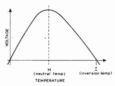
Fig. 7. General temperature versus voltage graph for a thermocouple.
