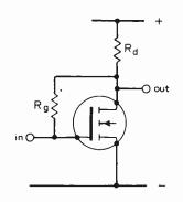
Fig. 13. Basic circuit for d.c. stabilisation of an enhancement type f.e.t.
