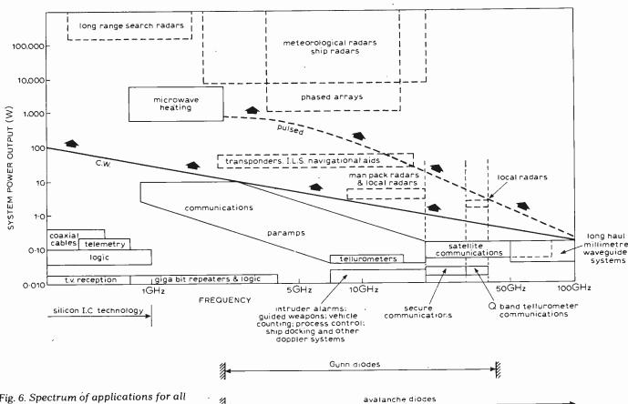
Fig. 6. Spectrum of applications for all solid-state microwave systems.
