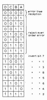
A,B,C & D are parity checks over the following bit no's
