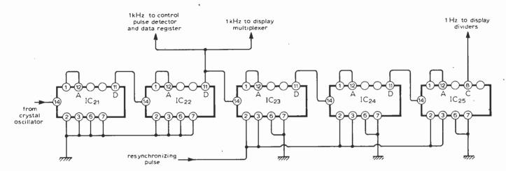
Fig. 3. (top) Display dividers — seconds, minutes and hours each use decade counters and the tens of seconds and minutes use divide-by-12s.
