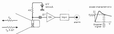
Fig. 8. Self-oscillating mixer alarm system. Due to a higher noise level and small signal from a moving object the circuit is only suitable for up to 10m.
