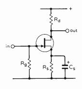
Fig. 15. Method of biasing and d.c. stabilising a depletion-type f.e.t.
