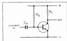
Fig. 1. Basic common-emitter amplifier. This circuit (and Fig. 2) have a number of serious disadvantages discussed in the text.
