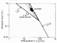
Fig. 4. Idealized plot of power output versus output frequency. The position of the  $1/f^2$  line is controlled by the material properties of the semiconductor used.
