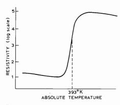
Fig. 3. Resistivity versus temperature graph for barium titanate.
