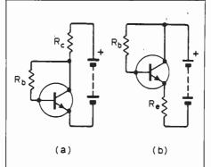
Fig. 3. Two fundamental methods of applying negative feedback to a bipolar transistor.
