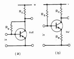
Fig. 8. A video amplifier based on the circuit of Fig. 7 (b).
