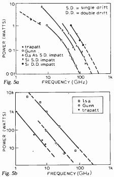
Fig. 5. Limiting plots of power versus frequency for (a) c.w. and (b) pulsed generation using current techniques and devices.
