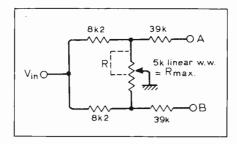
The calculated error for the circuit is less than 1dB over the full range of the potentiometer. The input impedance, about  $5k\Omega$ , is constant within 10% over the same range  $A_{max}=0.35V_{in}$ .
