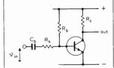
Fig. 2. The inclusion of the series resistor  $R_s$  enables the basic circuit to be used with a voltage input.
