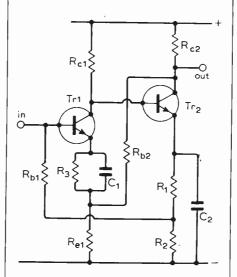
Fig. 11. Final form of the circuit of the two-stage voltage amplifier.
