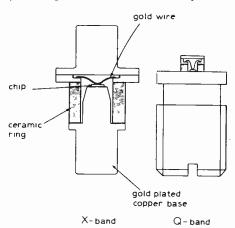
Fig. 3. Final packages for an IMPATT diode. These packages are similar for Gunn devices.
