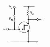
Fig. 12. Simplest type of f.e.t. amplifier which has a number of disadvantages.
