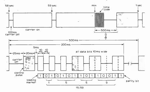
before it is allowed to influence either internal timing or displayed time. The transmission is normally maintained twenty four hours a day, except for five or six hours on the first Tuesday of each month to allow for maintenance. The clock will free-run during this period and the accumulated error (a fraction of a second) will be eliminated when the code is again received.
