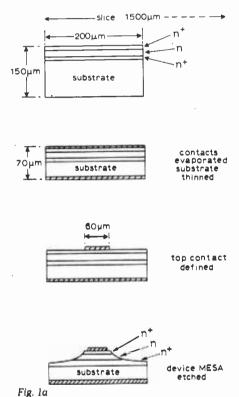
Fig. 1(a). Fabrication of a typical low power 20mW c.w. device. Scanning electron microscope photograph of such a device is shown at (b).
