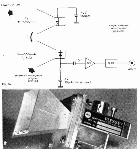
Fig. 7(a). Gunn diode intruder alarm system using a separate detector. (b) Typical transmit/receive module'- normally used for ranges from 10 to 100m.
