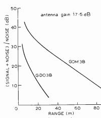
Fig. 9. (Signal + noise) / noise versus. range of a self-oscillating mixer system and a separate-detector type using a man as the target, and the circuits used to obtain the range data.
