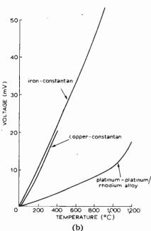
Fig. 6(a)(b). Difference-voltages developed by several common types of thermocouples for two different temperature ranges.
