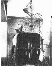
Intelsat IV-A communication satellite (see news item). British Aircraft Corporation Electronic & Space Systems Group at Bristol under contract to Hughes Aircraft Company manufactured major sections of the satellite including the spun structure, booster adapter, despun components, cable harness and solar arrays.
