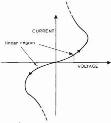
Fig. 5. Approximate current versus voltage characteristic for an n.t.c. thermistor heated by its own power dissipation.
