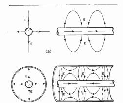
Fig. 1 Circularly symmetrical  $E_{\rm o}$  waves (a)  $E_{\rm o}$  surface-wave supported by a single conductor isolated in space. This is a slow-wave. (b)  $E_{\rm o}$  wave between coaxial metal surfaces. This is also a slow-wave and can be regarded as a form of dual surface-wave.
