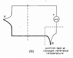
Fig. 9 (a). Simple thermocouple thermometer and a superior arrangement (b) where a second thermocouple is held at a constant reference temperature.
