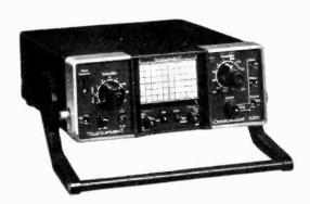
The S22 is a single trace 5MHz scope with an additional high sensitivity (1mV) facility, and offers automatic selection of TV line or frame displays. It is battery or mains operated. The internal batteries are rechargeable.
