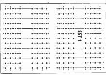
When your circuit is proved working on your DEC, simply plug the components into a Super Solder Board — a fibre-glass, drilled, roller-tinned finished circuit board using the same layout as the DEC breadboard. Once the components are plugged in, in the same positions as on the DEC, solder! (No cutting or drilling of contact rails.) The result — a perfect, finished, printed circuit board.
