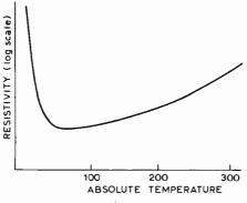
Fig. 2. Resistivity versus temperature graph for extrinsic silicon.
