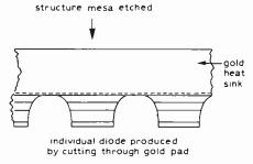
Fig. 2. Integral heat sink fabrication for an IMPATT diode. The active region of the device is adjacent to the metal heat sink for good thermal conductivity.
