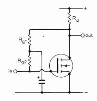
Fig. 14. Method of eliminating signal-frequency feedback in the circuit of Fig. 13.
