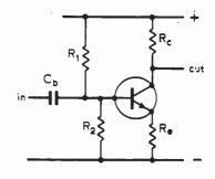
Fig. 5. Method of d.c. stabilising a transistor by a potential divider and emitter resistor.
