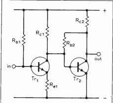
Fig. 9. Basic form of two-stage direct-coupled voltage amplifier.
