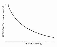
Fig. 4. Resistivity versus temperature for an intrinsic semiconductor material showing an approximate inverse-exponential curve.
