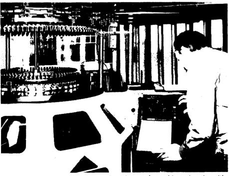
Vernon H. Cooper Ltd's new yarn speed monitor can be used in conjunction with all types of knitting machines, both circular and flat and having varied rates of feed. The monitor incorporates EMI's electronic fabric control system.
