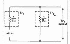
Fig.15. Essential features of the circuit of Fig.14 with S closed and for the left-hand signal.
