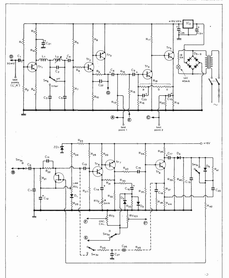
Fig. 12. Circuit of one channel of the stereo Dolby B noise reduction unit. Upper circuit is of main signal path, input at D, output at C. Point G feeds meter circuits of Fig. 15, while point A or point C feeds the side-path input B (bottom), according to whether encode
