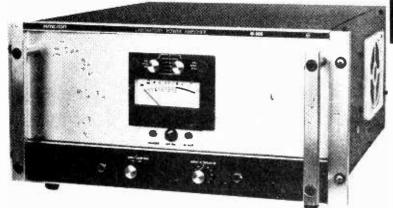
Coupling two M600s together through a socket provided at the back of each amplifier produces a 140 Volt balanced output. This configuration is called an M2000, and produces 2 kilowatts into an 80hm load. A peak catching meter, and threshold lights provide convenient front panel output monitoring
