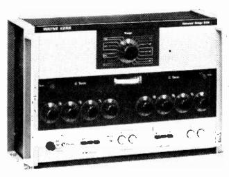
The B224 is a manually operated bridge, the resistive and reactive terms being independently set to a null indicated on the meter. A rechargeable battery is fitted in order to make the instrument portable.
