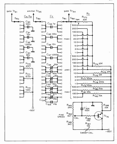
Fig. 8. Sweep-time selector switch and fine sweep-time control.  $C_H$  and  $R_H$  are hold-off components to allow  $C_T$  time to discharge.
