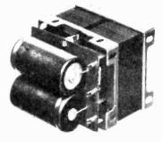
The PSU50 incorporated a specially designed transformer and can be used for either mono or stereo systems.
