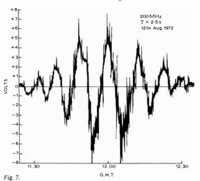
detectable signal is proportional to 1/bandwidth × time constant. Since the bandwidth is constant at about 8MHz, several time constants were available at 0.5 secs., 2.5 secs. and 80 secs. This latter gave very smooth traces but the loss of detail was considerable. In this connection, very good quality paper dielectric capacitors must be used, or leakage will give an unknown time constant. The signal now passes to a d.c. amplifier and thence to the pen recorder.
