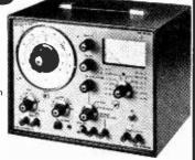
**DM344A Distortion Factor Meter.** Designed to make accurate and rapid measurements of total harmonic distortion generated within high quality audio amplifiers, recording and transmission equipment. **Selling Price:** c/w Bench Case £175.00 + VAT.
