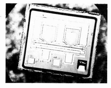
Development microwave f.e.t. from NEC showing ½ micron channel.
