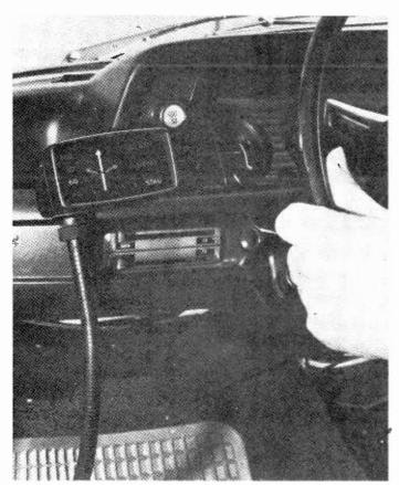
Fig. 2. Announcement display in the vehicle. This has arrows to give directions, warnings of road conditions and recommended speeds.
