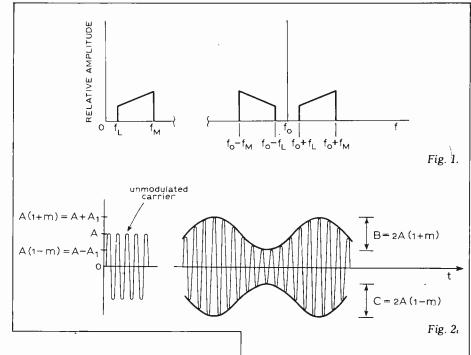
methods of producing amplitude modulation.
