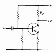
Fig.5. A load resistor  $R_{\rm c}$  connected directly into the collector circuit of a biopolar transistor.
