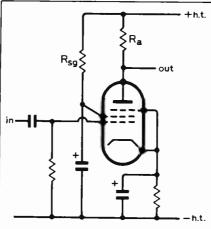
Fig.4. Method of applying positive bias to the screen-grid of a pentode.
