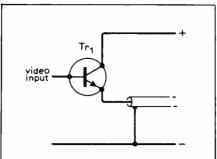
Fig.13. An emitter follower used to feed video signals into a coaxial cable.
