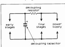
Fig.1. A decoupling resistor.
