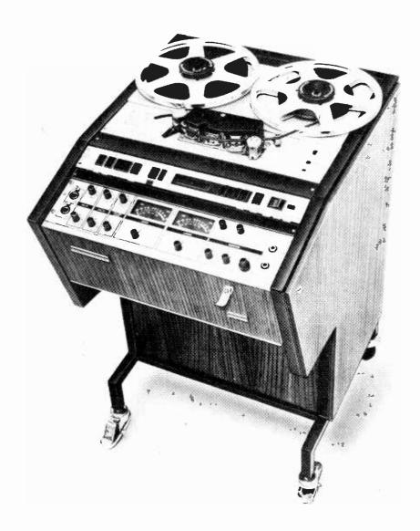
Full logic control. Tape motion sensing. Two speeds. Servo-controlled capstan. Constant tape tension. Direct-reading tape timer (minutes and seconds). Three editing modes. Provision for synchronisation, remote control and remote display panel. Available for line-in/line-out or with mixing and monitoring facilities. IEC or NAB equalisation. Full or
