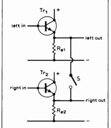
Fig.14. S is a stereo-mono switch which could lead to severe distortion.
