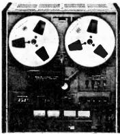
Similar facilities to Teac 3340 . Three motors. heads, solenoid operation, electronic echo Speeds  $7\frac{1}{2}$  and  $3\frac{3}{4}$  i.p.s. 7in. spools. Mic and linemixing
