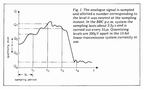
transmitted to represent each level must be increased. Each addition of a binary digit to the word length giving the number signifies a doubling of the number of levels and a reduction in quantizing noise of 6dB. But each addition of a bit to the binary word means an increase in the bandwidth needed to transmit the signal.
