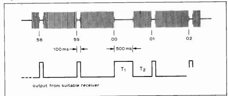
used. The rectified signal is inverted to give output pulses as in Fig. 1, and the bandwidth is made wide enough, together with a suitable gain setting, to ensure that the output follows the "r.f. off" transition to within 1ms. A.g.c. is not incorporated, because the received signal level is fairly constant, and also because an increase in gain when the transmitter is off would increase the sensitivity to noise.
