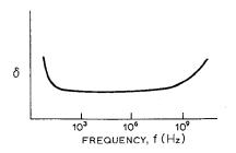
Fig. 9. Loss angle versus frequency for a non-polar dielectric material.
