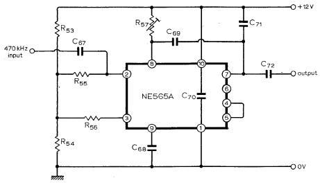
Fig. 19. Practical phase-locked loop circuitry.
