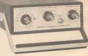
Frequency range of 0.1 Hz to 1 MHz. Sine, square or triangle waveforms. Calibrated attenuation from 0 to 50 dB in 10 dB steps. Output 10 volts peak to peak. Frequency accuracy of ± 3% of full scale on dial.
