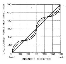
Fig. 4. Perceived localization vs intended direction of sounds in degrees, according to the mid-high frequency theory of this paper, for various systems via a square of speakers as in Fig. 2. Triangles indicate speaker positions. QMX data only applies for a full bandwidth system. Compare with Figs 19 and 20 of reference 26.
