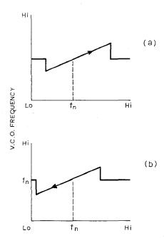
Fig. 18. Asymmetrical locking diagram of the phase-locked loop. (a) reference frequency rising (b) reference frequency falling.
