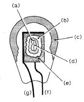
Fig. 13. Schematic of a complete solid tantalum capacitor (a) tantalum impregnated with manganese dioxide (b) graphite layer (c) resin outer coating (d) tantalum shown cut away to indicate anode terminal and tantalum pentoxide layer (e) solder layer completely surrounding cylinder (f) welded anode connection (g) cathode connection.
