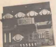
4 R.C.A. 150 watt 15 amp output transistors
