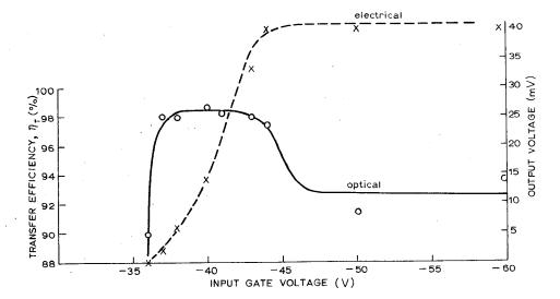
Fig. 10. Variation of optical transfer efficiency with voltage on input gate for an eight-bit p-channel device. Dashed line shows electrical transfer characteristic for the same device.
