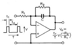
Fig. 5. LM3900 c.d.a. is well-suited to measurement of time period and frequency. An input capacitor can alternatively be charged through a diode to form a "pump" circuit (see card 10).
