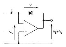
Fig. 6. Defining operating conditions for testing a zener diode with a c.d.a. (see card 5).
