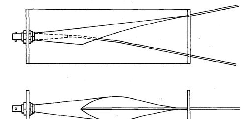
Fig. 5. Coaxial to open-wire flare.
