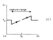
Fig. 16. Phase-locked loop capture range (a) reference frequency rising (b) reference frequency falling (c) resultant capture range. The v.c.o. natural frequency is f<sub>n</sub>.
