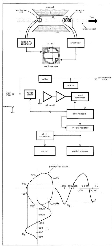
Fig. 3. Schematic arrangement for determining blood flow using nuclear magnetic resonance. The time taken (t) for protons "tipped" at the excitation point to reach the detector coil is used to calculate flow. Typical spacing (d) is 3cm
