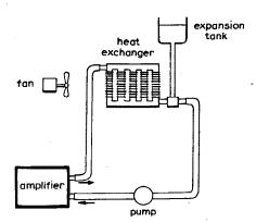
Fig. 2 Complete fluid cooling circuit
