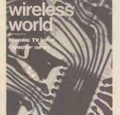
This month's front cover shows part of a printed circuit of Sphericall, a Pye TMC l.s.i. device for push-button telephone dialling.
