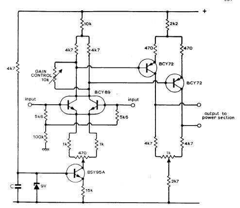
Fig. 7 Preamplifier circuit.
