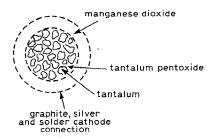
Fig. 12. Solid tantalum capacitor slug formed by sintering tantalum powder particles around a tantalum anode.
