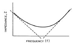
Fig. 3. Impedance versus frequency curve of the simple resonant circuit shown in Fig. 2.
