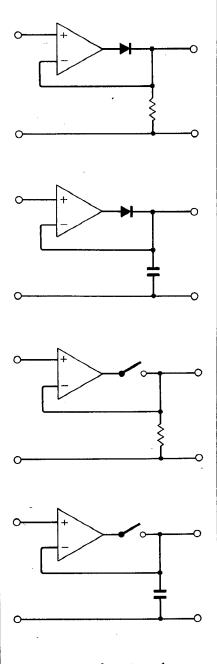
Figs. 1–4. Types of circuit used to measure amplitude of a.c. waveforms (see Table). Complete circuits are given in cards 7 and 8 in set 18.
