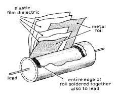
Fig. 16. Constructional features of a plastic film capacitor.
