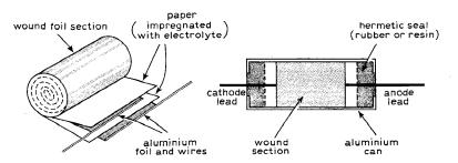
Fig. 11. Construction of an aluminium electrolytic capacitor.
