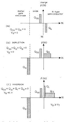
Fig. 9. Schematic diagram of the charge distribution in an m.o.s. structure for three cases: (a) zero volts on the gate, (b) depletion, and (c) inversion.
