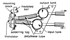
Fig. 1 Mechanical layout of liquid-cooled power output stage
