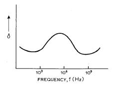
Fig. 8. Loss angle versus frequency for a polar dielectric material.
