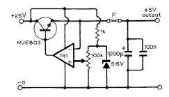
Fig. 12. Circuit of high-current 5V regulator for on-card use.
