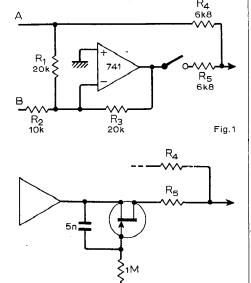
and  $R_4$  (assuming source impedance at input  $A \ll 6.8 k\Omega$ . The degree of attenuation of the unselected input depends on the tolerances of  $R_1$ ,  $R_3$ ,  $R_4$  and  $R_5$ , and if more than about 30dB rejection is required, some trimming may be necessary.
