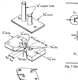
Fig. 4 Dimensions of transistor mountings.
