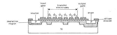
long (in the transfer directions) by  $300\mu m$  wide with a gap between the electrodes of  $2.5\mu m$ .
