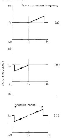
Fig. 17. Tracking range diagram for the p.l.l. (a) reference frequency rising (b) reference frequency falling (c) resultant tracking range.
