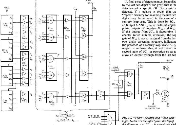
digits screening circuitry, for indication of ordinary leap-year. In either case, whichever gate a signal comes through, it will cause a resultant output of logic 0 since again  $IC_{25}$  is an open-collector type and the common collector resistor  $R_6$  gives wired-OR logic.
