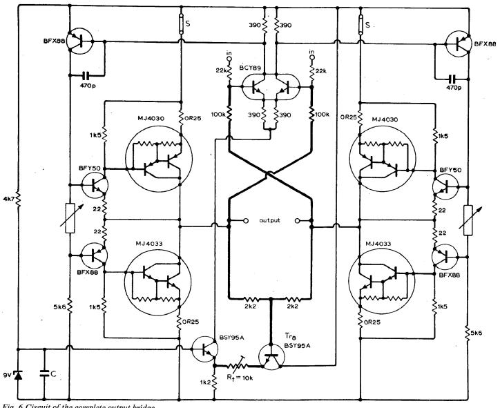
Fig. 6 Circuit of the complete output bridge.
