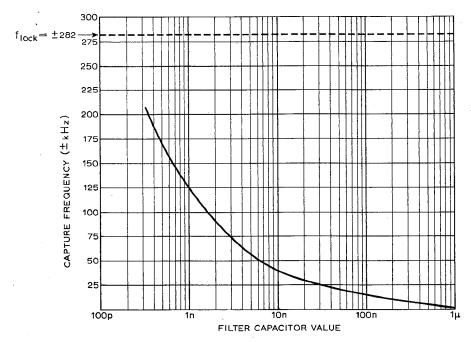
Fig. 20. Capture range versus filter capacitance for 475kHz p.l.l. circuit in Fig. 19. Discriminated output at pin  $7 \approx 100 \text{mV per } 25 \text{kHz shift.}$
