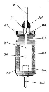
Fig. 14. Schematic of a wet-sintered tantalum capacitor (a) fine silver (b) anodized sintered tantalum anode (c) tantalum wire (d) solder seal (e) tantalum to nickel weld within header (f) nickel wire (g) solder seal between header and external anode lead (h) glass-to-metal seal (j) internal seal (k) electrolyte (l) anode boot (m) cathode.
