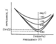
Fig. 4. Impedance curve for a tantalum electrolytic capacitor.
