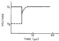
Fig. 15. Process of self healing of a metallized dielectric capacitor. The voltage trace is typical during the process.
