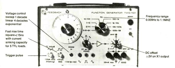
All seven outputs are simultaneously available with amplitudes constant over frequency range
