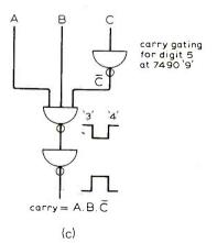
Fig. 2(a). A typical counter, decoder and display, showing the "crossed" connexions between decoder and display. "Carry" to the next decade is enabled by the circuits of (b) and (c) for resets to "0" or "9".
