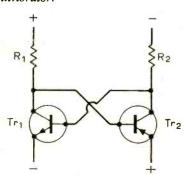
Fig. 6 A redraw of the circuit diagram of Fig. 5: in this form it is clearly a multivibrator.
