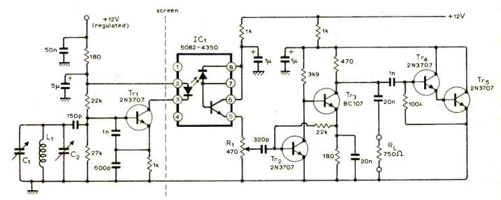
Fig. 1. Oscillator, optically coupled isolator and first stage of amplification.
