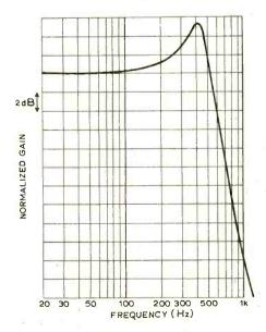
Fig. 8. Peak of appropriate height to compensate dip in Fig. 7 obtains for  $R_2 = 27k\Omega$ , with  $R_1 = 47k\Omega$  in  $IC_2$  circuit.
