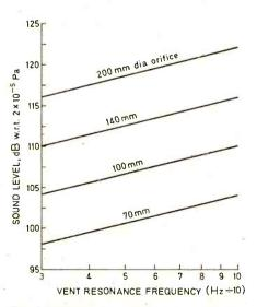
Fig. 3. Minimum programme sound level in room of 2000ft<sup>3</sup> (60m<sup>3</sup>) for various size orifices and vent resonance frequencies before nonlinearity is appreciable from orifice.
