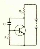
Fig. 13 The Miller integrator circuit.
