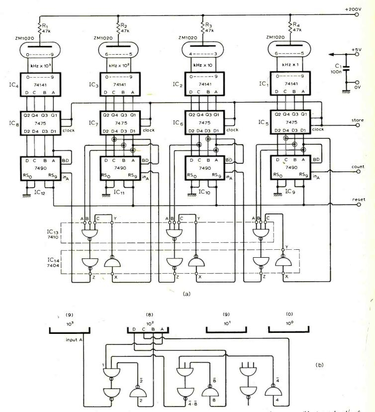
Fig. 3(a). Counter display arranged for reset to 9535. If carry circuits and counter connexions are taken to accessible pins at the edge of the circuit board, it is easy to arrange alternative i.f. offsets. A gating arrangement for an i.f. of 110kHz is shown in (b).
