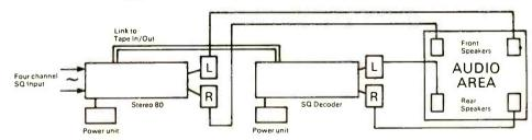
The output from any good stereo cartridge feeds into Stereo 80 and passes via the tape outlet to the 80SQ decoder. Here the signal is separated into its constituent 4 channels, those for the front being accepted by the Stereo 80, those for the rear going from the decoder to the two additional power amplifiers and speakers.
