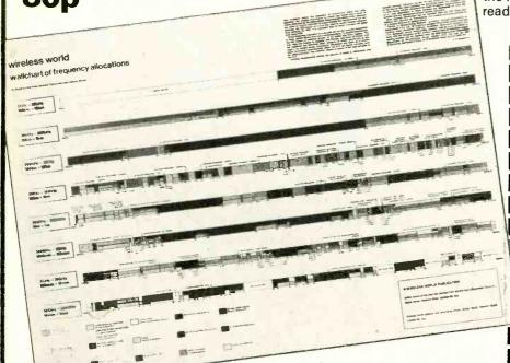
The wallchart shows the allocation of frequencies within the radio spectrum ranging from 3 kHz to 300 GHz and is scaled on eight logarithmic bands contriving 15 main categories of transmissions which are identified by colours. All the important spot frequencies and 'special interest' frequencies are marked. The information is taken from the ITU and has been condensed into easily read chart form. Measures 2'11" × 1'11".
