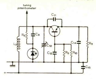
Fig. 7 Circuit diagram of a stage in an f.m. receiver.
