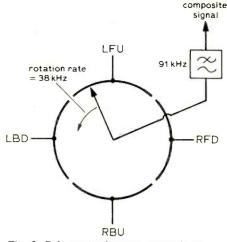
Fig. 5. Schematic showing principle of sampling four signals sequentially to produce a composite signal.
