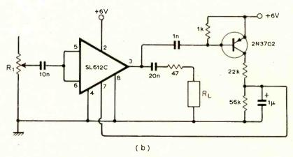
Fig. 5. Alternatives to Fig. 1 using integrated circuits.
