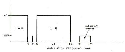
Fig. 1. Present allocation of the modulation spectrum showing the positions of the monophonic signal, difference signal and "storecast" channel.
