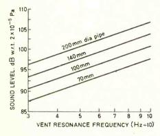
Fig. 6. Minimum pure-tone sound levels at vent resonance frequency in room of 2000ft<sup>3</sup> (60m<sup>3</sup>) for various diameter long pipes and vent resonance frequencies before distortion is appreciable.
