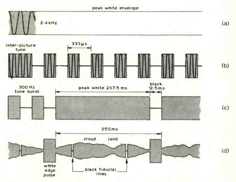
Fig. 1. ESSA-8 telemetry waveform sequence (APT), (a) peak white inter-picture tone, (b) three-second 300Hz tone burst, (c) five-second white/black phasing signal, (d) typical picture line.
