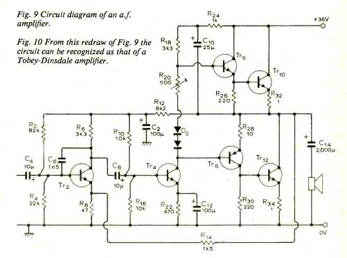
(d)  $Tr_6$  and  $Tr_8$  are a complementary pushpull pair and should be in line vertically.
