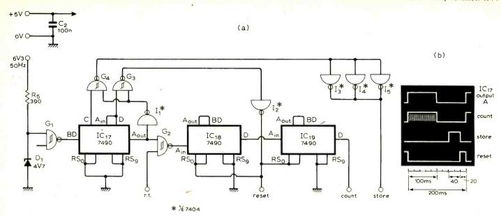
Fig. 4(a). Pulse generator circuit. The four Schmitt gates were 7414 in the prototype, but as they are rather difficult to obtain it is suggested that 7413 + 7440 be used in its place (7413 in  $G_1$  and  $G_2$  positions). A timing diagram for the unit is shown at (b).
