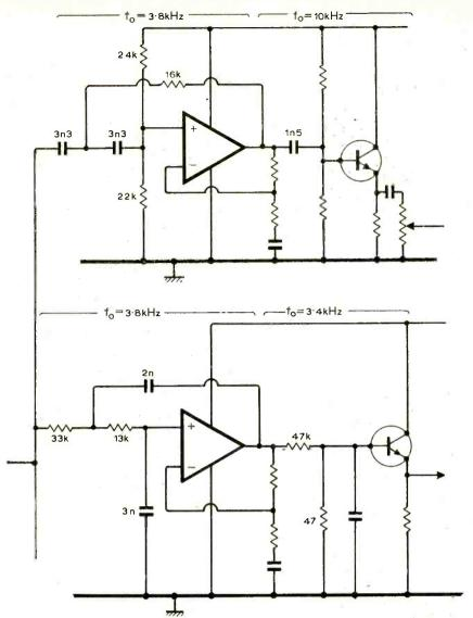
Fig. 9. Original active crossover design (December) can be improved by lowering upper crossover frequency to 4kHz. New component values shown above.
