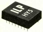
The HY5 is a complete mono hybrid preamplifier, ideally suited for both mono and stereo applications. Internally the device consists of two high quality amplifiers—the first contains frequency equalisation and gain correction, while the second caters for tone control and balance. balance
