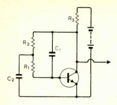
Fig. 12 A redraw of Fig. 10 with  $R_3$  in the collector circuit.
