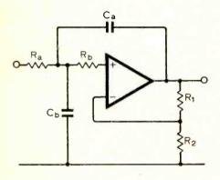
First, choose a suitable value for  $C_a$  (in  $\mu$ F) and thus find a value for a number, k, where  $k=2\pi\,C_af_a$ . In this expression,  $f_a$  is the 3dB-down frequency which can be related to a wanted crossover frequency (normally at the 6dB-down point) by inspection of the appropriate curve.
