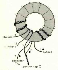
Fig. 3. Construction of the broadband output transformer for  $Tr_6$ .
