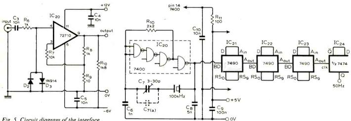
Fig. 5. Circuit diagram of the interface amplifier.
