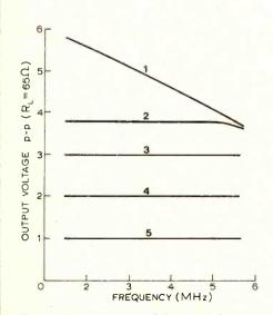
Fig. 4. Output curves of Fig. 2. Voltages are peak-to-peak across the secondary winding loaded with a  $65\Omega$  carbon resistor.
