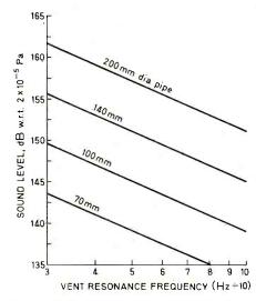
Fig. 5. Minimum pure-tone sound levels at vent resonance frequency in room of 2000st<sup>3</sup> (60m<sup>3</sup>) from vent pipes of 100mm length and various diameters for 3% second harmonic distortion.
