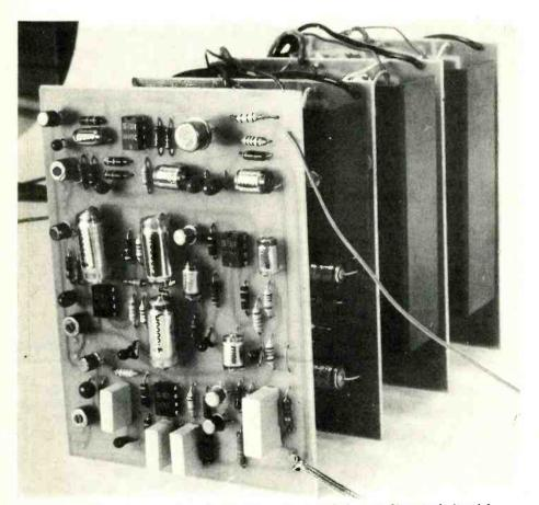
Complete amplifier for one channel. Front board is modified active filter, including l.f. section and voltage regulator, not needed for the other channel. Note reduced-size heat dissipator for h.f. power amplifier.
