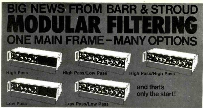
Barr & Stroud's new EF3 Electronic Filter System means no more compromises when you buy variable filters. Now you can get the filter you need today, and additional plug-in units tomorrow. Today—the basic main frame and your choice of two modules to operate in low-pass, high-pass, band-pass, band-stop, band-separate, band-combine or cascade modes. Tomorrow—other interchangeable modules to meet your newest requirements. The first two modules,
