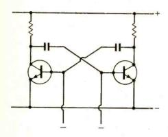
Fig. 3 A redraw of the circuit diagram of Fig. 2 in a more familiar layout.
