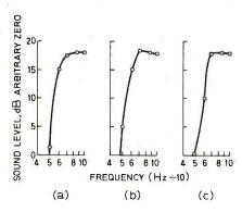
Fig. 4. Level of fundamental tone for 3% third harmonic distortion from miniature loudspeaker fitted with various vents.
