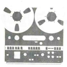
3-speeds. Full deck logic. Four inputs. Crystal servo control. Tape footage counter. Servo tape tension.
