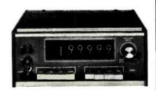
Linstead M2B electronic d.c./ a.c. voltmeter
