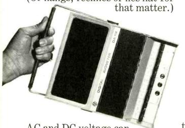
AC and DC voltage can be measured between 100mV and 1kV full range, ac and dc current between 100µA and 1A full range and resistance between  $100\Omega$  and  $1M\Omega$  full range with an overrange availability between 1000 and 1999 (except on 1kV and 1A ranges).
