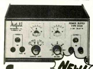
The 6130 variable d.c. power unit provides laboratories and test rooms with a new compact supply at an exceptionally low price. Among its many features are separate output and mains switching and individual voltage and current meter. Price in Great Britain. £29
