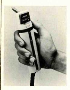
Hewlett Packard HP970A digital multimeter
