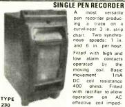
most versatile pen recorder producing a trace on a curvilinear 3 in. strip chart. Two synchronous speeds: 1 in. and 6 in. per hour.
