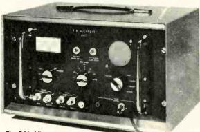
Unit Type FMU/1 illustrated was designed at the Royal Radar Establishment, Malvern, to suit Ampex Recorders working on the IRIG intermediate band specification (using ES 100 Electronics) e.g. Model Numbers FR 1200, FR 1260, FR 1300, FR 1800L, FB 400, PR 500
