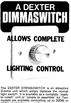
600W of all lights, except fluorescents, at mains 200-250V, 50Hz. All DEXTER DIMASWITCH models have built-in radio interference suppres-sion. 600 watt £3.52 Kit form £2.97 300 watt £2.97 Kit form £2.42
