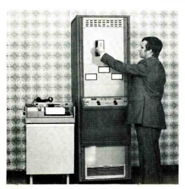
Complete prototype colour telephoto transmitter.
