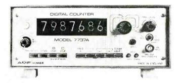
Digital counter model 7737A manufactured by AMF Venner. This is a seven-digit counter/timer suitable for frequency measurements up to 100MHz.
