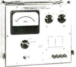
With the 747 MILLIWATT TEST Set you get laboratory accuracy in portable form. Just one instrument to standardise signal levels on 75, 140 and 600 ohm circuits.
