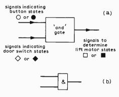
Fig. 2. The device which performs the required action is an 'and' gate (a), the logic symbol for which is shown at (b).
