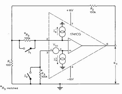
Fig. 2.1. Closed loop test circuit for measurement of input bias currents and input offset voltage.
