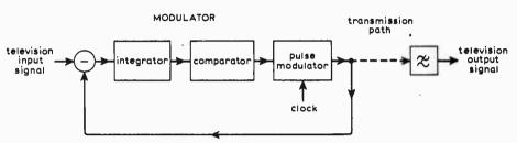
Fig. 4. Delta-sigma modulation system as applied to television signals.
