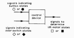
Fig. 1. Schematic of a system for controlling a lift motor from a press-button and a door sensing switch. (See text for meaning of 'state' symbols.)
