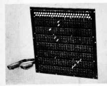
by a clock pulse every 30 minutes directed to a motorized selector switch. By means of interconnecting plugs inserted in the matrix holes at the desired cross-points, any combination of outputs is possible on the horizontal busbars. Indication of the programme status is provided by the pin situations and by indicator lamps above the vertical columns. Sealectro Ltd, Walton Road, Farlington, Portsmouth PO6 1TB. WW301 for further details
