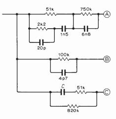
Fig. 6. Equalizing networks for Fig. 3 circuit. Values are for magnetic disc pickup A, dynamic microphone B, and tape head C. Capacitor C should be 910pF for 7½in/sec and 1.5nF for 3¾in/sec. Component tolerances should be 5% or better.
