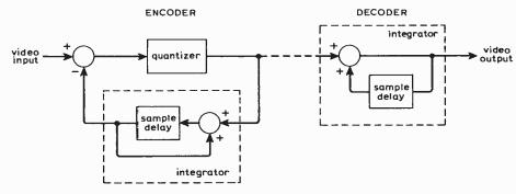
Fig. 1. Basic principle of a differential encoder-decoder as used for Post Office video telephone signals. (Binary codec for p.c.m. not shown.)
