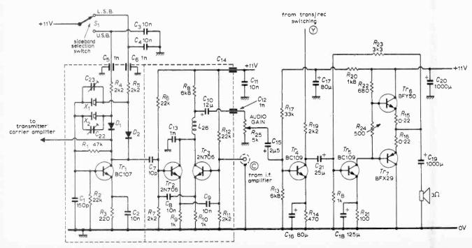
Fig. 10. Circuit of b.f.o., product detector and audio amplifier.
