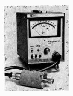
provided. Power head consists of a thermo-electric calorimeter (which converts the input r.f. power to a low-level d.c. signal) and a linear i.c. amplifier which produces a d.c. current proportional to the r.f. input. The meter measures  $165 \times 135 \times 254$ mm and weighs 3.4kg. REL Equipment and Components Ltd, Croft House, Bancroft, Hitchin, Herts. WW529 for further details
