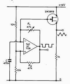
Only a moderately stable power supply is needed to obtain good frequency stability. Amplitude is directly related to the power supply voltage. Because the amplifier is used in a switching mode, reliable operation of linear integrated circuits is possible at much below the minimum power supply voltage. Consequently it is possible to achieve square-wave oscillation with a power supply of 5V making the circuit t.t.l. compatible.
