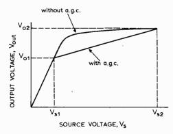
Fig. 4. Effect of a.g.c. on amplifier characteristic.
