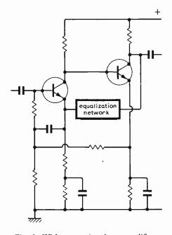
Fig. 1. With conventional pre-amplifiers of the type shown, equalization results in relatively high distortion at low frequencies — R.I.A.A. correction of 18dB boost at 30Hz means there is relatively little negative feedback at l.f.
