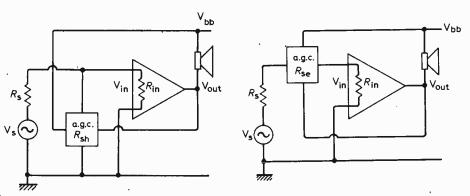
Fig. 3. Shunt a.g.c. system (a) has greater constraints on component values than series circuit (b).
