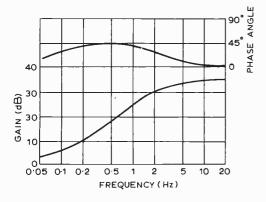
Fig. 9. Effect of l.f. roll-off capacitor  $C_f$
