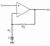
Fig. 5. Overall gain is  $(R_1 + R_2)/R_1$ . Resistor  $R_1$  is  $1k\Omega$  and  $R_2$  is in the feedback network — Fig. 6.
