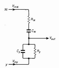
Fig. 3. Circuit of the Wien null network.
