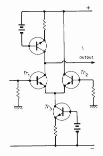
Fig. 2. Better linearity means more feedback means more open-loop gain. Use of a 'dynamic' current source as a collector load increases gain.
