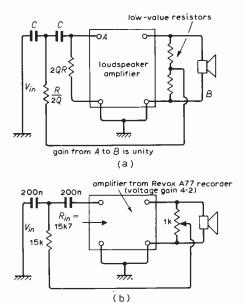
Fig. 2. Second-order high-pass active filter systems.
