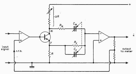
Fig. 1. Schematic arrangement of the distortion measuring system based on the Wien network.
