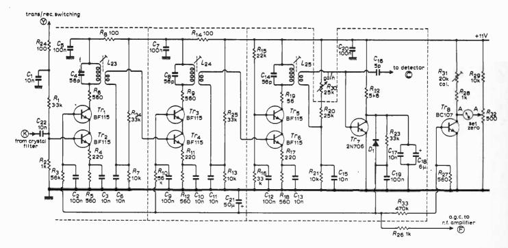
Fig. 7. The i.f. amplifier, a.g.c. amplifier and S meter. The leads to the meter (marked A) are connected to switches so that other parameters can be monitored. The circuit of the switching will be given in a later issue.
