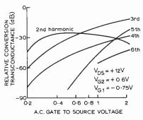
Fig. 5. Showing a.g.c. performance and the relative conversion gain of several harmonics as a function of oscillator voltage for the 3N201.
