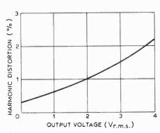
Output voltage vs harmonic distortion before feedback is applied.
