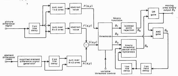
Fig. 2. Schematic of system for separating moving areas of the picture from the static background, intended for the Picturephone video telephone. Information from the present field as well as from the previous field is used.
