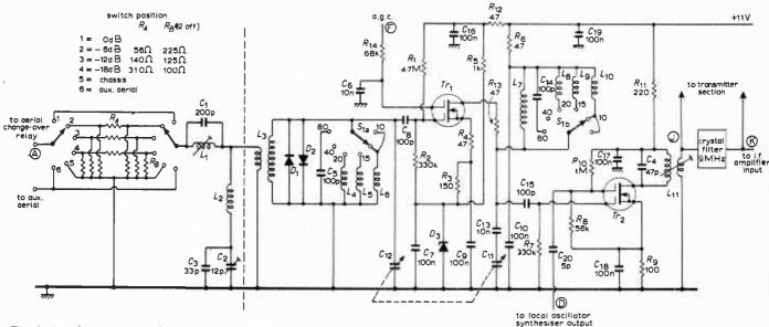
Fig. 6. Aerial attenuator, r.f. amplifier and receiver mixer.
