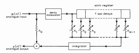
Fig. 5. Digital filter based on delta modulation in binary transversal filter technique. The resistors  $h_1, h_2, \ldots h_{M-1}$  represent different weightings applied to the tap outputs of the shift register. The input and output signals are functions of  $\mathfrak{n}$ , the number of samples, and of T the delta modulator clock period (in seconds).
