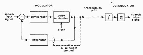
Fig. 3. Basic delta modulation system, as used for speech. An additional feedback loop for adaptive modulation, using pulse height control, is shown as a broken line loop.
