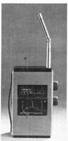
range. Octave band analysis requires one adjustment for correct readings since the input signal level and optimized signal-tonoise ratio are adjusted automatically. A telescoping microphone mast helps to eliminate the need for tripods and extension cables. Sound level measurements can be made from 10 to 150dB, A-, B- or C-weighted. Frequency is 5Hz to 100kHz and there are 10 octave bands with centrefrequencies from 31.5Hz to 16kHz. General Radio Company (U.K.) Ltd, Bourne End, Bucks. SL8 5AT.
