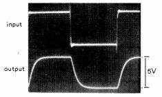
110-kHz square-wave response of circuit using network B of Fig. 6.
