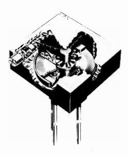
rating is 1W at  $70^{\circ}$ C (zero at  $150^{\circ}$ C) and the operating temperature range is  $-55^{\circ}$  to +  $150^{\circ}$ C. The trimmer is protected against vibration, humidity and salt spray. Dielectric strength is 900V r.m.s. at room conditions, 350V r.m.s. at 80,000ft. The wiper is shock and vibration proof, with a self-locking leadscrew and ratcheting clutch, and has a carbon tipped metal contact. Amphenol Ltd., Thanet Way, Whitstable, Kent.
