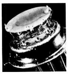
Quartz crystal and integrated circuit comprise new Marconi oscillator housed in a TO-5 package (type F3187).
