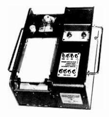
large ink well mounted coaxially with the frame. Error on d.c. is 2.5% rising to 10% at maximum frequency. One of nine chart speeds can be selected from 1.2 to 3000mm/min. Internal impedance is 210 ohms. Prices are £55 (single channel) and £90 (three channels). A ten-channel event recorder, type H30, is also available in which the ink syphons are connected to rotary relays in each channel. Current consumption is 120mA per pen. Price £52. Z & I Aero Services Ltd, 44a Westbourne Grove, London W.2.
