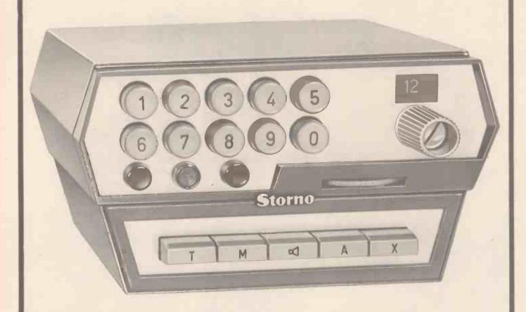
The new Storno fully automatic VHF/UHF radio communication system permits direct two-way selection dialling between mobiles and any telephone extension connected to a private automatic exchange. There are also facilities for car-to-car dialling and for predetermined selection of most frequently used extensions.
