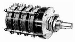
24 positions (15° indexing angle); up to 12 decks; up to 12 poles per deck; diameter over tags 1.35in; gold plated contacts. Panel and spindle seals are available. Highland Electronics Ltd, 33-41 Dallington Street, London E.C.1.
