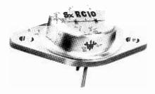
SxRC10 and SxRN10. Higher than usual overload to mean-current rating ratio is claimed. Housing is a standard TO-3 glass/metal package which permits mounting on normal transistor heat sinks. Westinghouse Brake and Signal Co. Ltd. 82 York Way, King's Cross, London N.I. WW 306 for further details
