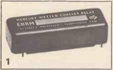
Mercury Wetted Contact Relay Type EBRM: Height only 10mm for low profile pcb mounting; 20mW bi-stable, 40mW single-side-stable; operate time Ims nominal at max. coil power; life over 25 x 109 operations at rated load of 100VA; bounce-free for both Form C or D contact resistance.
