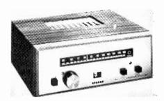
Sensitivity:  $5\mu V$  (usable). I.F. rejection: 85dB. Image rejection: 70dB. A.M. suppression: 50dB.
