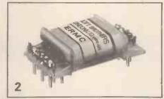
Dry Reed Relay Type ERMC/D/E: Miniature open, shielded and encapsulated styles with up to 5 poles, offering all the advantages of reeds at low cost; standard relays operate from 35mW depending on
