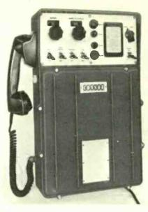
tion is given against reverse polarity. The transmitter output is 20W and the receiver audio output 3W to a built-in loudspeaker. Power supply is a nominal 24V d.c. and a range of converters is available for operation from any a.c. or d.c. ships' mains. Transceiver and extended control unit can be bulkhead mounted. Cossor Electronics Ltd, The Pinnacles, Elizabeth Way, Harlow, Essex.
