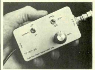
low drift high mode common small size battery powered
