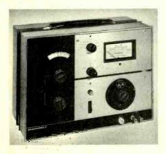
external. This can be measured in three ranges without the need for an external voltmeter. Frequency range is 86-108MHz with ±0.5% accuracy. Output is 0.1-100,000 pV and modulation 400, 1,000 and 10,000Hz (internal): Deviation is in three metered ranges of 0-30kHz, 0-100kHz and 0-300kHz, and deviation response is within ldB from d.c. to 75kHz. Wessex Electronics Ltd, Royal London Buildings, Baldwin Street, Bristol 1.
