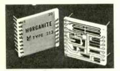
fier summation. Model 213 is a 10-bit binary resistor array designed to be compatible with the Fairchild  $\mu A$  722 current source for D/A and A/D applications. Resistance values correspond directly with those specified on the A 722 data sheet. The resistance temperature coefficient is 0 to -200 p.p.m./°C with resistance tolerance of  $\pm 2\%$  over the temperature range -20 to  $\pm 85$ °C. Morganite Resistors Ltd, Bede Industrial Estate, Jarrow, Co.
