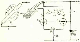
Fig. 3. Bridge containing compensating resistor R<sub>k</sub>.
