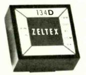
plastic /epoxy case can be mounted directly on a p.c. board or plugged into a mating connector. Specification includes an output of  $\pm V$  at 4mA, a d.c. gain of 50,000, and a gain/ bandwidth product of 1.3 MHz. Frequency at full output is 100kHz. The slew rate is 6V/s and operating temperature -25 to +85°C. Price is £8 5s. Advance Institute Electronics, Raynham Road, Bishops Stortford, Herts
