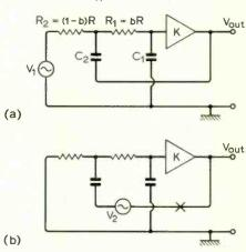
Fig. 1. (a) Sallen-and-Key low-pass filter; (b) the same with  $V_1$ short-circuited and a new source  $V_2$ introduced to facilitate analysis as a lead-lag loop with positive gain.
