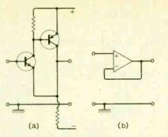
Fig. 3. Possible amplifier configurations for  $K \rightarrow I$ .
