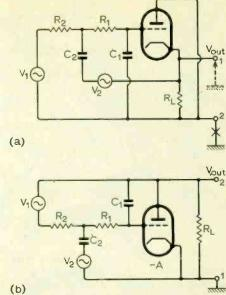
Fig. 4. By changing only the earth point, a Sallen-and-Key l.p. filter is shown to be a lag-and-integrator loop. Also, as the alternative input,  $V_2$ , has one side earthed, the circuit is now suitable for use as a 1st-order band-pass filter.
