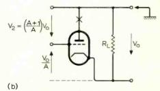
Fig. 2. Example of an active device—a value: (a) in common-cathode connection, i.e. as a high-gain amplifier,  $V_0/V_1 = -A$ ; (b) in common-anode (cathode-follower) connection, i.e. with 100% series negative feedback,  $V_0/V_2 = A/(A + 1)$ .
