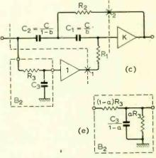
Fig. 11. Modifications for obtaining a notch (or zero): (a) Effectively passive symmetrical notch filter with buffer amplifier in h.p. path; (b) the same made active; (c) similar circuit with buffer in the l.p. path; (d) a method of putting attenuation in the h.p. path of (b); (e) in the l.p. path of (c).
