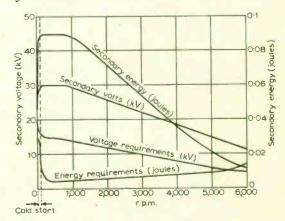
Fig. 2. Typical performance of the circuit of Fig. 1 together with engine energy requirements. The curves assume that battery voltage is normally 13.5V falling to 10V at cold start.
