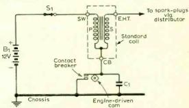
Fig. 1. Circuit of a conventional inductive discharge ignition system.
