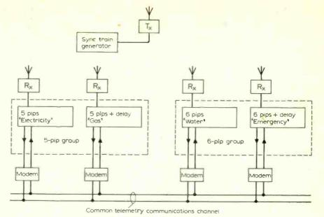
Fig. 1 "Telegrid" diagrammatic network arrangement.
