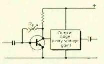
Fig. 1. Arrangement where driver stage  $Tr_1$  controls d.c. level of output pair.
