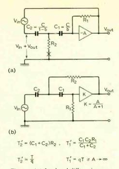
Fig. 10. (a) Lead-and-differentiator loop with series feedback; (b) the same converted by change of earth point to Sallen-and-Key h.p. filter.
