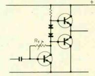
Fig. 2. Typical low-to-medium power output stage.
