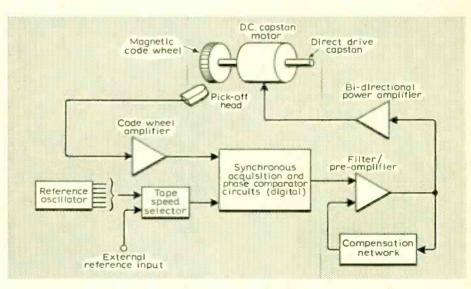
Fig. 1. Speed control system employing magnetic tachometer.
