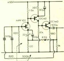
Wien bridge oscillator covering audio range with no capacitor switching. (C. A. Pye)
