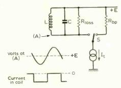
Fig. 1. Principle of a current switched LC oscillator.
