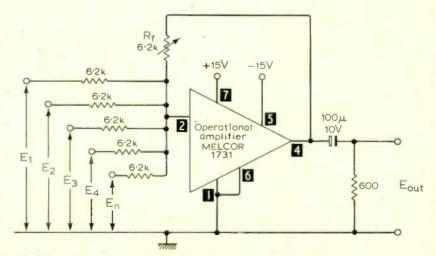
Fig. 2. Mixer using operational amplifier.
