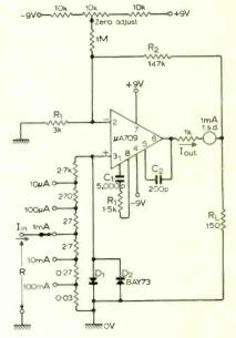
of accuracy with temperature is given as 0.2% °C. Extracted from: "The Application of Linear Microcircuits", Vol.1, SGS Ltd.
