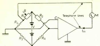
Fig. 2. Mean-square ammeter circuit.  $F_1 = type A_1$ manganese zinc ferrite (Ferroxcube toroid FX 1322) (i.d. = 6.35 mm,  $l_l = 2.76$  cm,  $l_g = 0.59$  mm,  $\mu_{min} = 100$ ).  $T_{r_1}$ ,  $T_{r_2} = type C444$  transistors (SGS Fairchild).  $R_1$ ,  $R_2 = type$ FP28D470 magnetoresistances (see Fig. 1 and Table 1).
