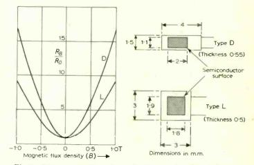
Fig. 1. Magnetoresistance relation  $R_B/R_0$  as a function of the magnetic flux density B for two commercial devices.
