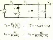
Fig. 6. CR network with resistance loading.
