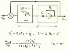
Fig. 8. Lead-and-differentiator loop as h.p. filter.
