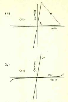
Fig. 5. Ovonic switches (a) the ovonic threshold switch: O.T.S. (b) the ovonic memory switch: O.M.S.
