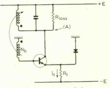
Fig. 2. Tail current is switched between the transistor and the diode.
