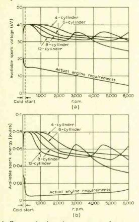
Fig. 4. Curves showing the measure performance of the capacitive discharge ignition system with the same battery voltage conditions as Fig. 2.
