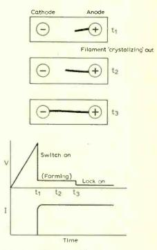
Fig. 6. Schematic of filament formation in memory device. When the voltage exceeds the threshold the current increases (switches on) but the filament takes time to form travelling from the anode. When fully formed the device resistance is lowest. This is termed locked on.
