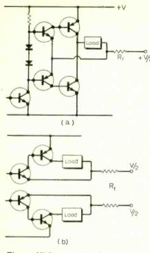
Fig. 5. High output impedance power stage. (a) Actual configuration, (b) Convenient bisection for analysis.
