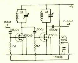
for maximum efficiency. Since  $C_{iss}$  is not highly dependent on the applied gate voltage, adjustment of VR, does not detune the preceding circuit. Doublers are not prone to feedback and interaction problems so that dual m.o.s. devices such as the Marconi-Elliott E6029 could be used. The circuit will operate up to 150MHz with the high  $g_m$  devices of the E6019, E6029 series.
