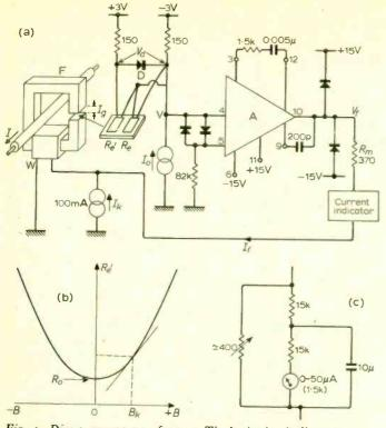
Fig. 4. Direct-current transformer. The basic circuit diagram (a) has  $R_e'$ ,  $R_e = type FP_{17}L_{100}$  magnetoresistances (see Fig. 1 and Table 1). All diodes = silicon, type ZS72 (Ferranti).  $F = manganese-zinc ferrite, grade A5 (l_g = 0.89 mm,$  $<math>l_l = 18.7 cm, \mu = 1,000$  (Ferroxcube U-cores FX1795). W = 500 turn (N) winding of 24 s.w.g.  $A = 45,000 \pm 50\%$ (MC1709CP integrated amplifier, Motorola).
