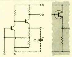
Fig. 1. The Mullard F104A/B is shown on the left which can fulfil nearly all the industrial manufacturers needs for l.f. and h.f. amplification. The shaded area contains an emitterfollower circuit which can be added so that the circuit can be made to drive long coaxial lines.
