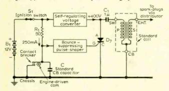
Fig. 3. Block diagram of the capacitive discharge ignition system described in the article.
