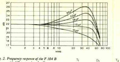
Fig. 2. Frequency response of the F 104 B with different values for C ...
