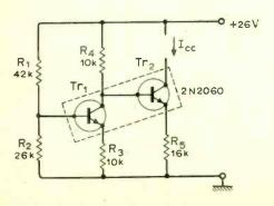
The measured temperature coefficient of  $I_{cc}$  is typically 0.0015%/°C over the temperature range 0 to 100°C.
