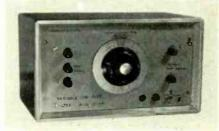
9th order Butterworth or Chebychev configuration and can realize 80dB/decade attenuation at cut off. The filters will accept an input voltage of ±10V peak and may be loaded with a minimum of 2,000 (2 Lionmount & Co. Ltd, Bellevue Road, New Southgate, London N.11. WW 318 for further details.
