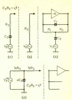
Fig. 13. Derivation of band-pass filter and an alternative form of low-pass filter from the standard l.p. filter (Fig. 4).
