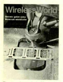
The macrophotograph on this month's cover shows wires being bonded on to integrated circuits at the Mullard Southampton works. On page 6 the future of linear i.cs is discussed.
