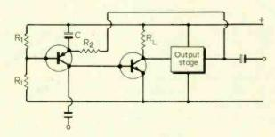
Fig. 3. Use of common-base stage to control d.c. level of amplifier output.
