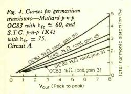
in circuit A would introduce 1-2% harmonic distortion. If 0.1% total harmonic distortion is the target figure, the largest output which could be obtained from such a circuit would be some 180mV peak to peak, equivalent to some 60mV r.m.s.
