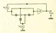
Fig. 12. Active parallel-T system with alternative input connections.
