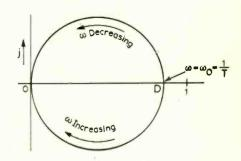
Fig. 7. Nyquist plot for positive-feedback loop containing lead-lag network.
