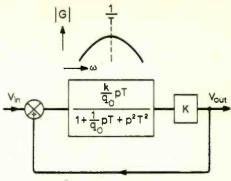
Fig. 6. Positive gain and a network with "tuned-circuit" response, given by equn. (14).
