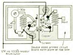
The 90MHz amplifier employs a 316-04 i.c. made by Marconi-Elliott Microelectronics. Both coils consist of five turns of 18 s.w.g. (0.3in diameter, 0.25in long), and  $L_{\perp}$  is centre-tapped.
