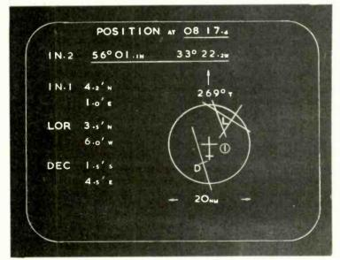
A possible solution to the problem of clearly presenting navigation information to the crew was suggested by J. G. Carr and F. S. Stringer and is shown above. The c.r.t. display shows the outputs of four navigation systems—two inertial navigators, Loran and Decca. The display graphically shows the positional information from the four equipments and shows how the outputs of three of the equipments differ from the one selected, which happens to be inertial navigator No. 2.
