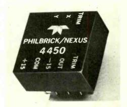
trim is required for setting up. An optional scale factor trim may be used to improve accuracy to  $\pm 0.6\%$  typical ( $\pm 1\%$  maximum) referred to 10V full-scale output. When scale-factor trim is not used, accuracy is  $\pm 1\%$  typical and  $\pm 2\%$  maximum. The price of the model 4450 in quantities of 1–9 is £41 10s each. Philbrick/Nexus Research, 81a North Street, Chichester, Sussex. WW309 for further details
