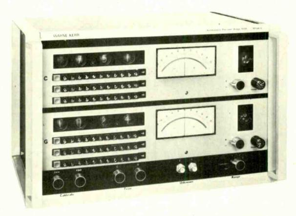
WIDE RANGE a.f. bridge for precise measurements of single components or any LCR combination - including negative resistance.
