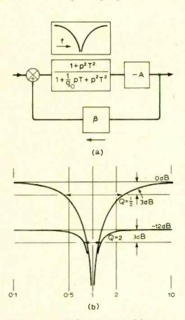
Fig. 10. (a) Feedback loop containing parallel-T network. (b) Shows increases in Q factor by application of feedback.
