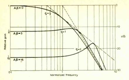
Fig. 3. Showing the effect of negative gain and feedback on a two-lag network. A is constant,  $\beta$  varies.
