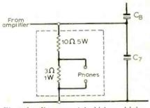
Fig. 5. Loading network for high-sensitivity earphones.
