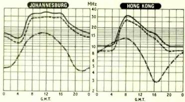
— Median standard MUF ---- Optimum traffic frequency ----- Lowest usable HF
