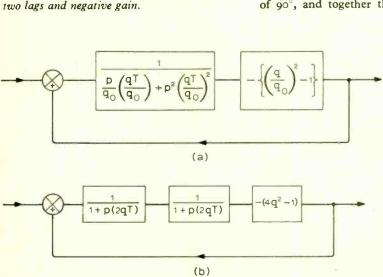
Fig. 5. Block diagrams for synthesis of feedback loops containing two lags, or their analogue (two leads, or two "tuned circuits").
