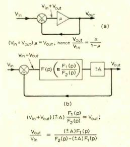
Fig. 1(a). Schematic of active feedback system; (b) the same in which μ is arbitrarily divided into a frequency-dependent factor and an aperiodic factor.
