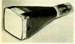
and an overall length of only 35cm. The X-sensitivity is 11V/cm and the Y-sensitivity 5V/cm. Deflection linearity is better than 5%. A typical final anode voltage for the 1400B is 12kV and under these conditions it can be used in oscilloscopes having bandwidths of 100MHz. The M-O Valve Co. Ltd, Brook Green Works, London W.6. WW323 for further details
