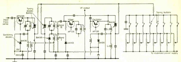
Simplified diagram of the Blaupunkt v.h.f. television tuner using varicap diodes.
