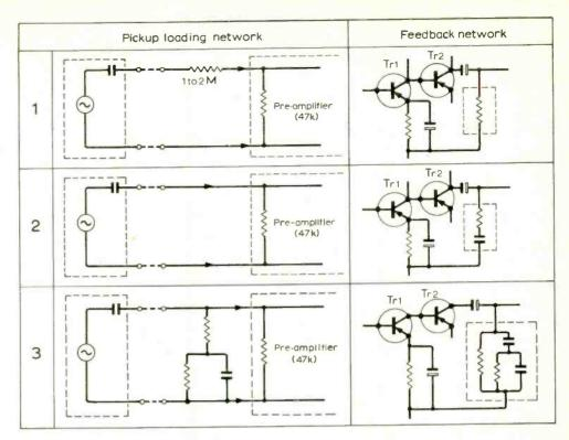
Fig. 3. Methods of loading crystal pickups. In 2 and 3 the time constants of the loading and feedback networks must be matched.
