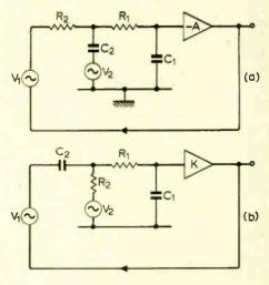
Fig. 11. Showing how a change in the position of the input can convert a low-pass filter to band-pass and vice versa.
