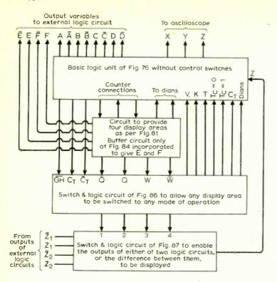
Fig. 88. A block diagram showing the interconnection of units in the type U instrument.
