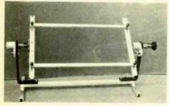
positive notch locations allowing the board to be reversed in a single operation. Extra guide rails can be fitted for simultaneous multi-assembly of smaller boards. A foam component-clamping pad is available. Keyston Engineers Ltd, 8 Tettenhall Road, Wolverhampton, Staffs.
