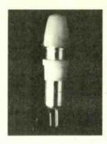
The Oxley Transistor-switched Indicator Lamp has been designed to indicate the state of logic or counting circuitry, and will find wide applications in computer read-outs and electronic instrument displays
