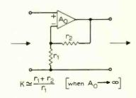
Fig. 8. Positive-gain amplifier with gain stabilized by feedback.
