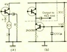
With the transistor full on, current through the load will be, instantaneously, (V/2)/R and with it cut off, the current will be I. These two currents should be equal, i.e. I = V/(2R), e.g. with a supply of 30 volts and load of 15 ohms, the standing current should be 1 amp. Efficiency should be 25% if the constant current source is ideal and the output transistor has zero saturation voltage.
