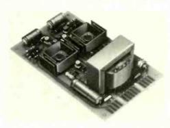
from its load. Connections can be made via a printed circuit edge connector which is supplied with the unit. Regulation drift is less than 0.05%. Ripple and noise are less than 1mV p-p. Weir Electronics Ltd, Durban Road, Bognor Regis, Sussex.
