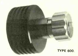
Series 600, 2, 5 and 12 watt Terminations are low reflection loads for terminating 50 ohm coaxial systems in their characteristic impedance. The frequency range is D.C. to 2.5 K mc/s with the V.S.W.R. of the termination less than 1.03 (.97) over the entire range for models fitted with E.I.D.3, Dezifix B, GR 874 or GR 900 connectors. In all 16 types of connector can be supplied.
