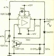
Oscillator giving constant amplitude sinewave output with unstable supply.
