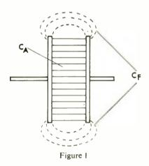
If a parallel plate capacitor is drawn, together with the associated electrostatic field, it will be apparent that the measured capacitance of this arrangement can be considered as the sum of two components;  $(^{\text{C}}_{\text{A}})$ , the value for the centre part of the field in which the lines of force are linear, and  $(^{\text{C}}_{\text{F}})$ , the value for the non-linear fringe field. Figure 1 illustrates these fields.
