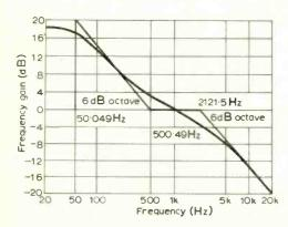
Standard R.I.A.A. curve for microgroove disc relay  $f_1 = 50.049 \, \text{Hz}$  (31 80  $\mu \text{s}$ ),  $f_2 = 500.49 \, \text{Hz}$  (318.  $\mu \text{s}$ ) and  $f_3 = 2121.5 \, \text{Hz}$  (75  $\mu \text{s}$ ).
