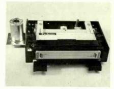
The plastic chassis loaded with a tape Packette and fitted with a drive motor.
