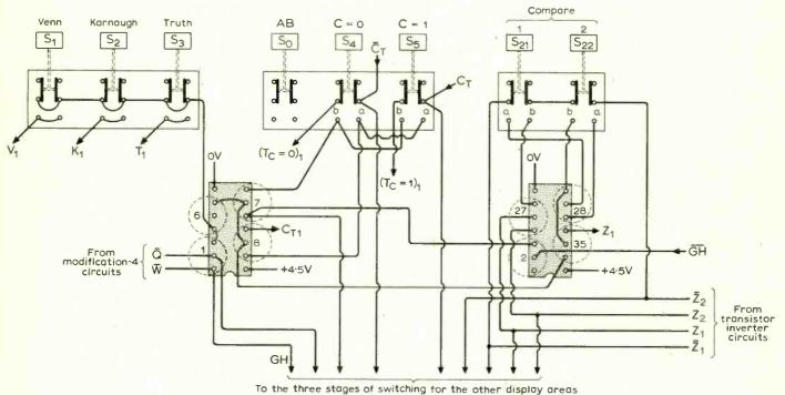
(Above) Fig. 89. Part practical layout for type U instrument. The two i.cs are ZN346Es.
