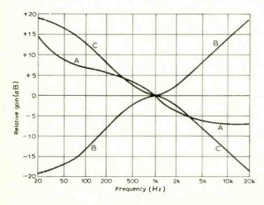
Fig. 1. Recording/ playback curves.
