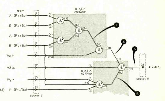
refer to the equations above. For convenience the board socket has been drawn in two halves. This circuit can now be built on board five.
