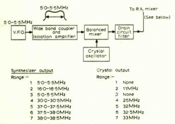
Fig. 4. The local oscillator synthesizer.
