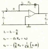
Features. The output is a composite signal made up of two components, one component proportional to the input signal added to another component proportional to the time integral of the input signal. Like the simple integrator, the circuit may be adapted to the summation of several input signals by the addition of appropriate input resistors.
