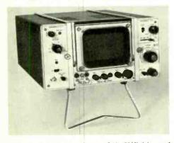
with a basic deflection factor of 50mV/division and a switched  $\times$  10 a.c.-coupled pre-amplifier. The timebase module provides calibrated sweep rates of  $0.5\mu\text{s}$  to 0.2s/division. A switched  $\times$  10 magnifier gives a maximum sweep speed of 50ns/division. Dynamco Ltd, Hanworth Lane, Chertsey, Surrey.
