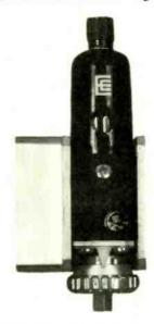
of the limiter stage gives added protection against spike leakage, which in turn reduces noise deterioration and limits crystal burn-out. For use in marine radar applications the BS908 is tunable over the frequency range 9250 to 9550MHz, and will work in duplexers with up to 75kW transmitted power. Overall dimensions are height 96.85mm, width across mounting flange 41.28mm and depth 39.5mm. Net weight is approximately 250g. English Electric Valve Co. Ltd, Chelmsford, Essex.
