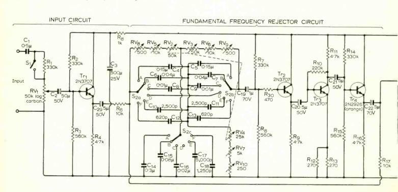
Of the six contacts in each arm of  $S_2$ , one (indicated by D) is used to disconnect the filter, so that by setting the switch  $S_3$  of the measuring amplifier at 100%, the input signal can be adjusted by  $RV_1$ , and if necessary  $S_1$ , to give a full-scale reading of 100 on the meter M, and this is the reference level.
