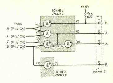
Fig. 38. Part code converter
