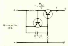
Fig. 2. Constant current source for stabilizer.
