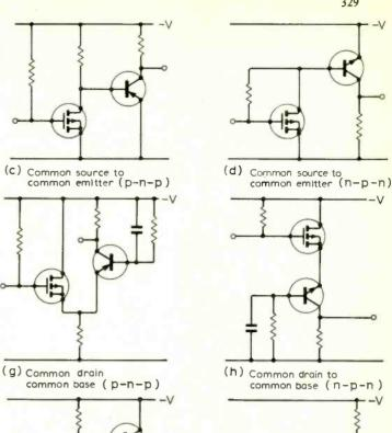
Fig. 1. Basic practical arrangements for high input impedance p-channel enhancement m.o.s.-bipolar amplifiers.
