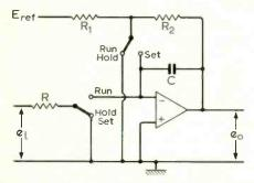
Features. With the switch in the "set" position the initial value of  $e_0$  may be set to any desired value within the capability of the amplifier;
