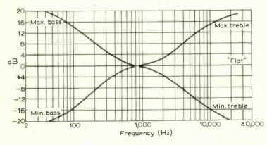
Fig. 6. Gain/frequency characteristics of the tone control stage.
