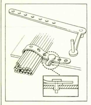
Another addition to the Insuloid range of cable fixing devices is the adjustable Rivet Clip.
