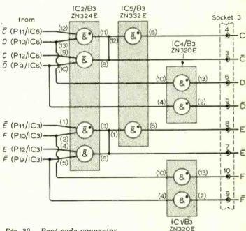
Fig. 39. Part code converter
