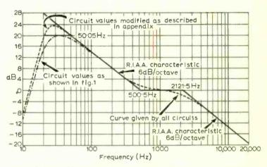
Fig. 3. Required R.I.A.A. frequency-response curve and circuit approximation to this.
