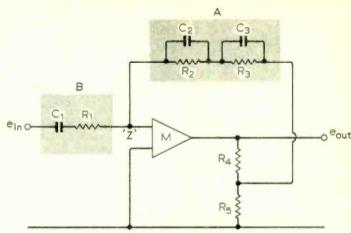
Fig. 2. Phase-inverting amplifier stage used to obtain R.I.A.A. replay characteristic.
