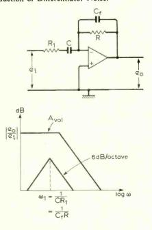
Improved rejection of high frequency noise may be obtained by the connection of a capacitor  $C_f$  in parallel with the feedback resistor R. If  $CR_1$  is made equal to  $C_fR$  the two networks have the same break frequency and combine to attenuate frequencies above  $\omega_1 = I/CR_1$ . The circuit is now in fact identical in form to the a.c. integrator considered earlier.
