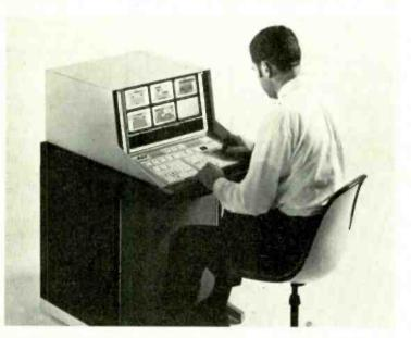
Ampex v.t.r. controller allowing randam access to material on on or more video tape recorders. Television frames are individually addressed to allow automatic searching.
