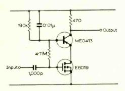
Fig. 6. Common source to common base wide-band amplifier.
