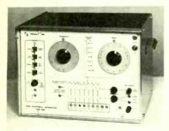
sary facilities for frequency and transient response testing, giving direct null balance readings. Using an additional generator to sweep a particular frequency range, it is possible to generate gain or loss against frequency displays on the oscilloscope. Price £334. Feedback Ltd., Park Road, Crowborough, Sussex. WW 302 for further details
