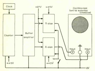
Fig. 37. Test circuit interconnection diagram
