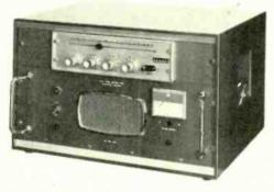
PPA120VA, complete in its own free-standing cabinet, can be used as a general purpose laboratory power supply to provide any frequency between 40Hz and 10kHz. The output voltage is continuously variable between zero and 100%.
