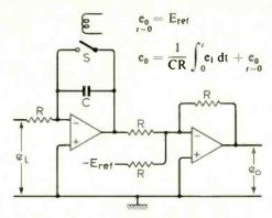
Features. With this circuit arrangement the integrator initial output is set by adding the initial conditions using a separate adder The integrator itself is set to zero with a single switch.
