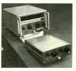
ates a polarity display and a wrong-polarity warning indicator. It also has a printer output socket at the rear. It operates from a.c. supplies from 110 to 250 volts, 47-400Hz, and has a 5MHz counter response.
