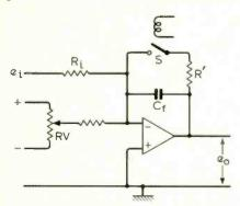
Features. With the relay reset switch open and  $e_i$  zero RV is adjusted for zero drift. With S closed the feedback capacitor is discharged and the initial output of the integrator is set to zero. A small series resistor R' is included to limit the capacitor discharge current and so protect the relay contacts and capacitor. The start of the integrating time is initiated by the opening of S.
