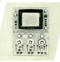
hp 1201 with dual-trace and 100 µV/cm deflection factor: £826. , hp 1207 with single-trace and 5 mV/cm deflection factor: £678. In rack and cabinet versions.
