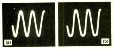
Fig.2. Oscilloscope trace of an 800-Hz wave having less than 0.1% distortion (a) and 10% distortion (b).
