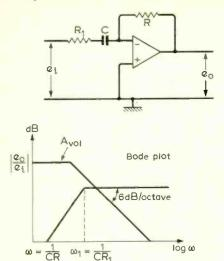
on the signal source driving the amplifier. At frequencies above  $\omega_1 = I/CR_1$  the amplifier acts as an inverter with gain  $-R/R_1$  and the rate of closure between the open loop and closed loop response becomes 6 dB/octave thus ensuring closed loop stability. The frequency  $\omega_1$  is arranged to be greater than the signal frequencies of interest.
