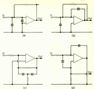
Fig. 7. Circuit arrangements for active low-pass filter design.
