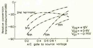
Showing the relative conversion gain of several harmonics as a function of oscillator voltage (reproduced with the permission of R.C.A.),
