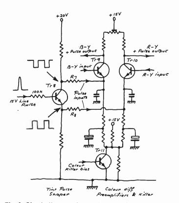
Fig. 3. Circuit diagram of part of the ITT/KB colour decoder panel showing the principle of operation of the automatic reference white correction circuit.
