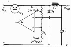
Fig. 7. Basic principle of self-oscillating switching d.c. voltage regulator using monolithic i.c.
