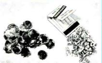
Solder chips which are usually made by dripping solder alloy on to a metal surface.
