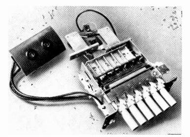
provides u.h.f./v.h.f. changeover switching. Six press-buttons provide mechanical selection of six channels in any combination of bands and systems. Each press-button incorporates a memorytype fine tuner and claims are made for high reset accuracy, ensured by designing-in a large mechanical tolerance.
