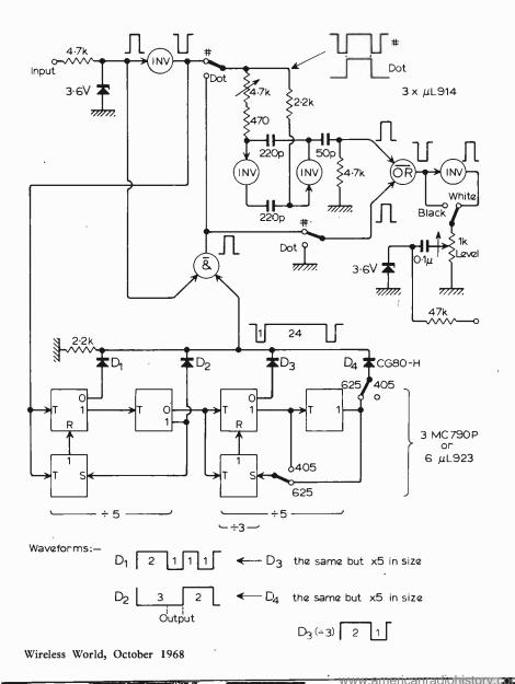
In my version a four input AND gate is required in order to achieve a one-line-wide pulse every twenty-five lines due to the odd waveforms.
