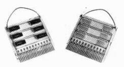
glass laminate with printed power supply tracks to each i.c. It is fitted with 24 input /output edge-connector terminations at 2.54mm (0.1in) pitch and provision is made for the attachment of a nylon cord loop to assist card removal. Size of the card is 68mm (2.7in) square and the price is 7s. 6d. Cards are also available as part of the components for a complete 6-way mounting framework. A.P.T. Electronic Industries Ltd., Chertsey Road, Byfleet, Surrey.
