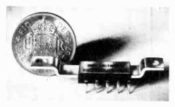
Sinclair IC-10 monolithic integrated circuit power- and pre-amplifier in dual-in-line package measuring  $2.5 \times 1 \times 0.5$ cm. Cutput of 5W r.m.s. (continuous) is claimed. Price:  $\pounds 2$  19s 6d.
