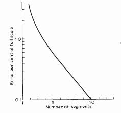
Fig. 3. A curve showing the accuracy of segmental fit.
