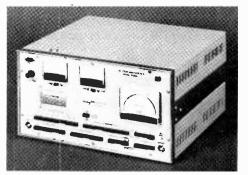
width, which is particularly advantageous when dealing with random noise. After squaring and smoothing, the result is plotted as spectral power density against frequency. Frequency accuracy is  $\pm 1\%$ over seven ranges, the lowest being 0.3 to 1.66Hz and the highest 4.69 to 26kHz Smoothing times are 1, 10, 25, 50 and 100 seconds, and integrator scaling is X1 and X10. Fenlow Electronics Ltd., Springfield Lane, Weybridge, Surrey.
