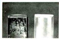
A section of a typical cast solder bar. Note the surface dross and general contamination.
