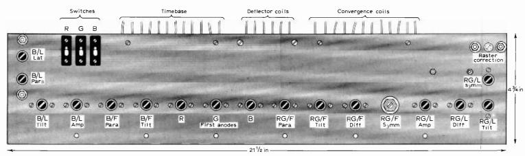
This photograph shows the underside of the convergence panel and indicates the positions of some of the chief components. The layout is far from critical.
