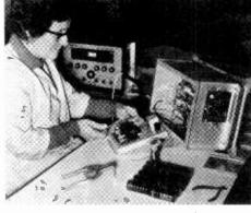
The picture shows the auxiliary power supply, a Deac rechargeable battery, being installed in a Wayne Kerr universal bridge model B221 Mk. III. The battery enables the instrument to be used in areas where no power supply is available and enables measurements to be made on in-situ components where a mains common link would be embarrassing.
