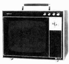
Teleton model 12-T 203U portable TV receiver with 31cm c.r.t. Power source 220/240V a.c. or 12V d.c. All v.h.f. and u.h.f. channels covered,  $300-\Omega$  balanced input. Eighteen transistors and four diodes employed. Weight 7kg. Price: about £79.
