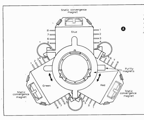
The diagram shows a rear view of the Plessey convergence assembly. For series coil connection, connect to tags 1 and 4 and join 2 and 3 for the field circuit and connect to tags 5 and 8 and join 6 and 7 for the line.
