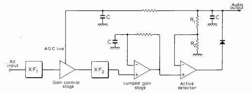
Fig. 2 Block diagram of the LM172—a complete a.g.c. stage, i.f. amplifier and a.m. detector. The capacitors and ceramic filters  $(XF_1, XF_2)$  are external to the chip.
