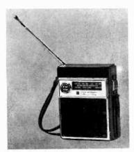
Standard model SR-K466F a.m./f.m. pocket radio receiver employing 11 transistors, and featuring a.f.c. on f.m. Output 200mW; speaker 4.5cm diameter. Power source: three mercury bateries. Dimensions:  $79 \times 62 \times$ 31mm. Price: 23gn.
