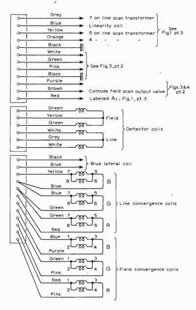
Fig. 2. External connections of the connector blocks are shown in this diagram.
