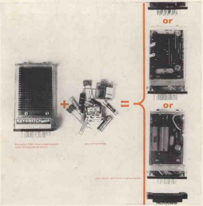
assembled units courtesy of South London Electrical Equipment Co. Ltd.
