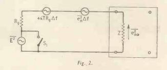
input terminals merely by dividing by the system power gain. This has been done in Fig. 2.
