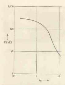
Fig. 2. Capacitance variation with reverse voltage in BAI63 tuning diode.
