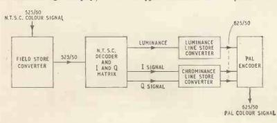
Fig. 1. Schematic of the complete conversion system The new electronic field store converter is the first unit in the chain.
