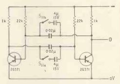
Fig. 28. Circuit of clock-pulse multivibrator. S , allows the frequency to be reduced for slow-motion demonstrations.
