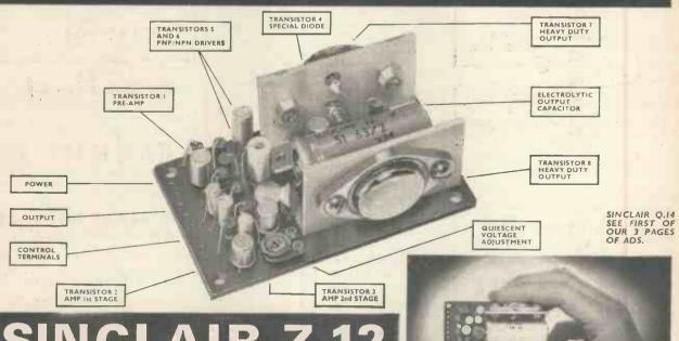
Because of its prformance and very small size, the Z.12 has completely revolutionised the whole approach to transistor amplifiers. It proves beyond all question that high-fidelity can be combined with very low price. No other amplifier in its field so successfully meets such a wide range of requirements. The Z.12 operates from any power supply between 6 and 20 v. D.C. Its output is suitable for any impedance between 1.5 and 15 ohms, making it suitable for any loudspeaker including of course,
