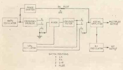
Fig. 1. Block diagram of stereo signal simulator.
