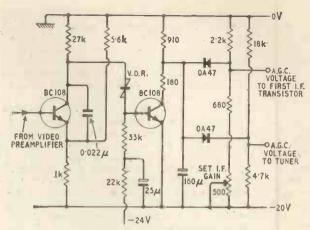
Fig. 4. A.g.c. control circuit.
