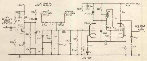
Fig. 5. Sync pulse separator (and line timebase oscillator) circuit.
