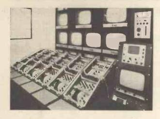
Our photograph shows the camera control position as fitted in outside broadcast vehicles supplied by Pye TVT Ltd. The equipment is from the new system 70 range recently shown at the Design Centre.
