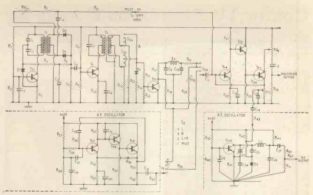
Fig. 7. Complete circuit of simulator showing a.f. and r.f. (corrier) oscillators separately
