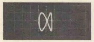
Fig. 4. Lissajus figure showing correct pilot tone phasing.
