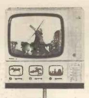
Colour receiver with three monochrome monitors which may be operated simultaneously (Nordmende).
