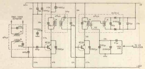
Fig. 2. 6Mc/s intercarrier sound i.f. strip.
