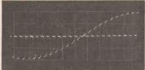
Fig. 3. Top: Waveform at Tr3 collector. Below: Expanded trace of collector waveform.
