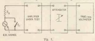
meter and the r.m.s. source voltage is noted. The attenuator is then set to 4.8 dB and the c.w. source voltage further increased to give the original reading once more. This process may be repeated for attenuator settings of 6, 7, 7.8, 8.5 dB, etc., corresponding to an output power multiplication of two, three, four, five, six and seven times the original output noise power.
