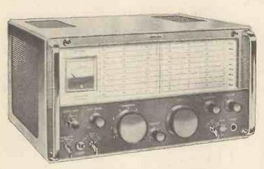
An amateur bands double-conversion superheterodyne receiver, for a.m, c.w, and s.s.b reception. For all amateur channels between 1.8 MHz and 30 MHz in nine 600 kHz bands with 28 MHz to 30 MHz in four bands.
