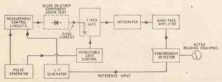
Fig. 2. Schematic of apparatus for measuring stored charges in semiconductor devices.
