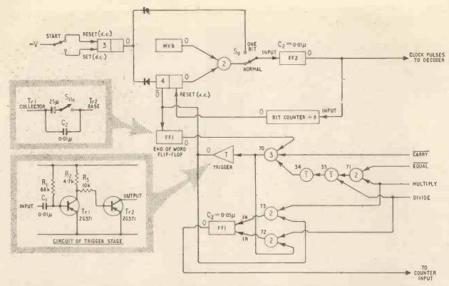
Fig. 29. The complete control unit. Note that the value of Co in e.w.t. flip-flop can be altered by S 11 for demonstration purposes.
