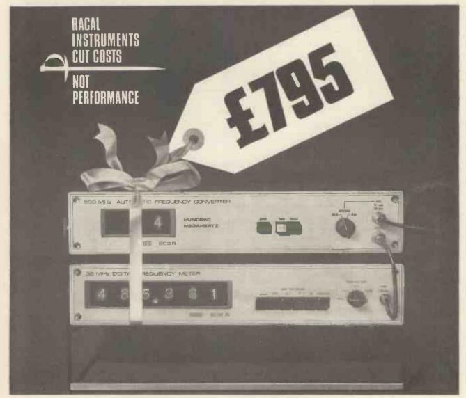
Top the 806 with the 803 and you have packaged performance. Measure to 500 MHz automatically, with the resolution and accuracy of the counter and the Racal Patent automatic heterodyne system built into the 803 convertor.
