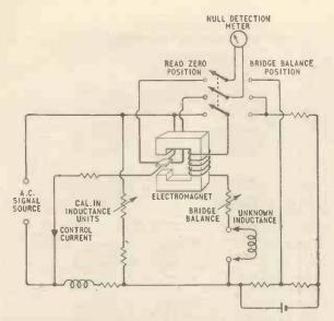
Fig. 5. Hall-effect inductance meter combined with resistance bridge.
