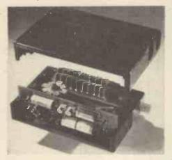
excess of 20 kc/s is fed to a Cockcroft-Walton type silicon diede multiplier stack. An external corona stabilizer is employed at the output to provide a constant voltage over a wide current range up to 200  $\mu$ A. Adjustment of output terminals across the multiplier
