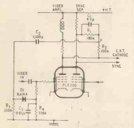
Fig. 6. Black-level correction circuit in Bush and Murphy monochrome 19-inch and 23-inch receivers.
